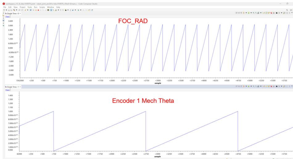
Figure 4-15. Encoder Position Feedback Data
