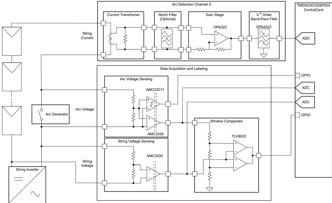
Figure 3-8. Test Setup for Test With Real Arcs
