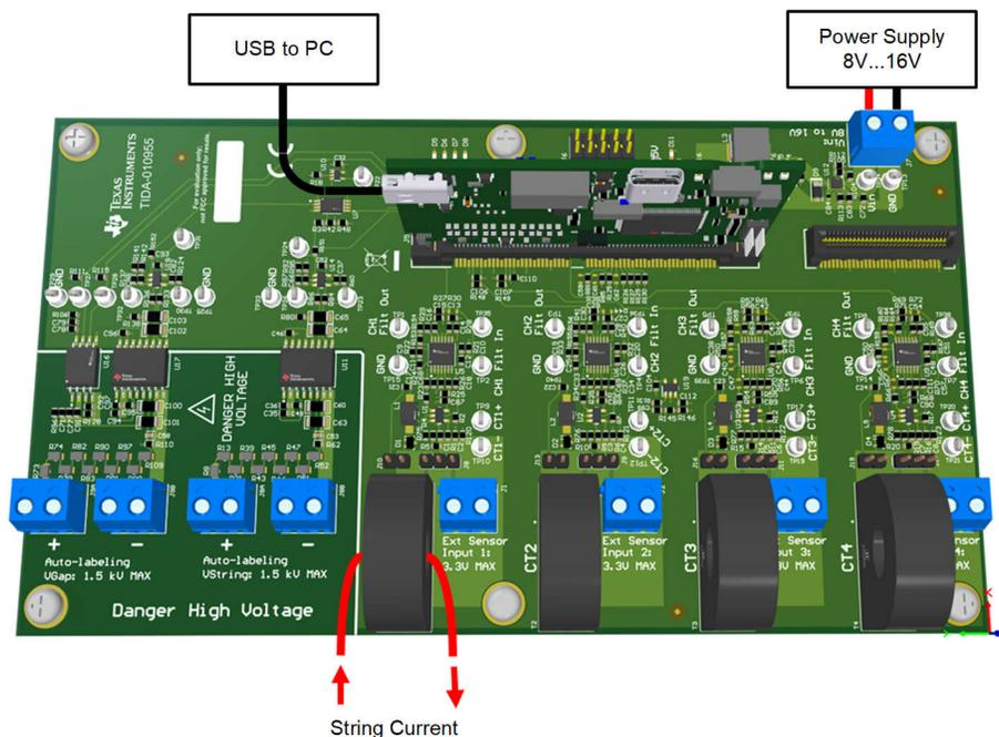
**Figure 3-1. Test Setup**
