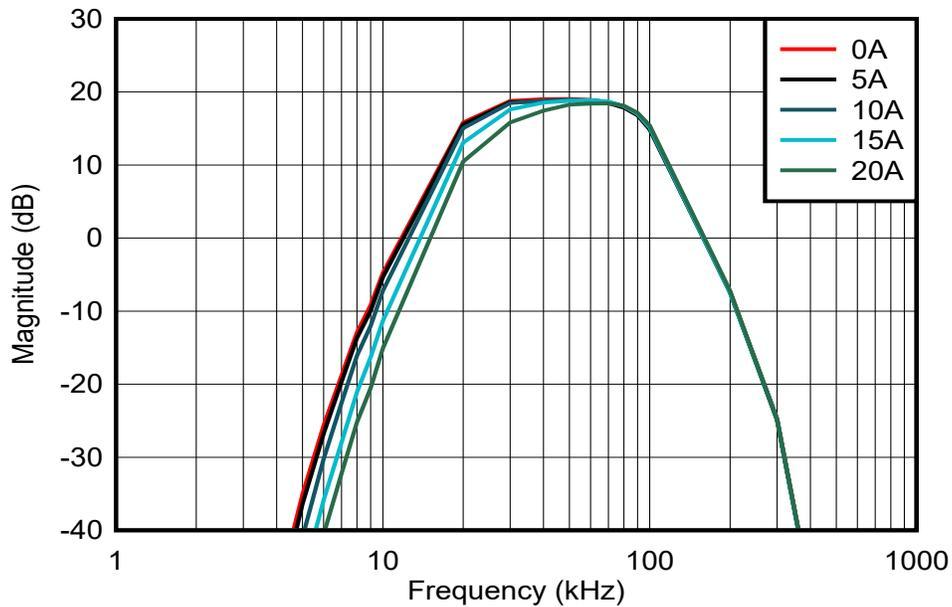
Figure 3-6. Transfer Curve of Analog Signal Chain With 8<sup>th</sup> Order Band-Pass Filter (CH1 and CH2)
