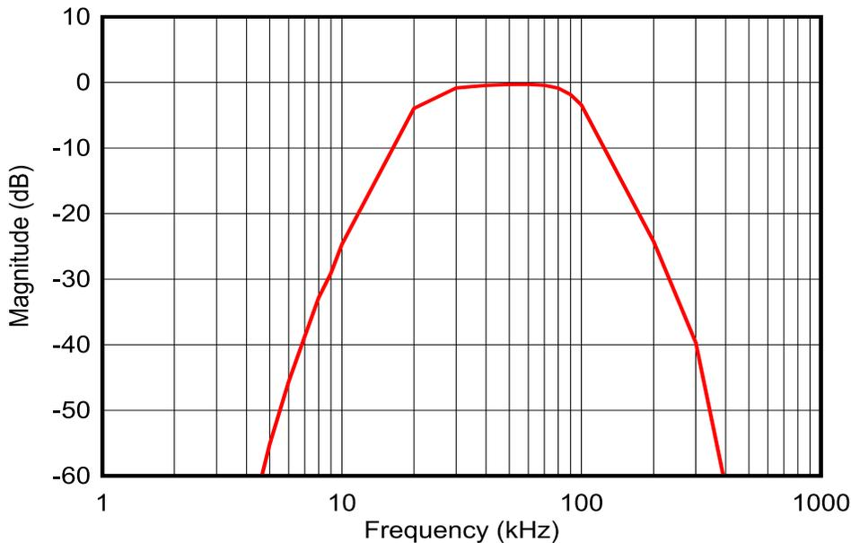
**Figure 3-4. Transfer Curve of 8<sup>th</sup> Order Band-Pass Filter Stage (CH1 and CH2)**
