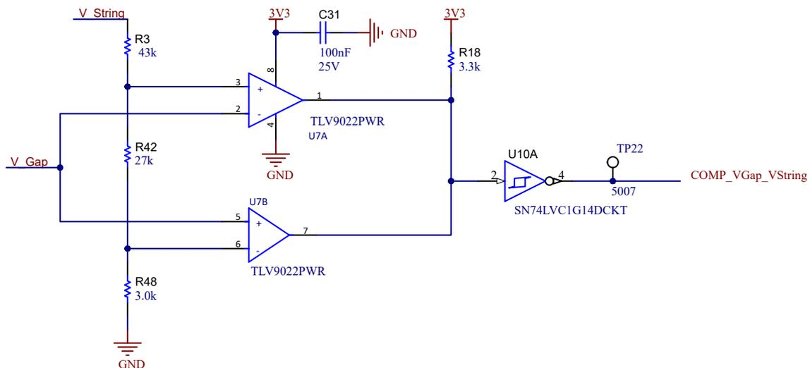
Figure 2-9. Schematics Window Comparator Circuit for Arc Labeling
