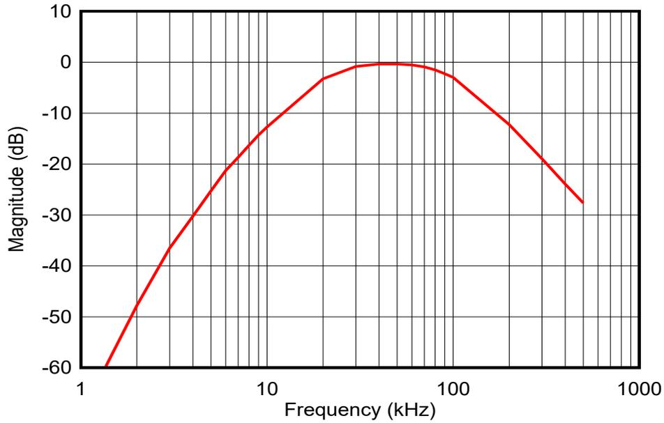
Figure 3-5. Transfer Curve of 4<sup>th</sup> Order Band-Pass Filter Stage (CH3 and CH4)
