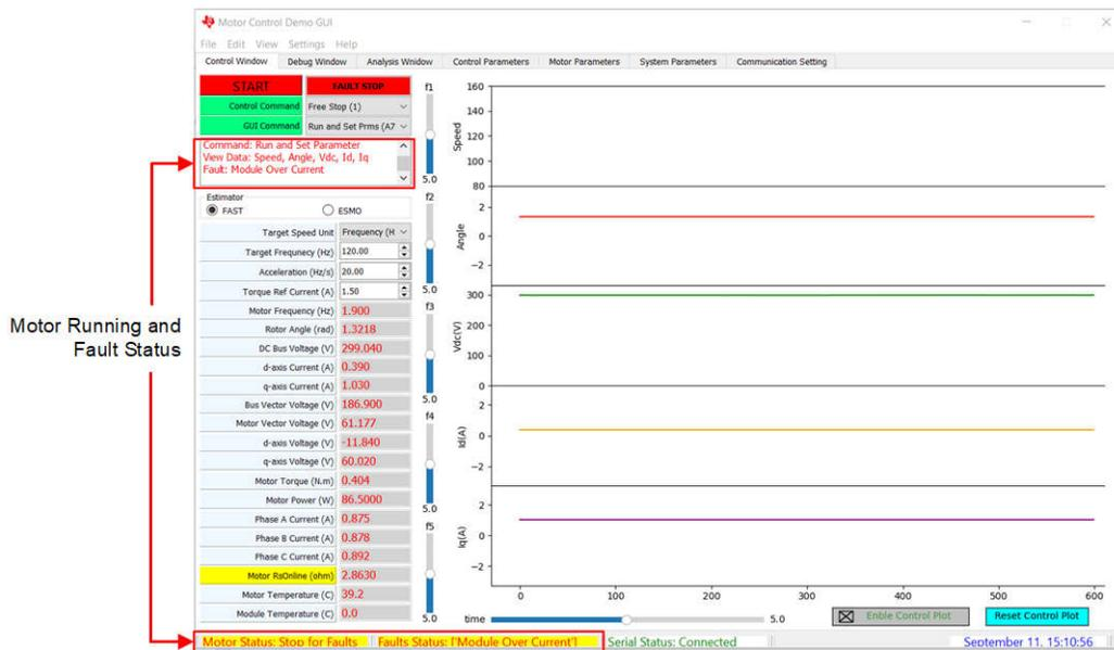
**Figure 3-12. Fault Status Monitor**
