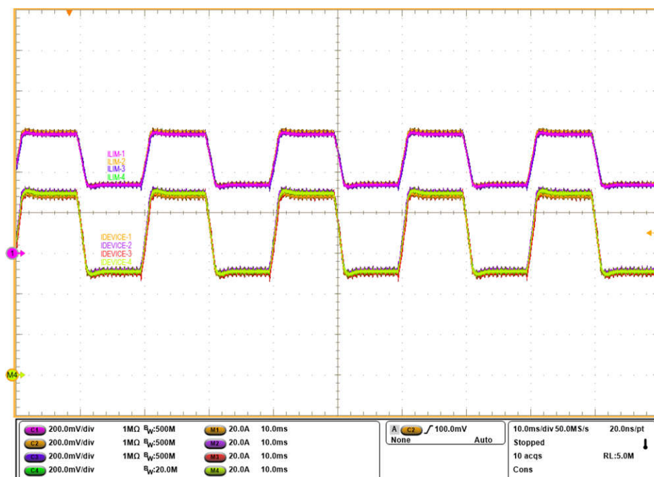
Figure 3-19. Current Sharing Among the Devices During Transient Overload Events With Four Devices in Parallel
