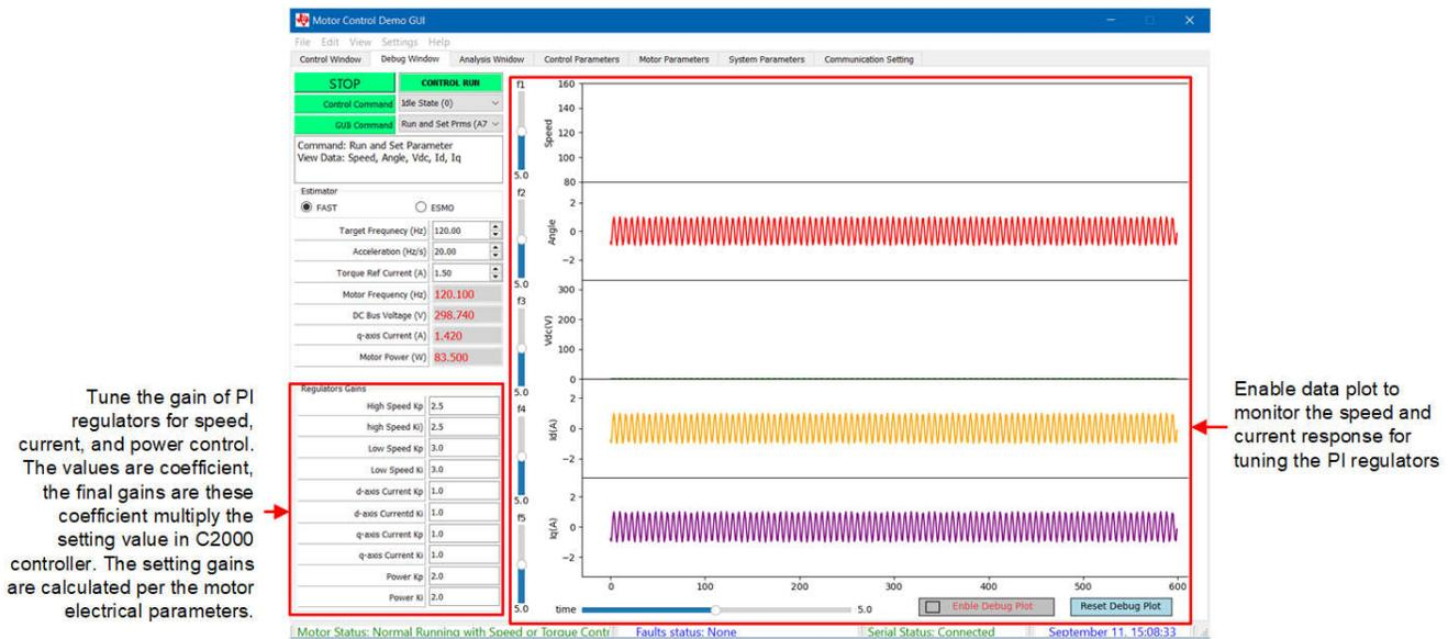
**Figure 3-14. Tune Control Parameters**
