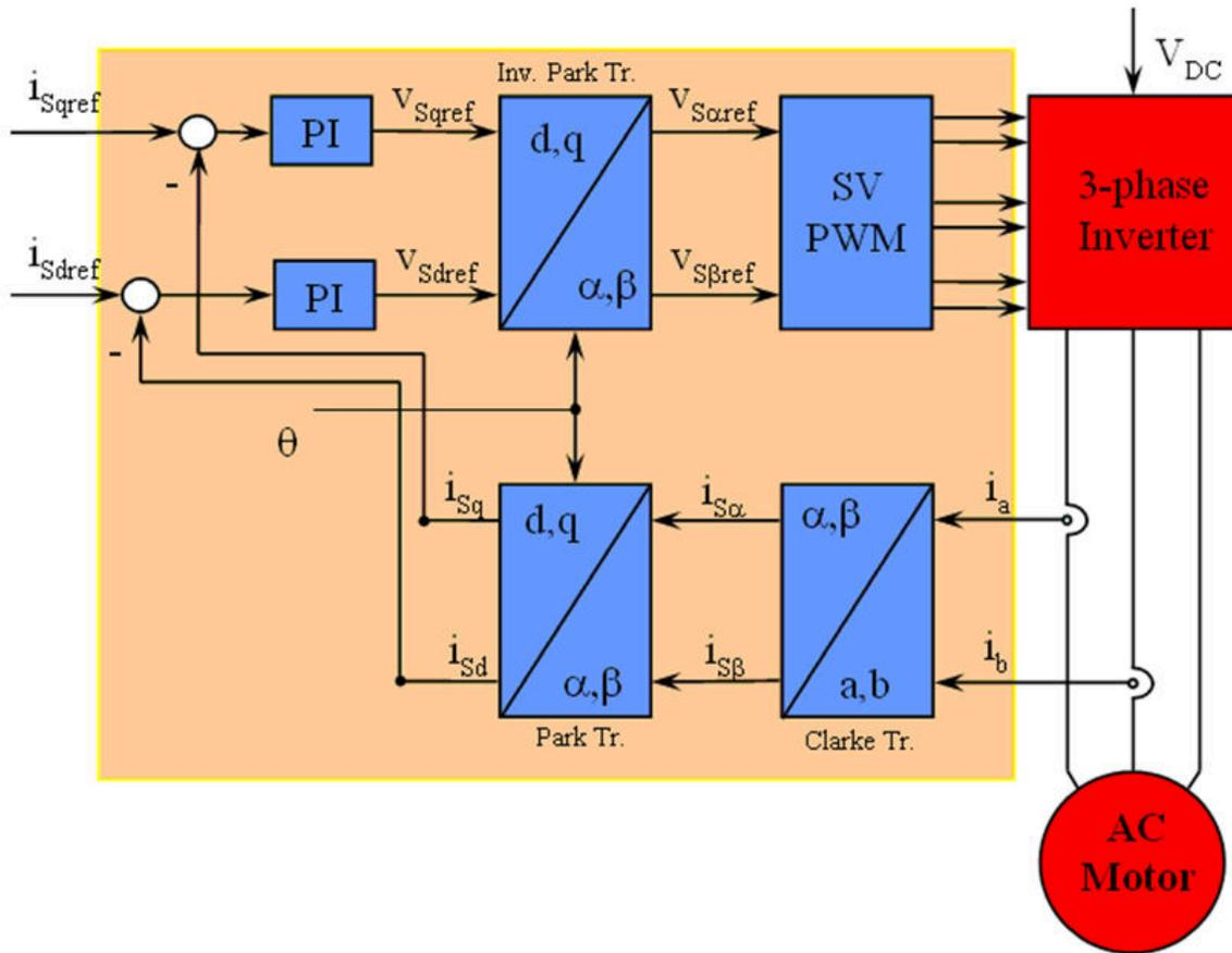
Figure 3-6. Basic Scheme of FOC for AC Motor
