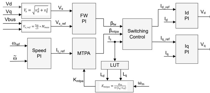
**Figure 3-10. Block Diagram of Field-Weakening and Maximum Torque per Ampere Control**
