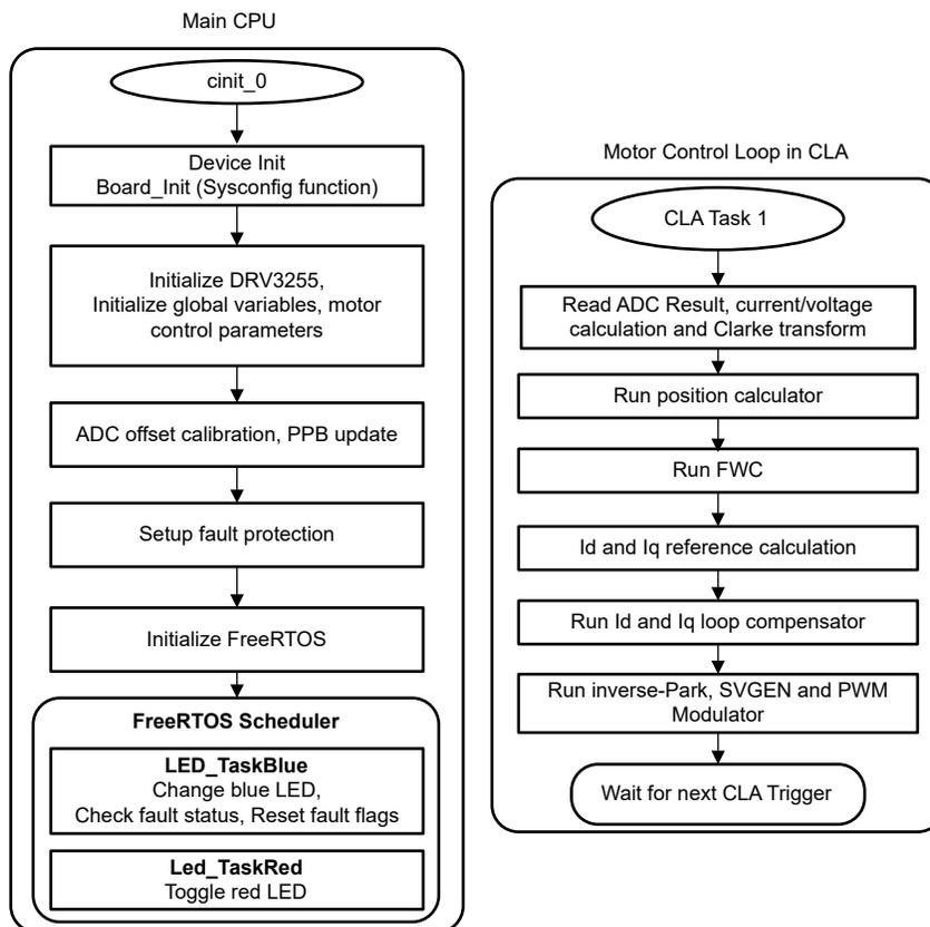
Figure 4-4. Flowcharts of Background Software and Motor Control ISR
