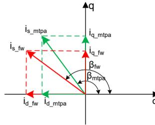
**Figure 3-11. Current Phasor Diagram of an IPMSM During FW and MTPA**
