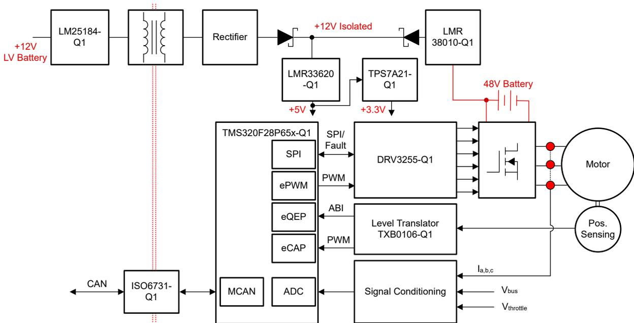
Figure 2-1. TIDM-02017 Two-Wheeler Traction Inverter Block Diagram
