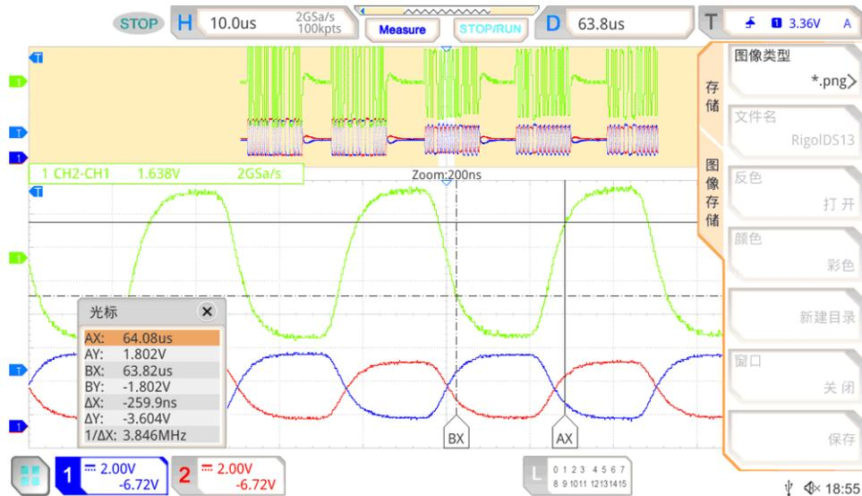
Figure 3-5. Positive Pulse-Width of Daisy Chain
