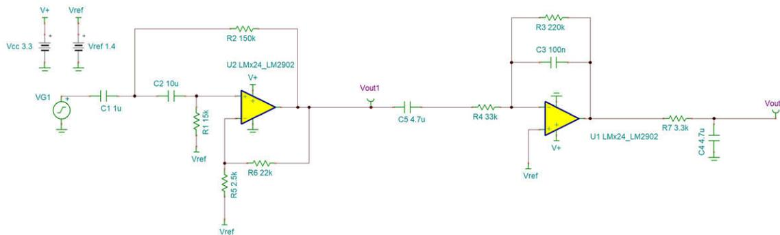
Figure 2-6. Sallen-Key High-Pass + Band Pass
