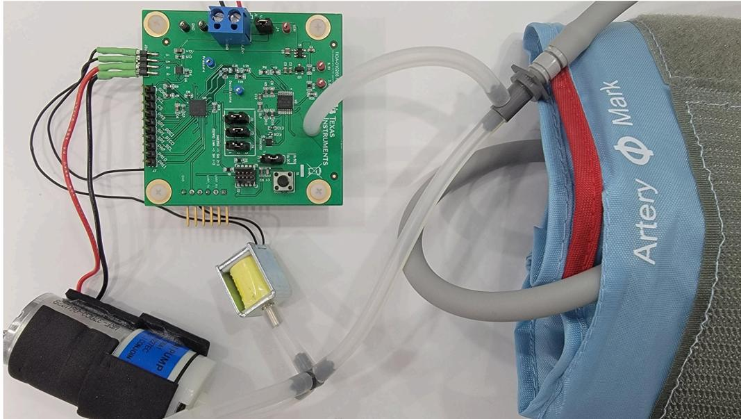
**Figure 3-1. Connection of Cuff, Pump, Valve, and Sensor for Gas Path**
