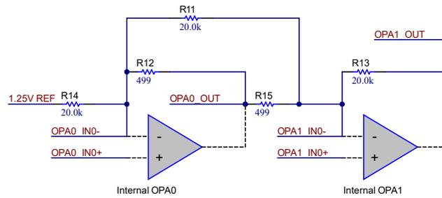
Figure 2-5. Two-Amplifier INA Circuit
