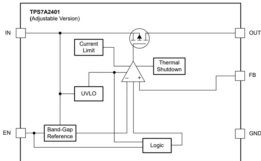
Figure 2-10. TPS7A2433 Functional Block Diagram
