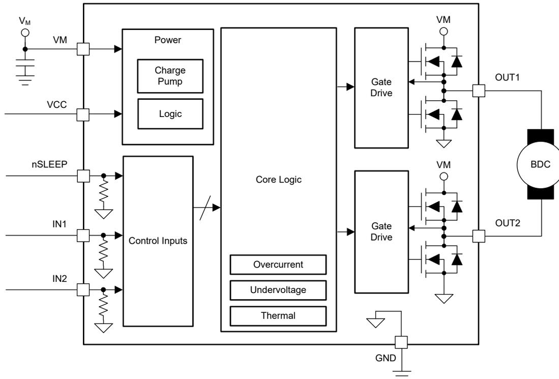
**Figure 2-12. DRV8210 Functional Block Diagram**
