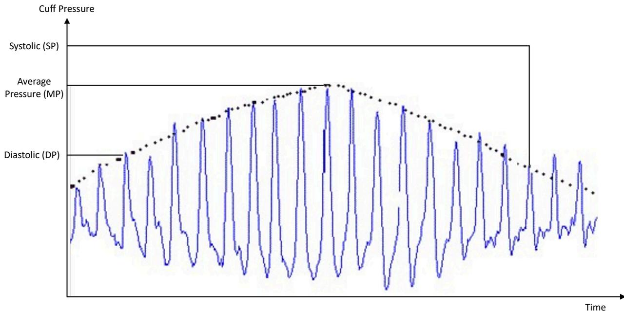
**Figure 2-3. Oscillation Method to Get Blood Pressure**
