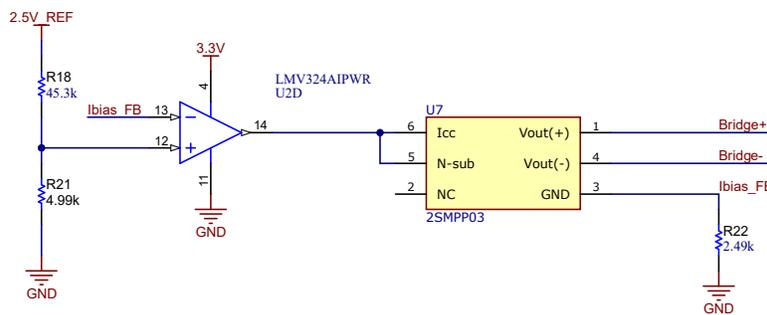
**Figure 2-4. Pressure Sensor Biasing Circuit**
