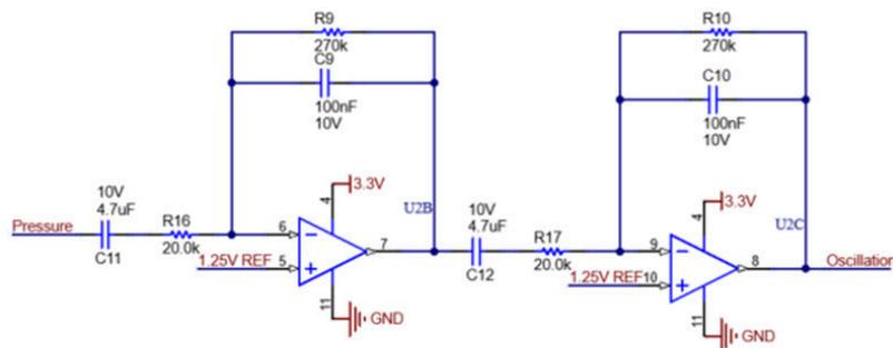
Figure 2-7. Two-Stage Band-Pass Circuit
