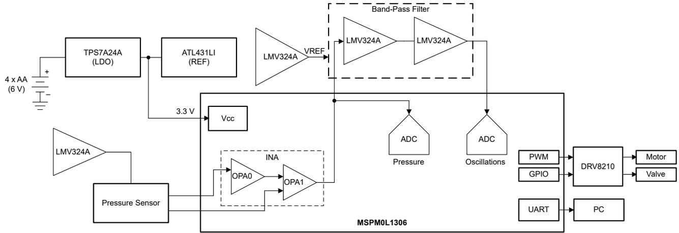
Figure 2-1. System Block Diagram A
