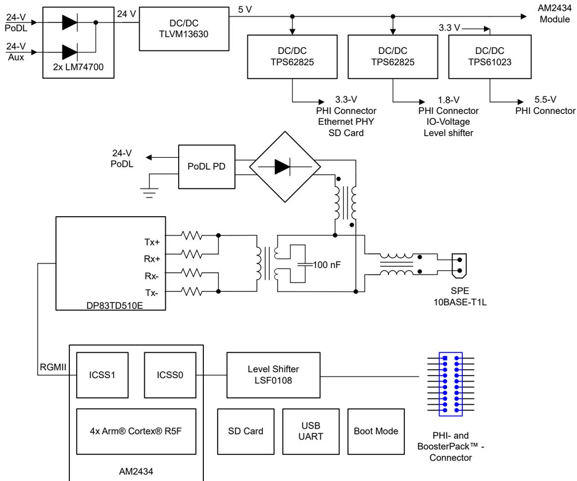
Figure 2-1. TIDA-010261 Block Diagram
