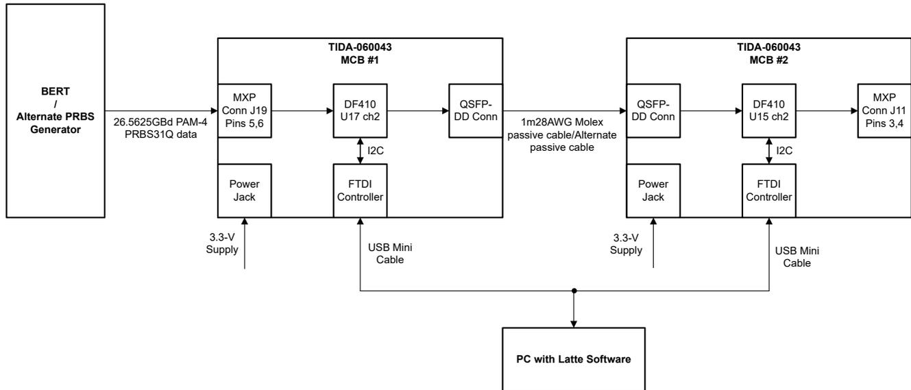
**Figure 3-2. RX Link Test Setup**
