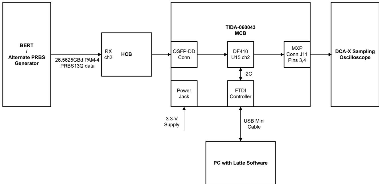
**Figure 3-1. TX Output Eye Test Setup**
