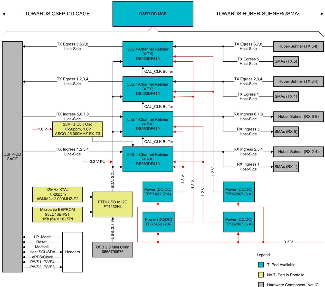
Figure 2-1. TIDA-060043 Block Diagram
