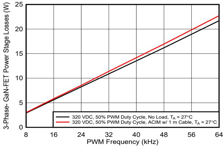
Figure 4-21. TIDA-010025 Power Losses at 320 V<sub>DC</sub> Without Heat Sink versus PWM Frequency at No Load
