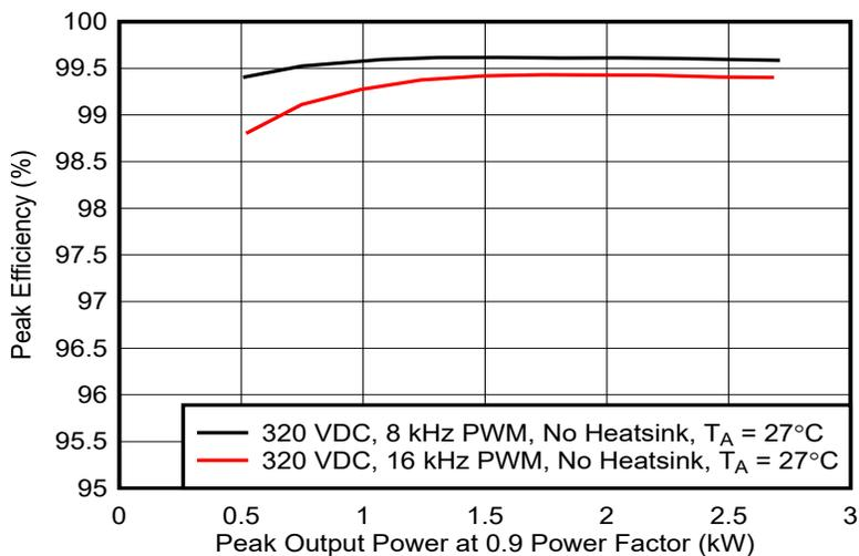
**Figure 4-20. Calculated Maximum Peak Efficiency at 320 V<sub>DC</sub>, 8-kHz and 16-kHz PWM**
