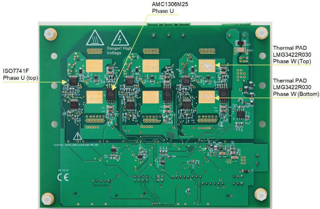
**Figure 4-2. TIDA-010255 PCB Bottom View**
