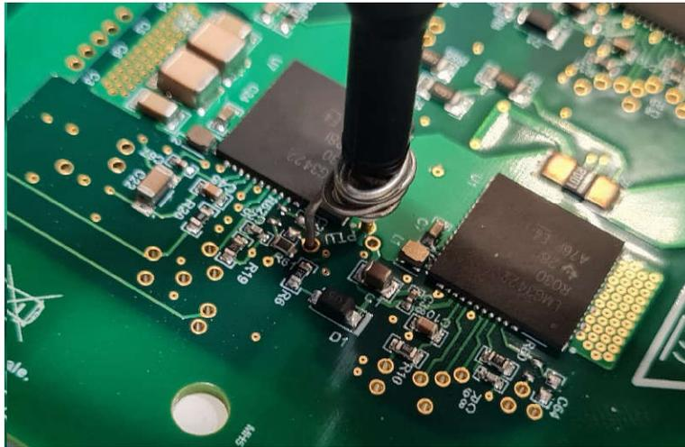
Figure 4-6. LMG3422 Switch Node Phase Voltage Measurement
