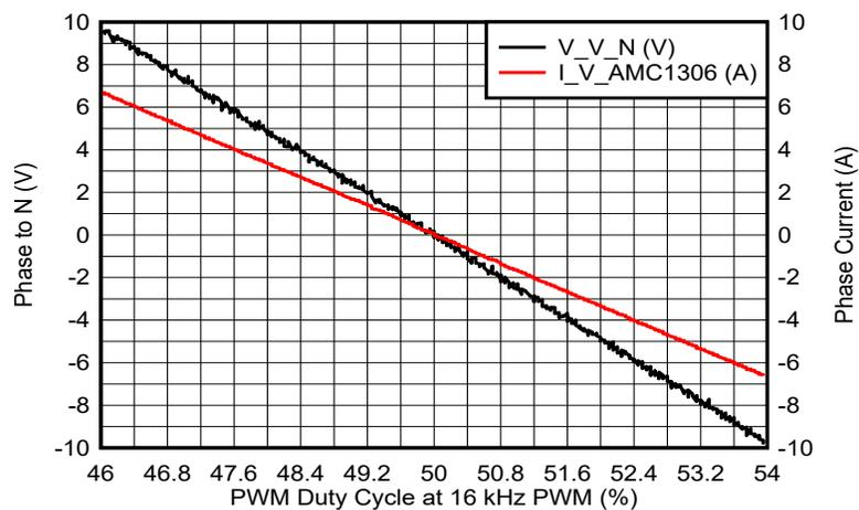
Figure 4-18. Linearity Plot of Phase Voltage and Current Versus of PWM Duty Cycle at 16-kHz PWM and 320-V<sub>DC</sub> Bus Voltage
