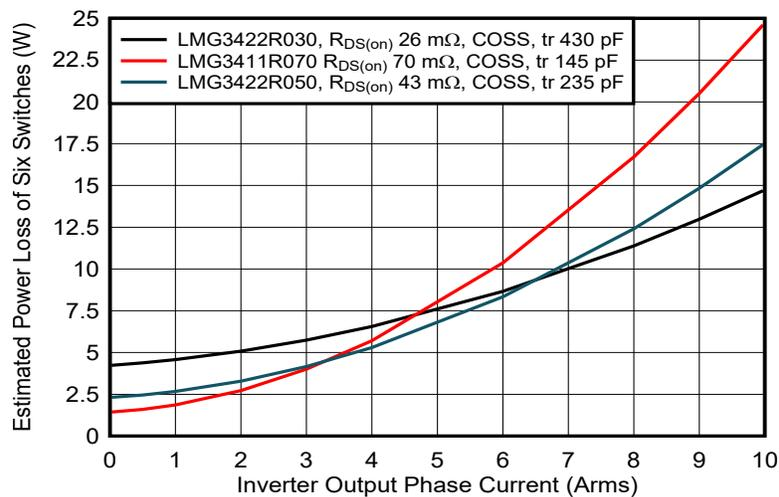
Figure 3-1. Estimated Power Switch Losses of a 320 V<sub>DC</sub>-fed 3-Phase Inverter at 16-kHz PWM
