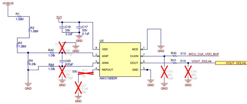
Figure 3-8. DC-link Voltage Sensing With Non-isolated Modulator Schematic
