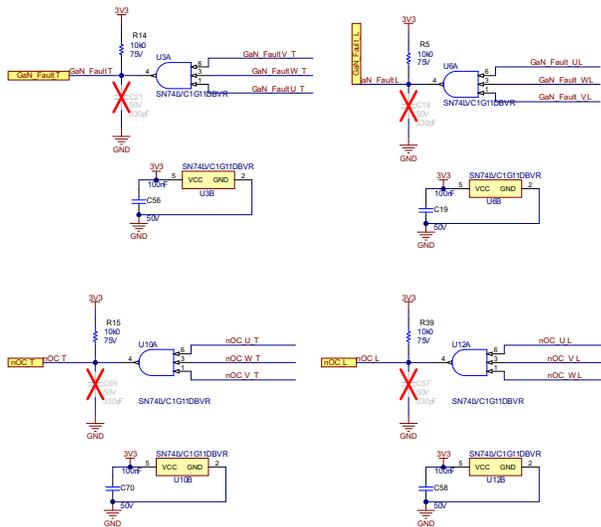
Figure 3-5. GaN-FET Fault and Overcurrent Reporting Schematic
