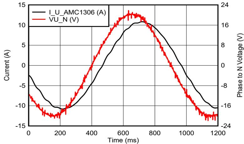
Figure 4-17. Filtered Phase U Voltage and Current With AC Induction Motor at 16-kHz PWM and 320-V<sub>DC</sub> Bus Voltage
