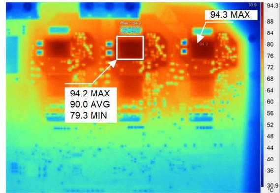
Figure 4-23. TIDA-010255 PCB Thermal Image at 7.7-A<sub>RMS</sub> Load Current
