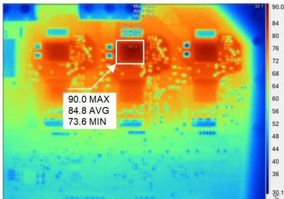
Figure 4-22. TIDA-010255 PCB Thermal Image at 7.1-A<sub>RMS</sub> Load Current
