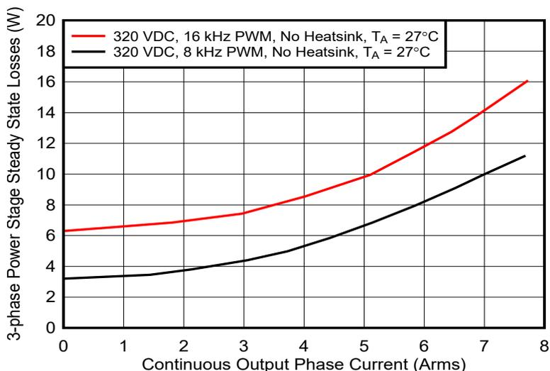
**Figure 4-19. TIDA-010025 Power Losses at 320 V<sub>DC</sub>, 8-kHz and 16-kHz PWM versus Output Current**
