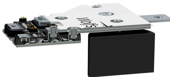
Figure 3-10. Cross-Sectional View of Laminated Bus-Bar Structure Showing Power Loop
