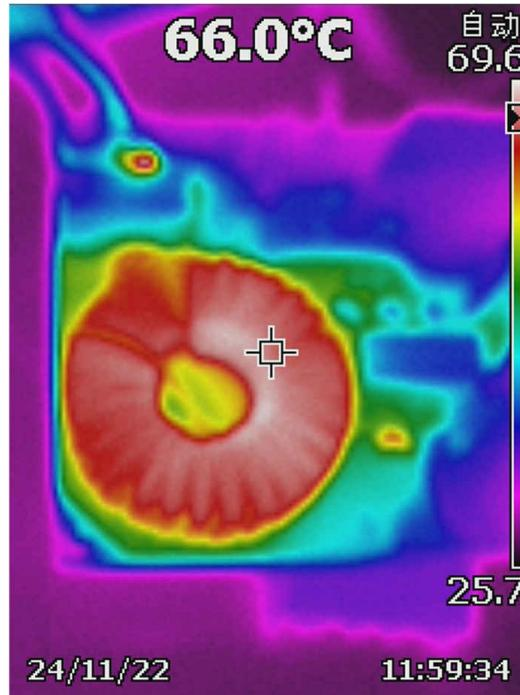
Figure 3-18. Boost Inductor Temperature
