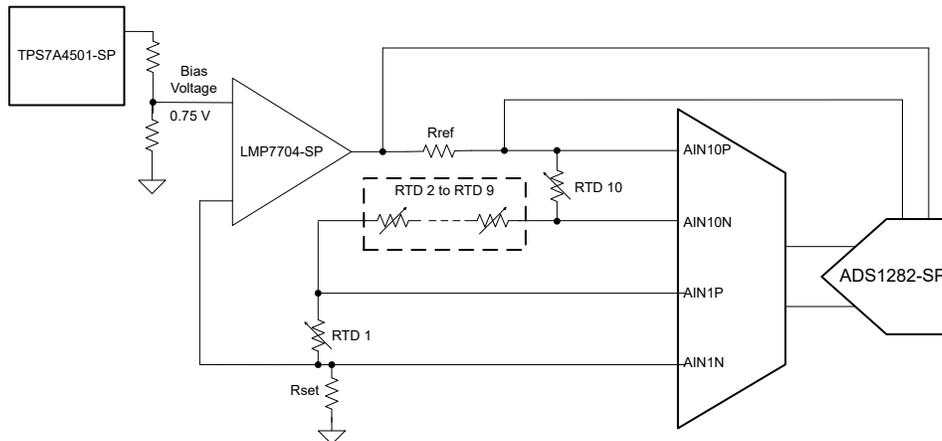
Figure 2-1. Temperature Sensing Application Block Diagram
