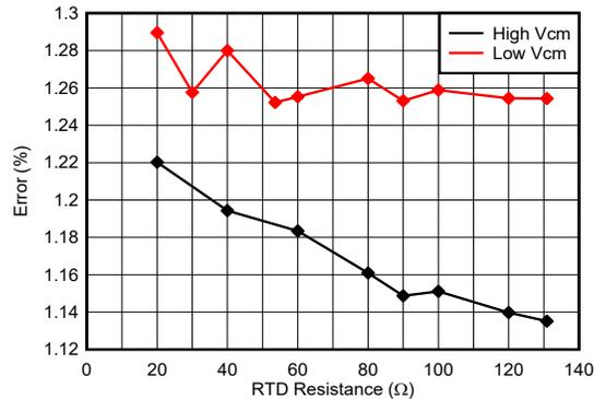
Figure 3-6. Temperature Measurement Accuracy with  $I_{RTD} = 1$  mA
