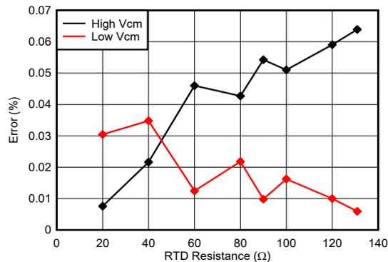
Figure 3-7. Temperature Measurement Accuracy with  $I_{RTD} = 1.5$  mA
