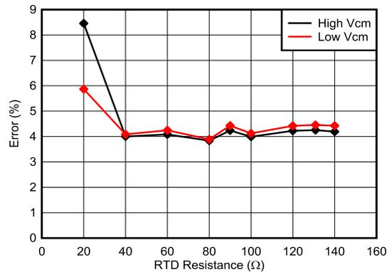
Figure 3-5. Temperature Measurement Accuracy with  $I_{RTD} = 0.5$  mA
