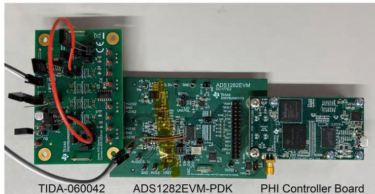
**Figure 3-2. Hardware Setup**
