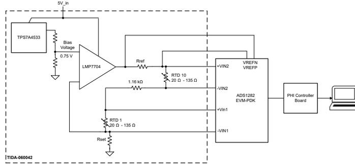
Figure 3-3. Lab Setup to Simulate Temperature Measurement
