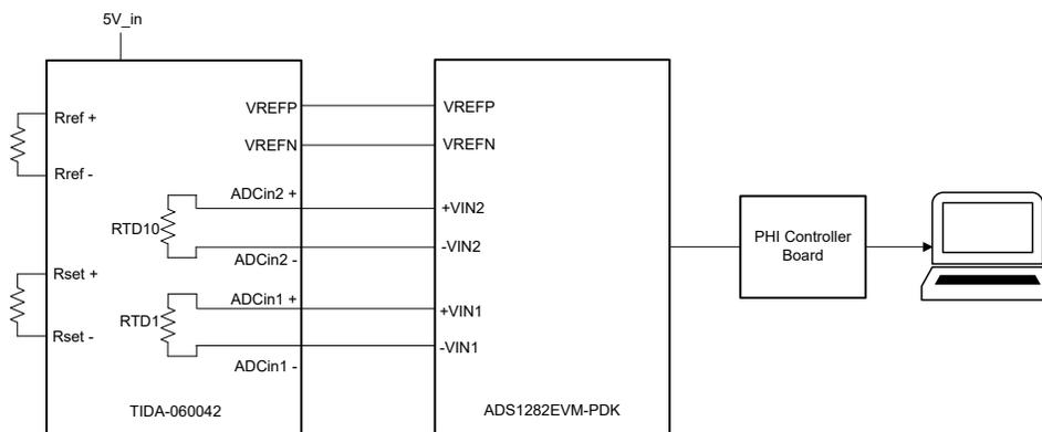
Figure 2-2. Connection Between TIDA-060042 and ADS1282EVM-PDK
