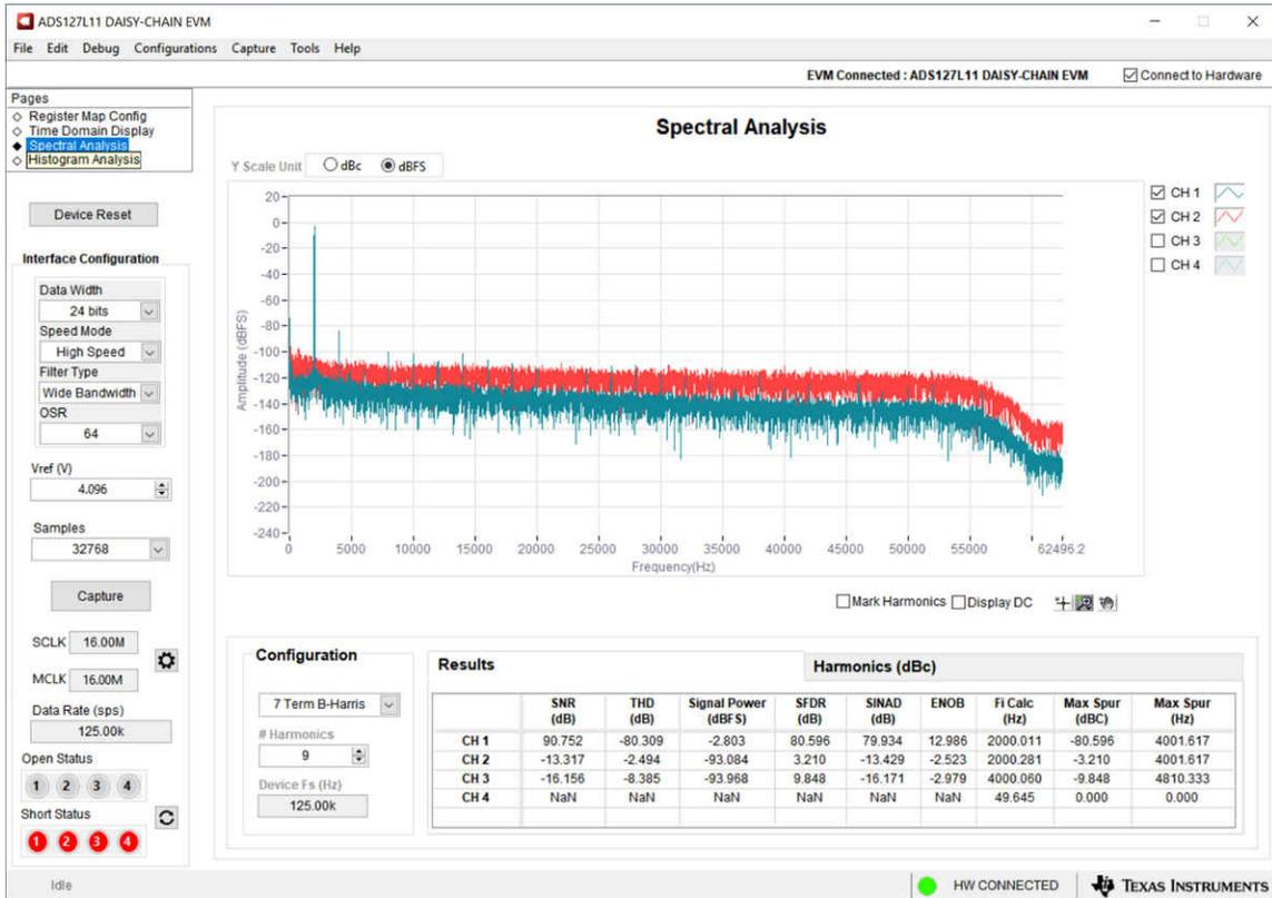
**Figure 4-14. Frequency-Domain Plot of 20-V<sub>PP</sub> Input at Channel 1**
