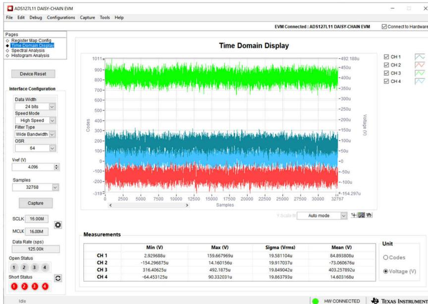
**Figure 4-12. Time-Domain Plot of Front-End Inputs Shorted**
