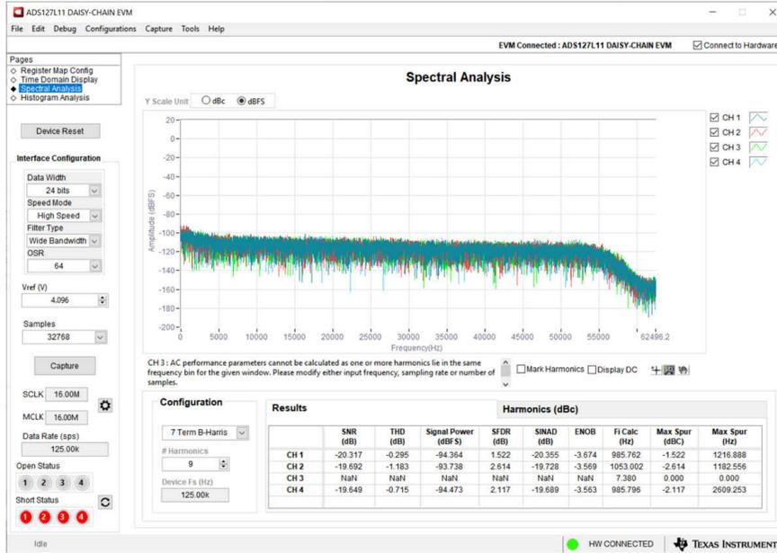
**Figure 4-11. Frequency-Domain Plot of Front-End Inputs Shorted**
