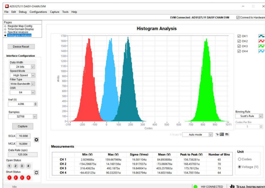
Figure 4-10. Histogram Plot of Front-End Inputs Shorted
