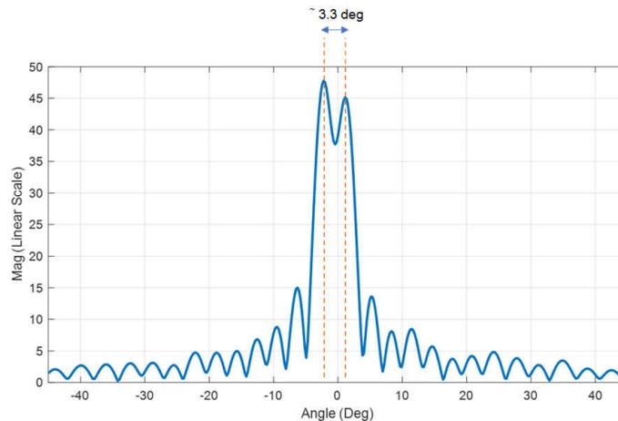
**Figure 4-4. Angular Resolution Measurement**
