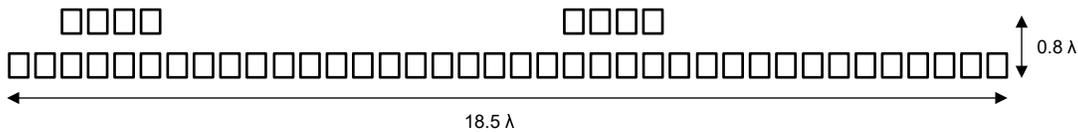
**Figure 4-2. MIMO Virtual Array**
