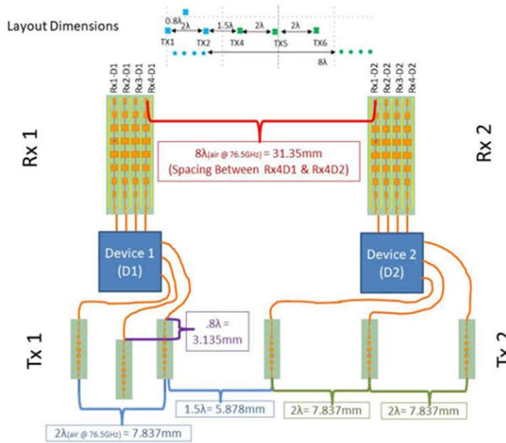
**Figure 4-1. TX and RX Channel Spacings**
