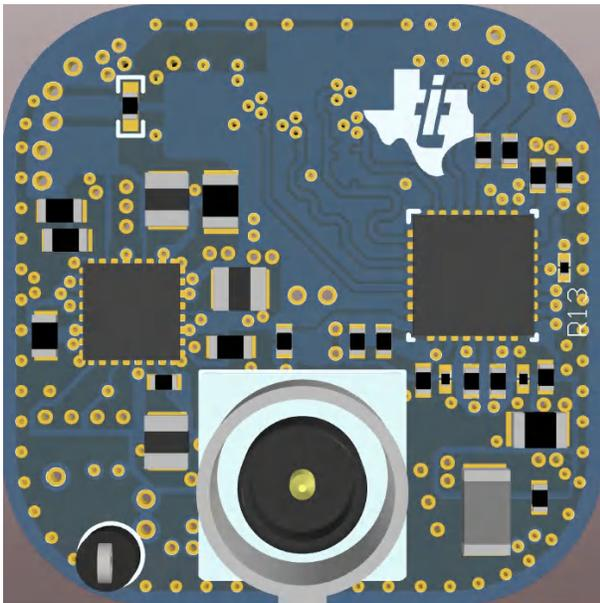
Figure 2-2. 3-D PCB Base Board (Top)
