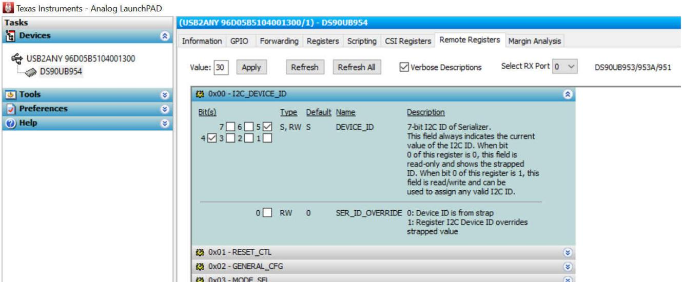
**Figure 3-10. Serializer Remote Registers**
