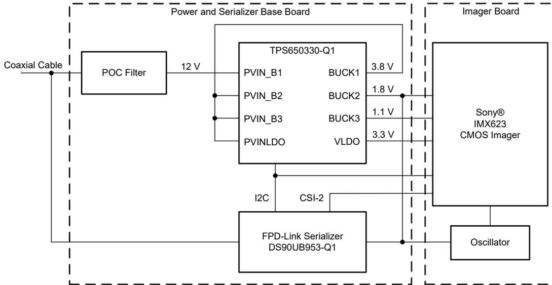
Figure 2-1. TIDA-050060 Block Diagram
