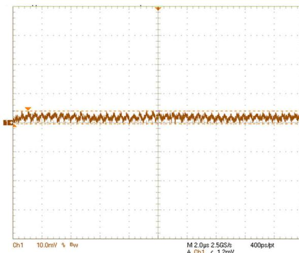
**Figure 3-8. Output Voltage Ripple: 3.3 V**
