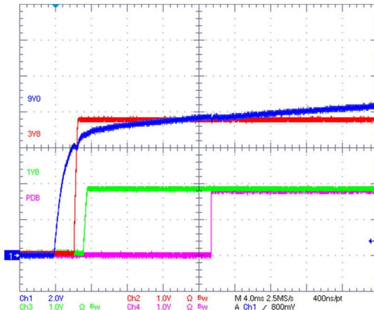
Figure 3-4. Serializer Power-Up Sequence
