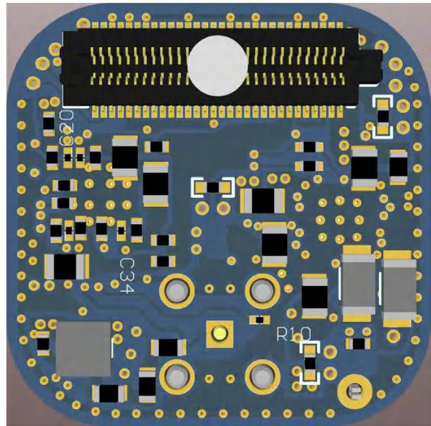
Figure 2-3. 3-D PCB Base Board (Bottom)
