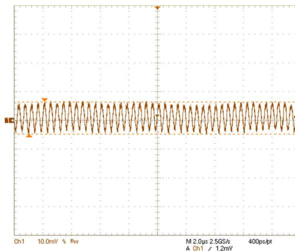
Figure 3-6. Output Voltage Ripple: 1.8 V
