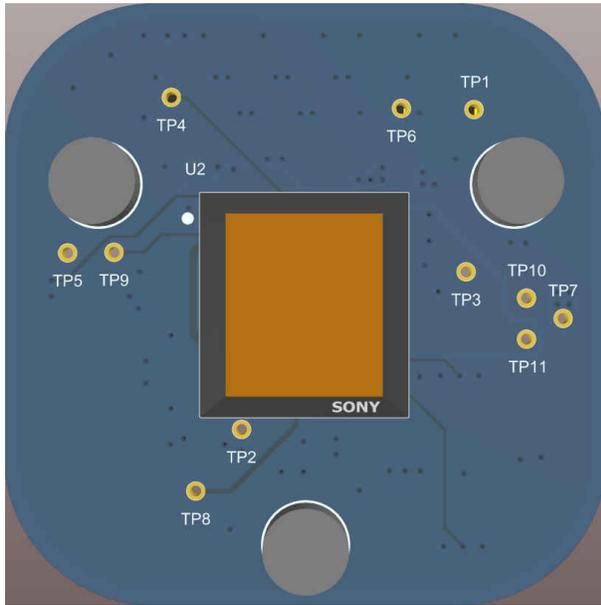
**Figure 2-4. 3-D PCB Imager Board (Top)**
