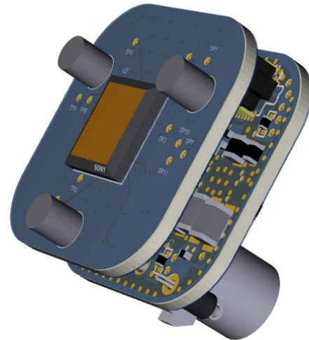
**Figure 2-7. 3-D PCB Assembled Boards (Angled View)**
