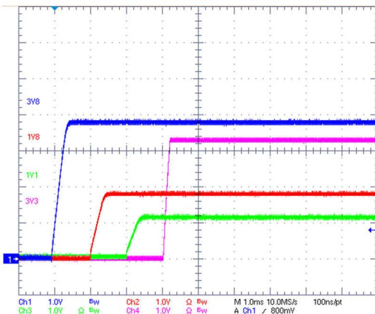
**Figure 3-3. Point-of-Load Power Supply Start Up**
