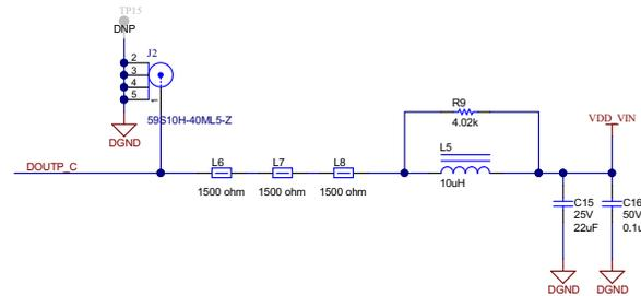
**Figure 1-1. POC Filter Schematic**
