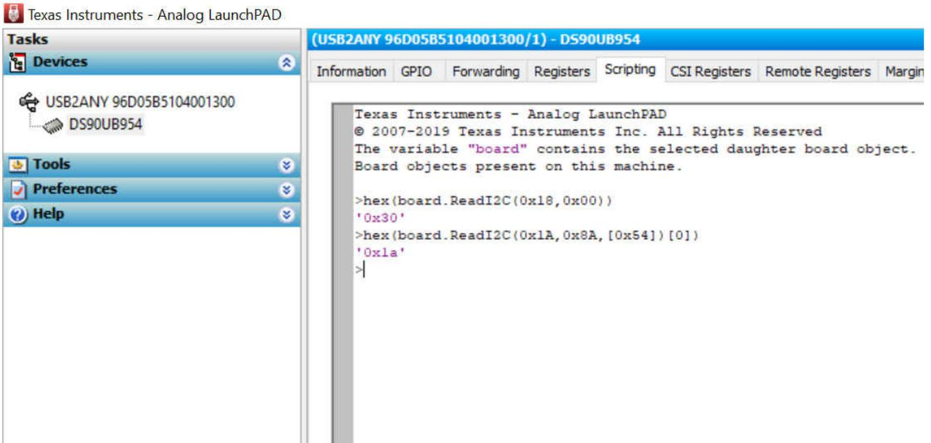
**Figure 3-11. Back-Channel I2C Communication**
