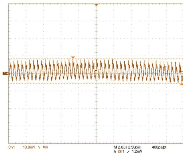
Figure 3-5. Output Voltage Ripple: 3.8 V
