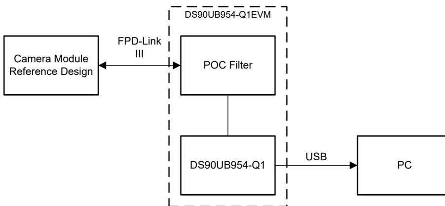
Figure 3-2. Test Setup
