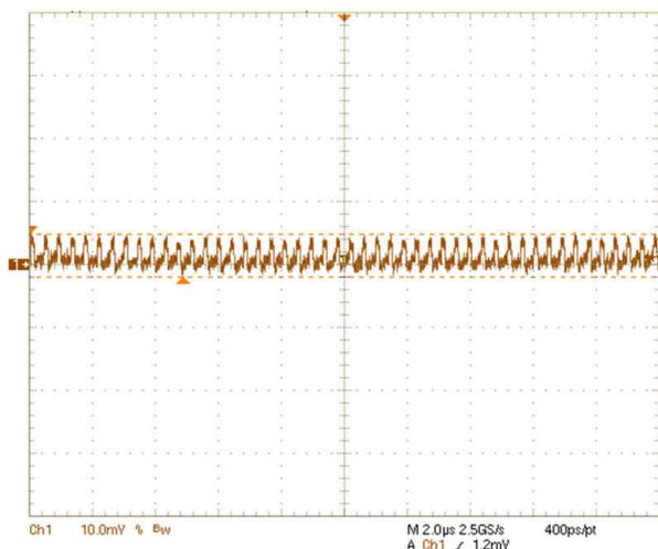
**Figure 3-7. Output Voltage Ripple: 1.1 V**
