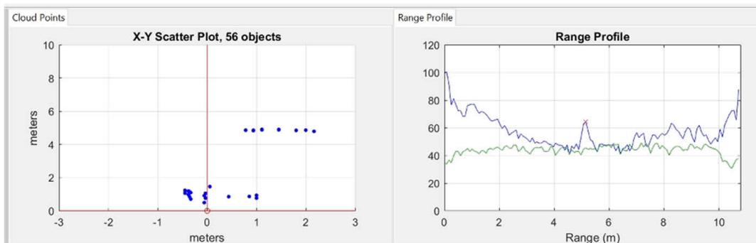
**Figure 3-10. Detection Point Cloud of Parking Block**
