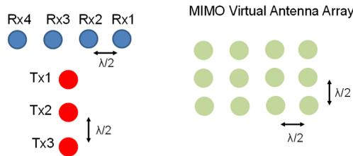
**Figure 2-4. AWR1843AOP Antenna Virtual Array**
