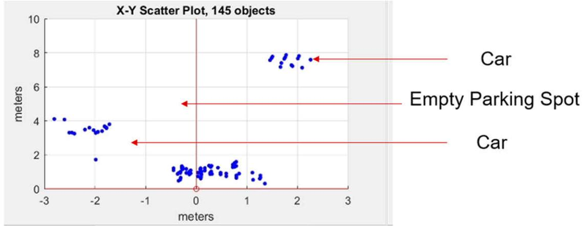
**Figure 3-8. Detection Point Cloud of Empty Parking Space**
