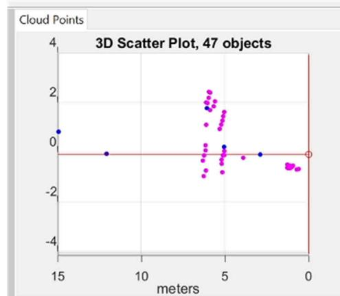
**Figure 3-3. Detection Point Cloud of Traffic Sign Pole – Elevation View**
