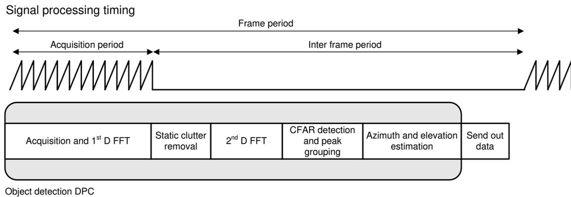
**Figure 2-2. Datapath Processing and Timing**
