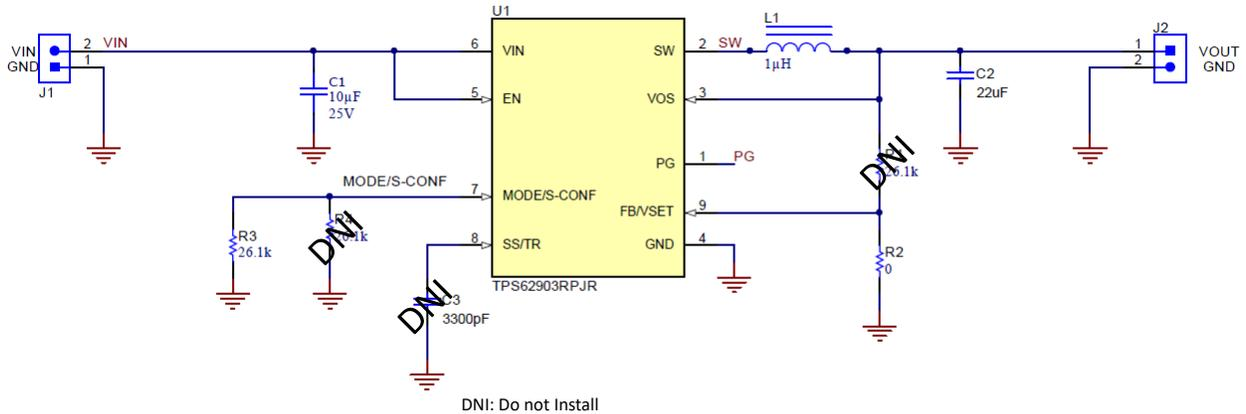
**Figure 2-2. Buck Converter Circuit Design Using TPS62903**
