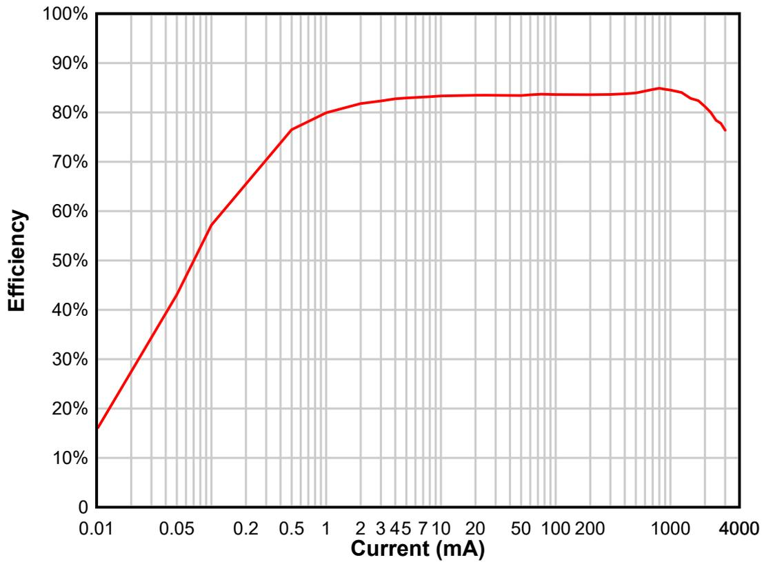
Figure 3-8. Efficiency Data with 12-V<sub>in</sub>, 1.2-V<sub>o</sub>, up to 3-A Load.
