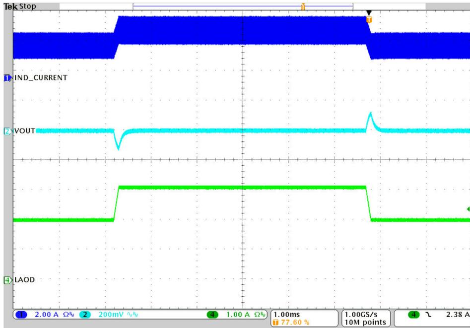
**Figure 3-5. Load Transient 2-A to 3-A with 12-Vin**
