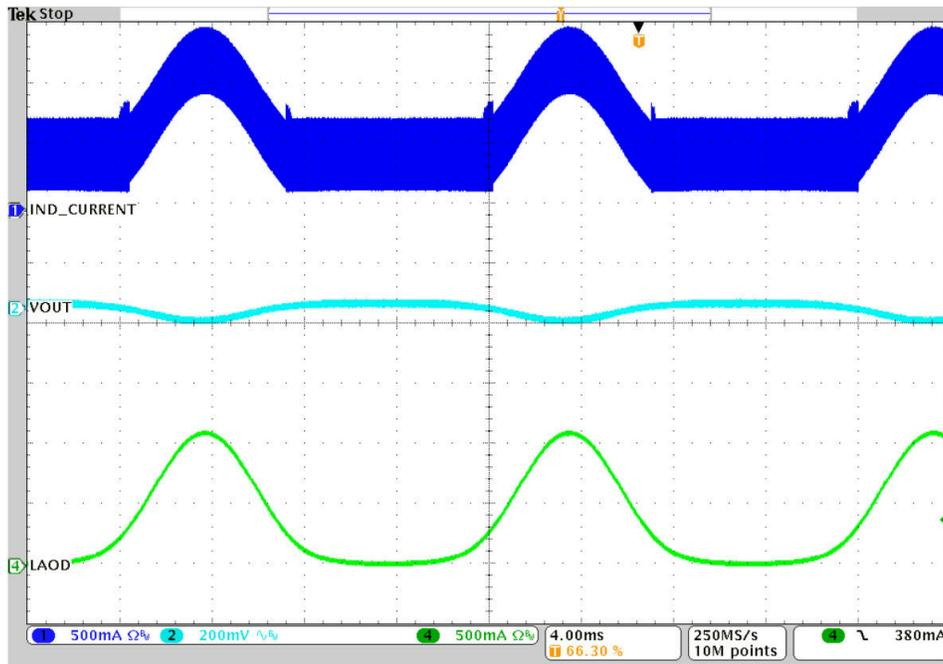
Figure 3-6. PSM to PWM Transition with 5-Vin
