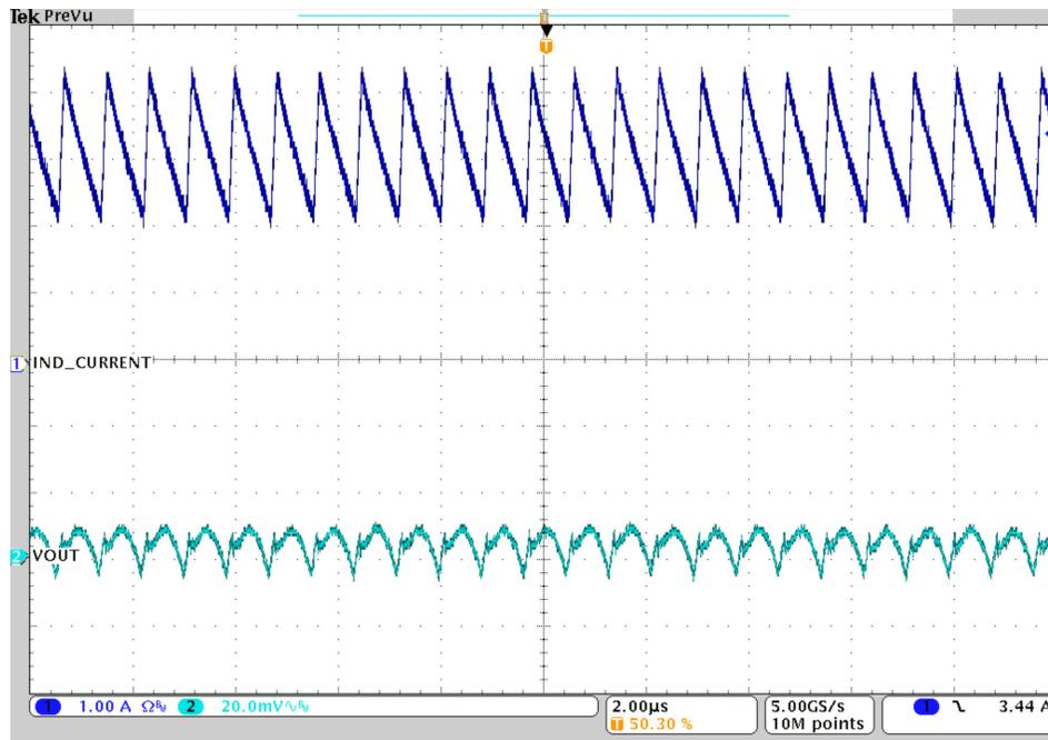
Figure 3-7. Vout ripple at 3-A
