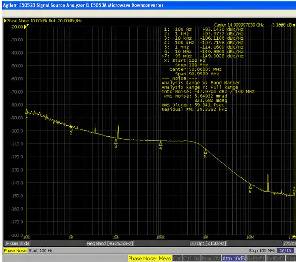
Figure 4-7. Phase Noise at 15-GHz Carrier Frequency
