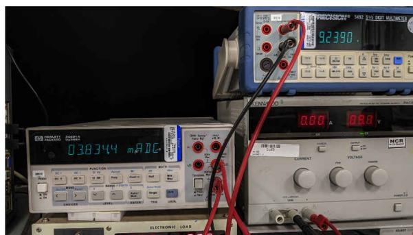
Figure 3-19. Constant Current Output Test Setup (9 V Applied)
