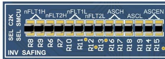
**Figure 3-4. Selection Between C2000 and Safety MCUs to Connect ASC and nFLT**
