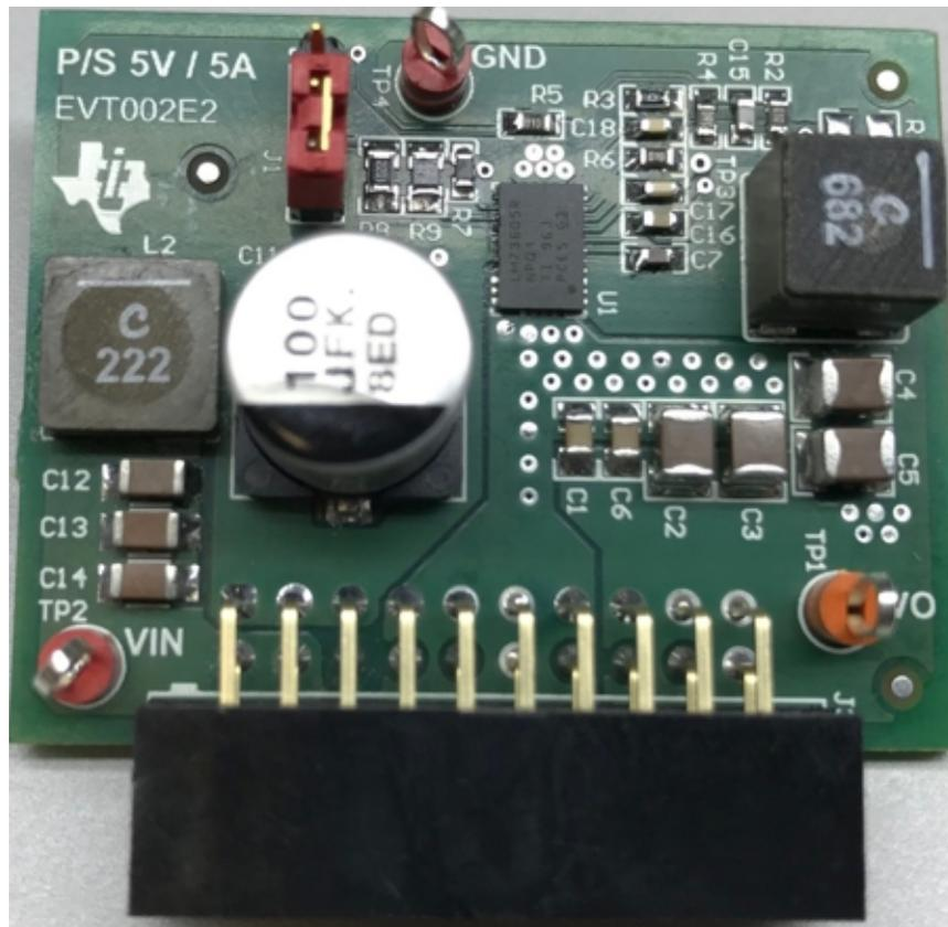
**Figure 3-12. Vbat to 5V/ 5A power supply module**
