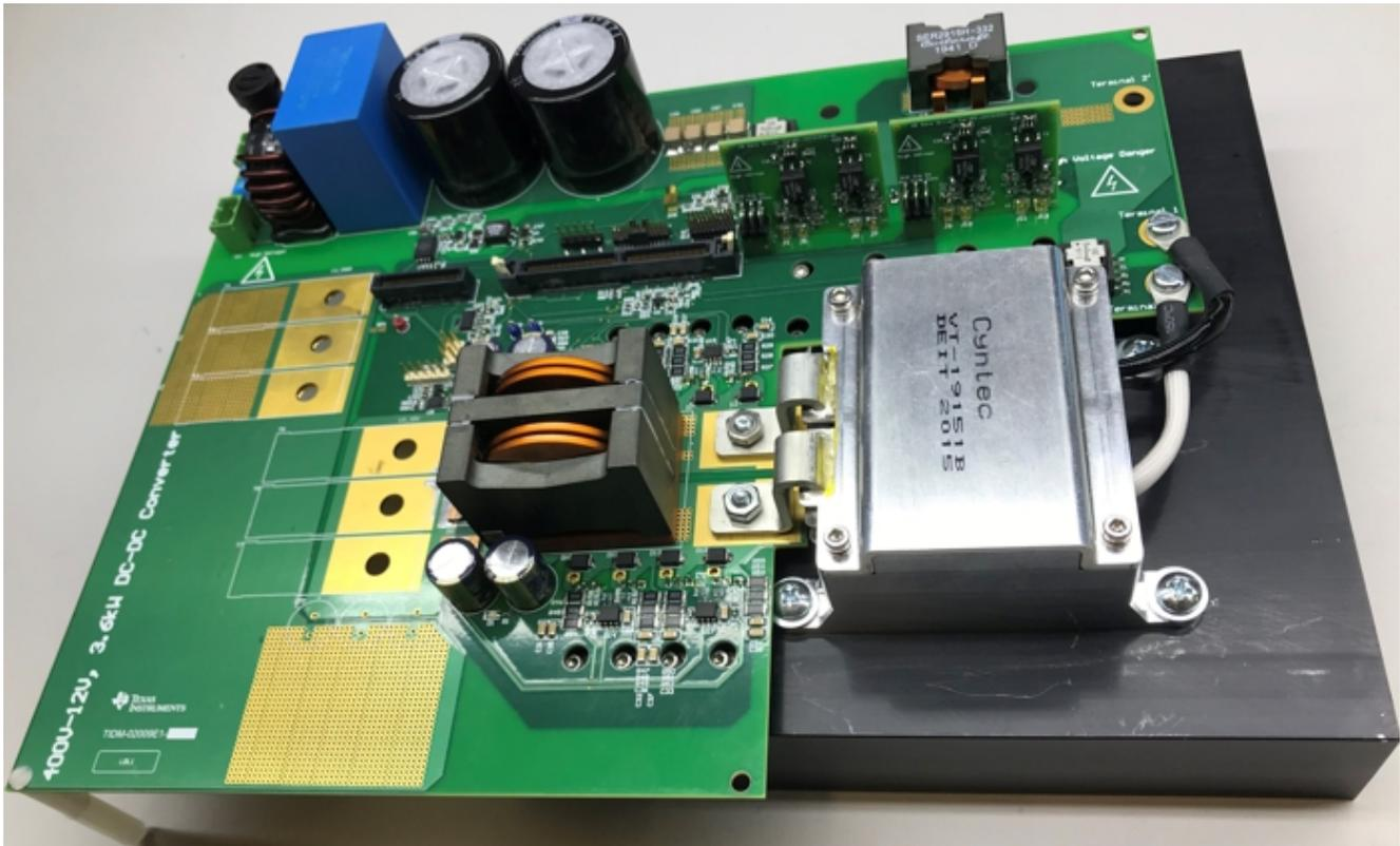
**Figure 3-27. DC-DC Converter Module**
