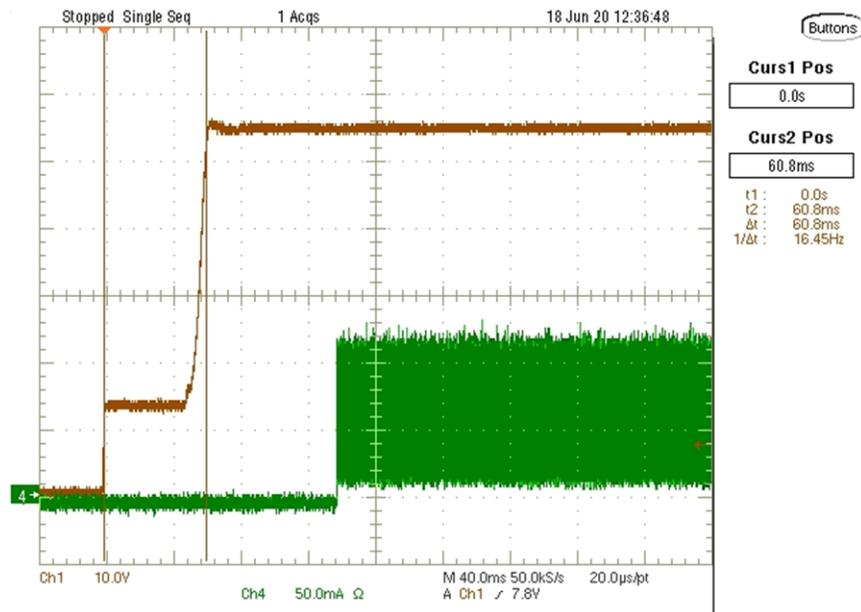
**Figure 3-5. Boost Turn on Delay**
