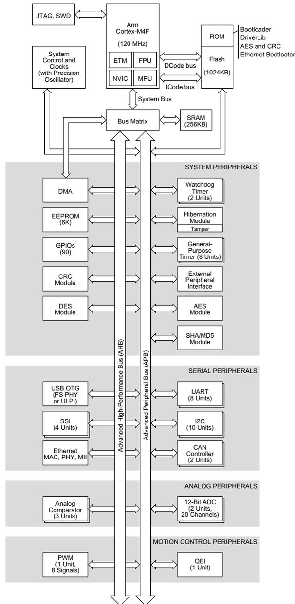
Figure 2-4. MSP432E401Y Functional Block Diagram
