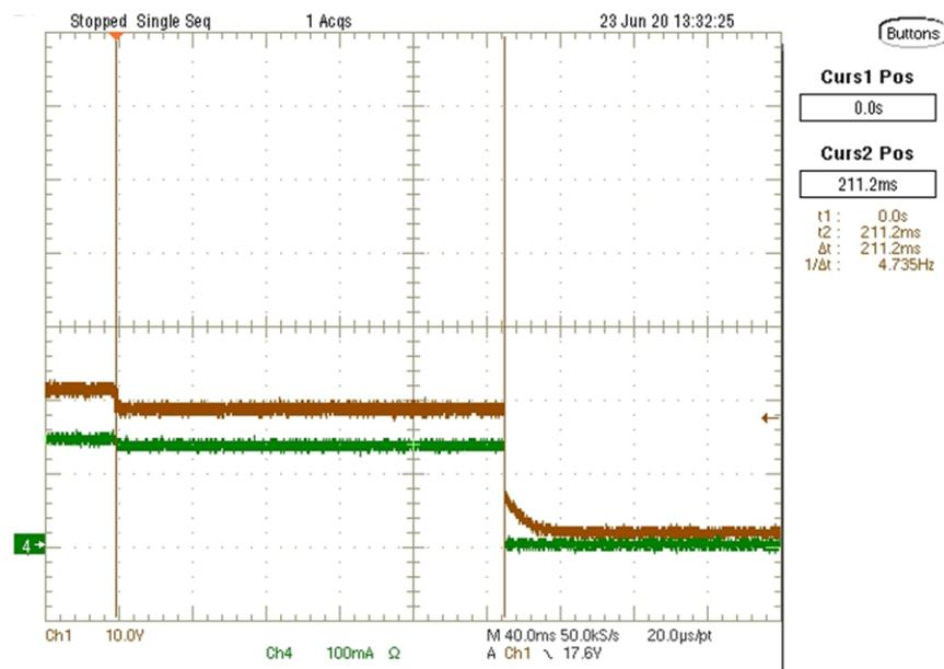
Figure 3-14. Highbeam/Lowbeam LED Short
