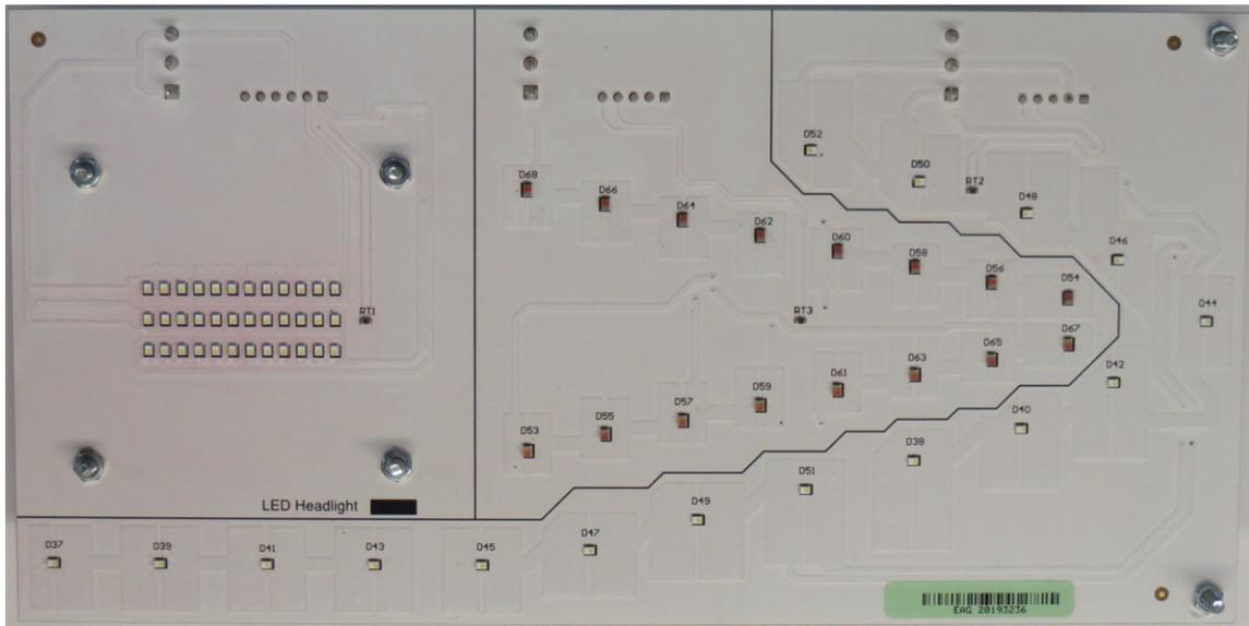
Figure 3-3. LED Load Board Top
