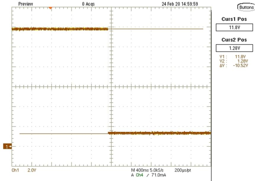
Figure 3-16. Turn Indicator Fault Output
