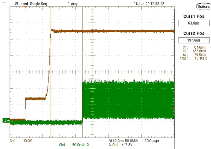
Figure 3-6. Highbeam/Lowbeam Turn on Delay
