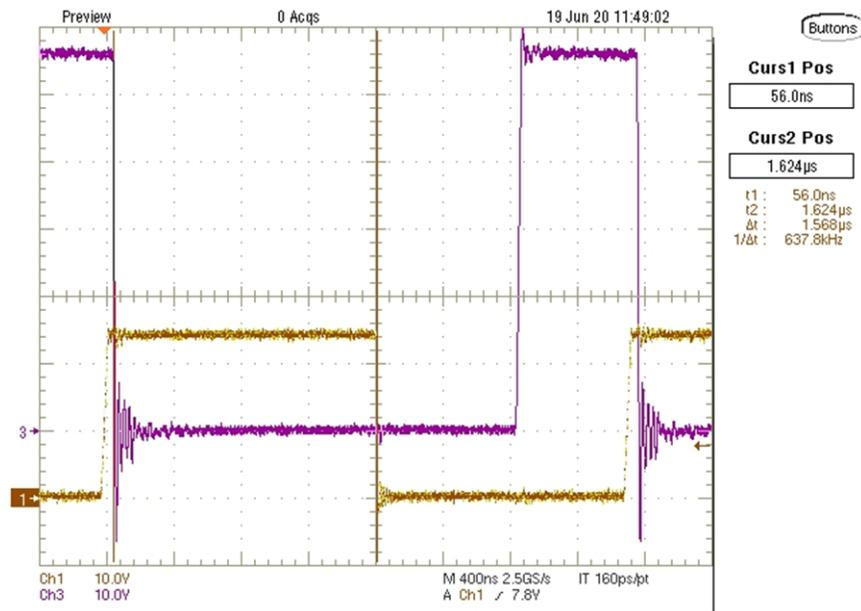
Figure 3-17. TPS92682-Q1 Boost and SEPIC Interleaving
