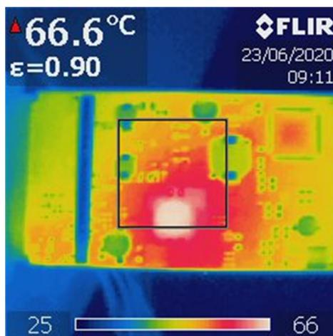
Figure 3-24. Bottom side thermal image DRL at 15W
