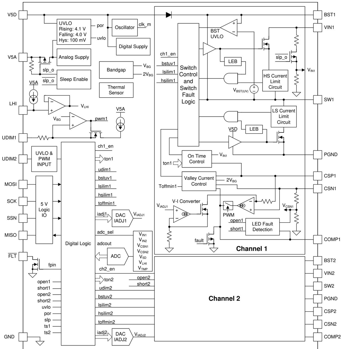
Figure 2-3. TPS92520-Q1 Functional Block Diagram
