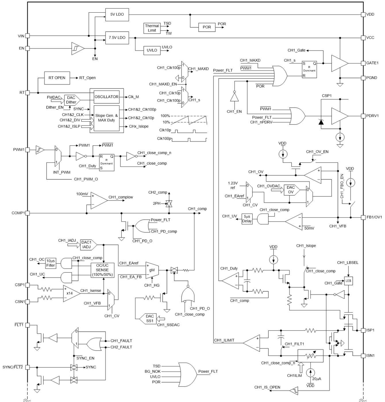
Figure 2-2. TPS92682-Q1 Functional Block Diagram
