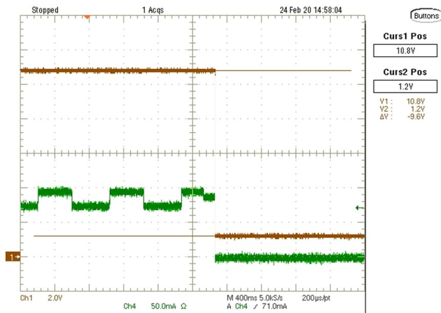
Figure 3-15. Highbeam/Lowbeam Fault Indicator
