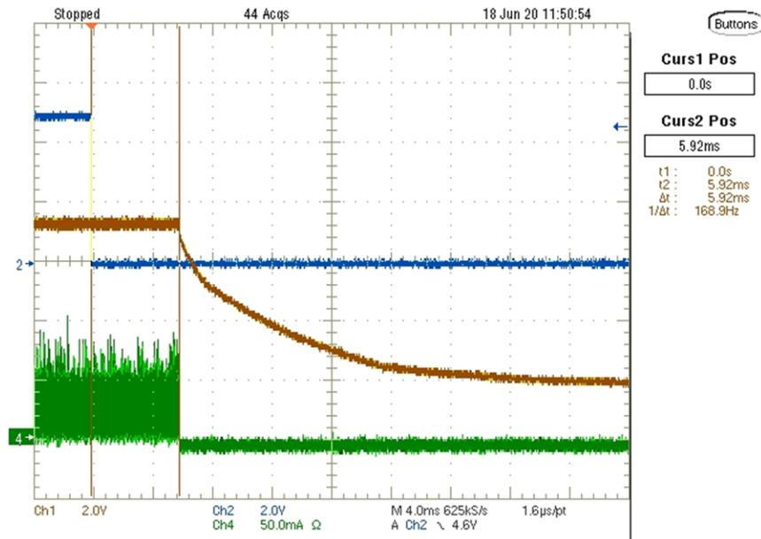
Figure 3-9. Turn Indicator Turn Off Delay
