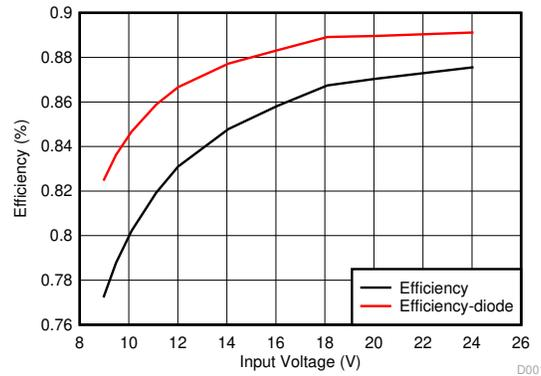
Figure 3-18. TIDA-050040 Full Load Efficiency
