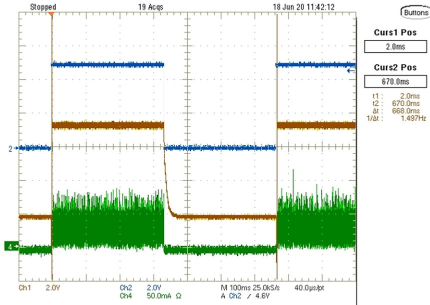
Figure 3-10. Turn Indicator 1.5 Hz Operation
