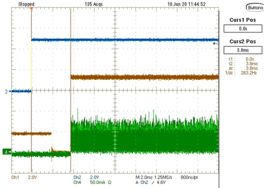
Figure 3-8. Turn Indicator Turn on Delay
