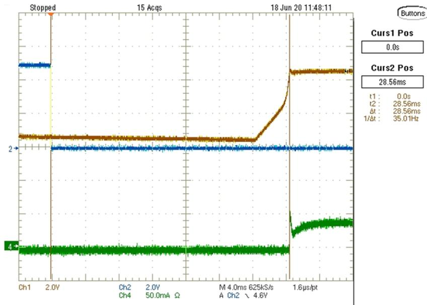
Figure 3-12. Daytime Running Light Turn-on Delay
