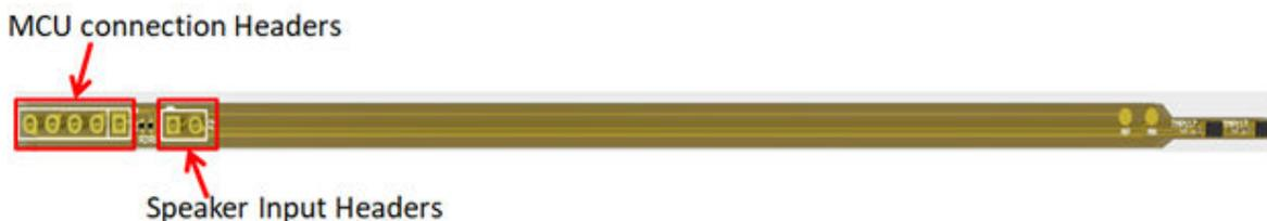
Figure 2-4. MCU and Speaker Input Headers
