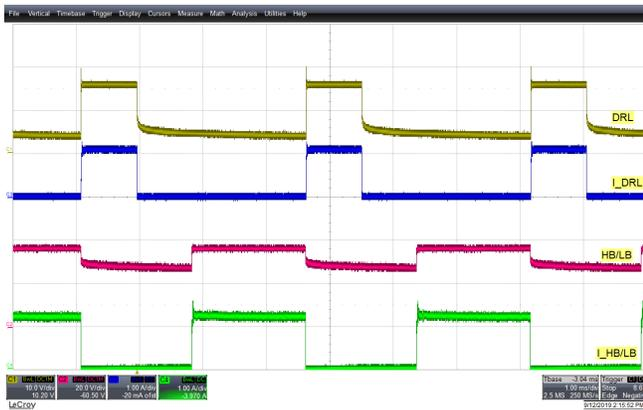
**Figure 18. 10% PWM'ing at High Power**
