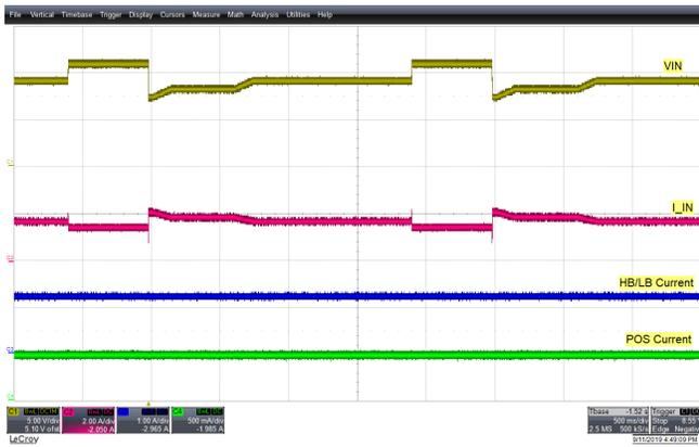
Figure 24. DRL/POS Open Protection
