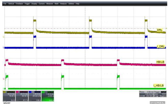
**Figure 19. 90% PWM'ing at Low Power**
