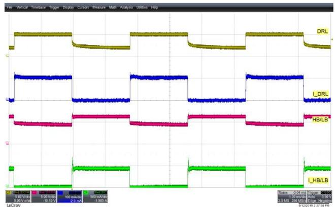
Figure 21. 10% PWM'ing at Low Power
