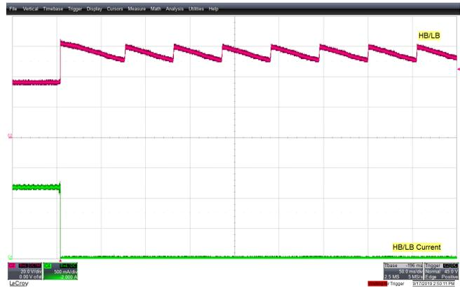
Figure 27. High Beam and Low Beam Short Protection
