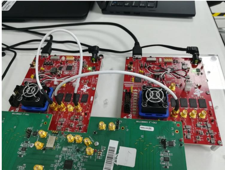
**NOTE:** Figure 21 illustrates that the length of cable must be length matched
