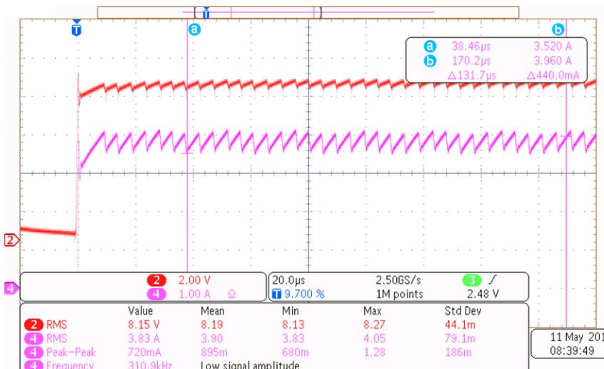
**Figure 5. 0.4-A LED Amplitude at 18-V Input Voltage**
