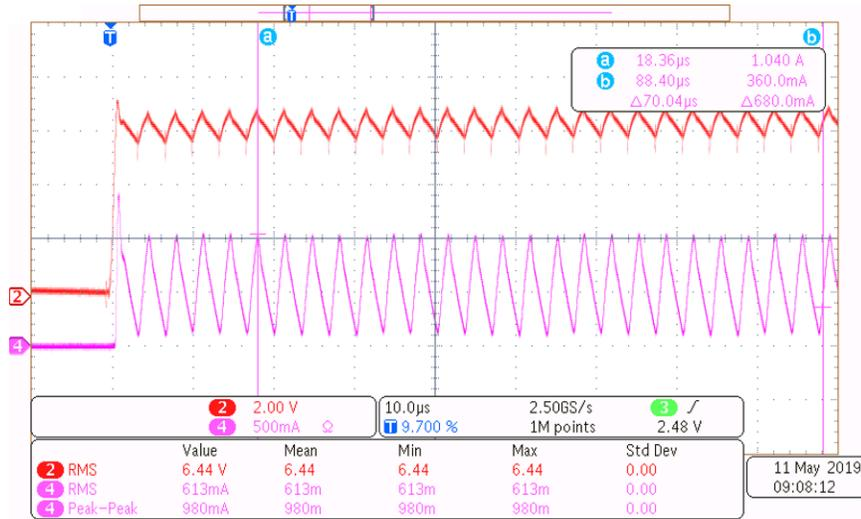
**Figure 6. 0.4-A LED Amplitude at 10-V Input Voltage**
