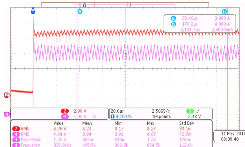
**Figure 4. 4-A LED Amplitude at 10-V Input Voltage**
