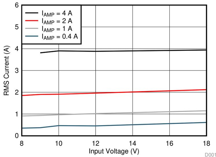
**Table 3. Percent Change in LED RMS Current With Varying Input Voltage**
