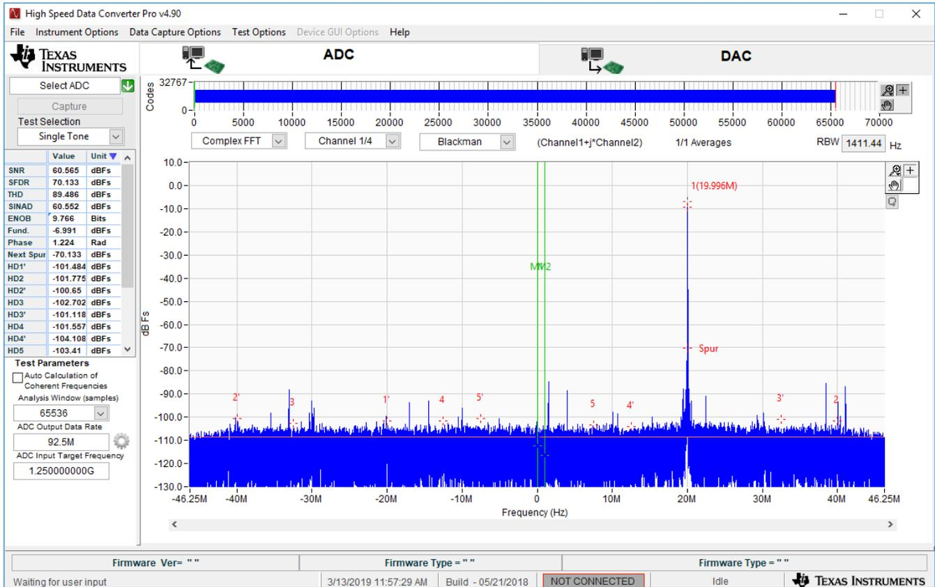
Figure 36. ADC2 Spectrum - Q Data,  $F_s = 1480$  MHz,  $F_{NCO} = 1270$ ,  $F_{in} = 1250$  MHz
