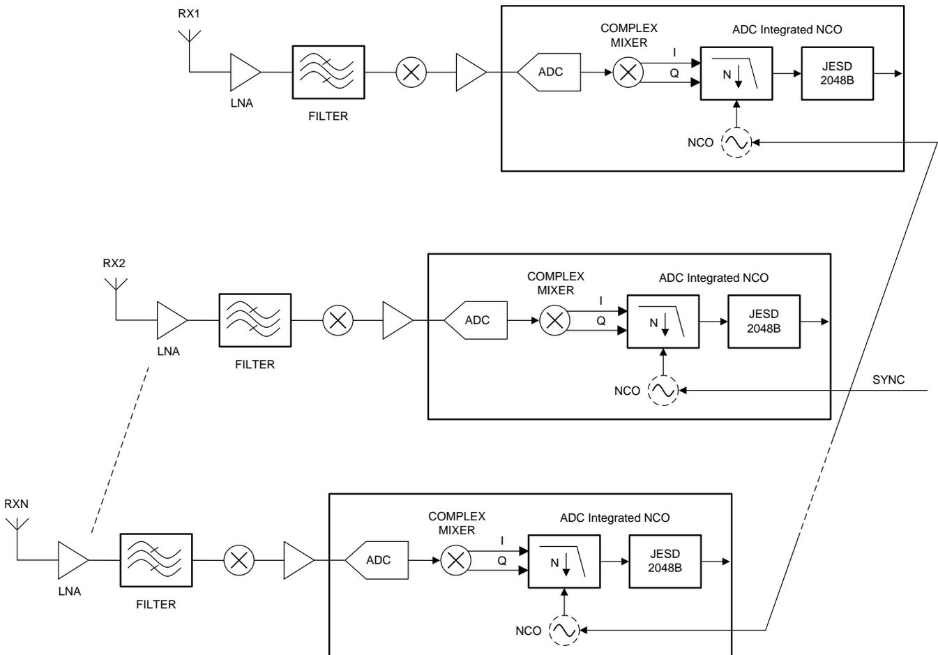
However, in multi-chip synchronization in sampled systems, it is crucial that samples from multiple receivers are aligned exactly with each other. Even a single clock cycle misalignment cannot be tolerated. Synchronization of multiple receivers requires timing calibration, careful routing, and a detailed timing analysis to ensure that the propagation delay across different analog-to-digital converters (ADCs) does not result in channel-to-channel skew that is greater than one clock cycle.
