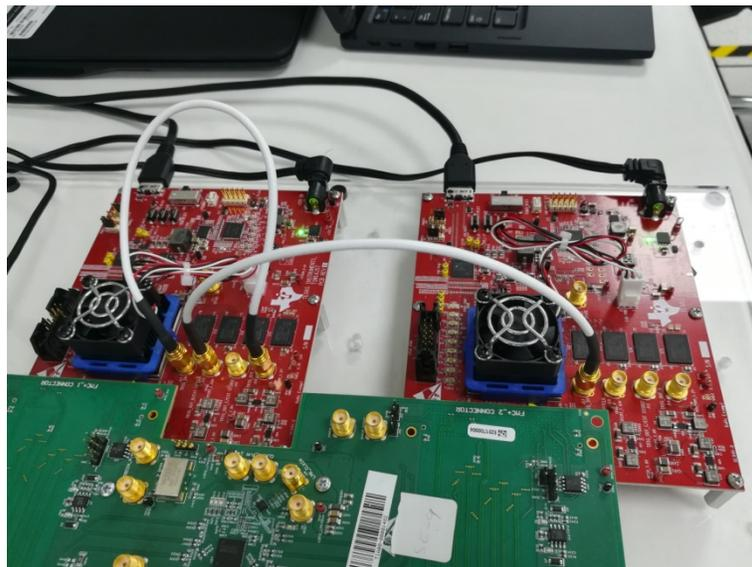
**NOTE:** Figure 27 illustrates that the length of cable must be length matched.
