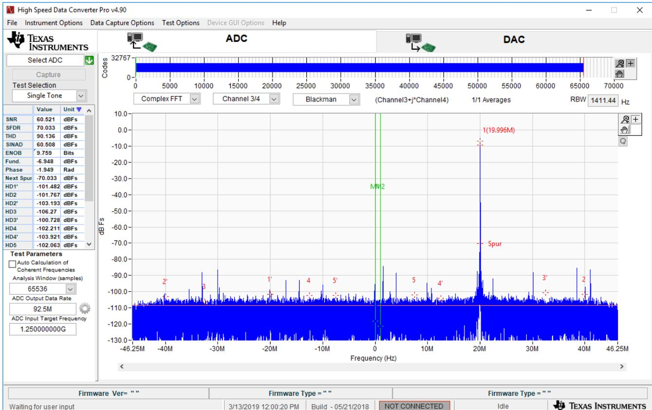
Figure 37 and Figure 38 show the SNR and SFDR performance curve for sampling frequency  $F_s = 1480$  MHz, NCO frequency  $F_{NCO} = 1250$  and input frequency  $F_{in}$  1200 MHz to 1290 MHz.
