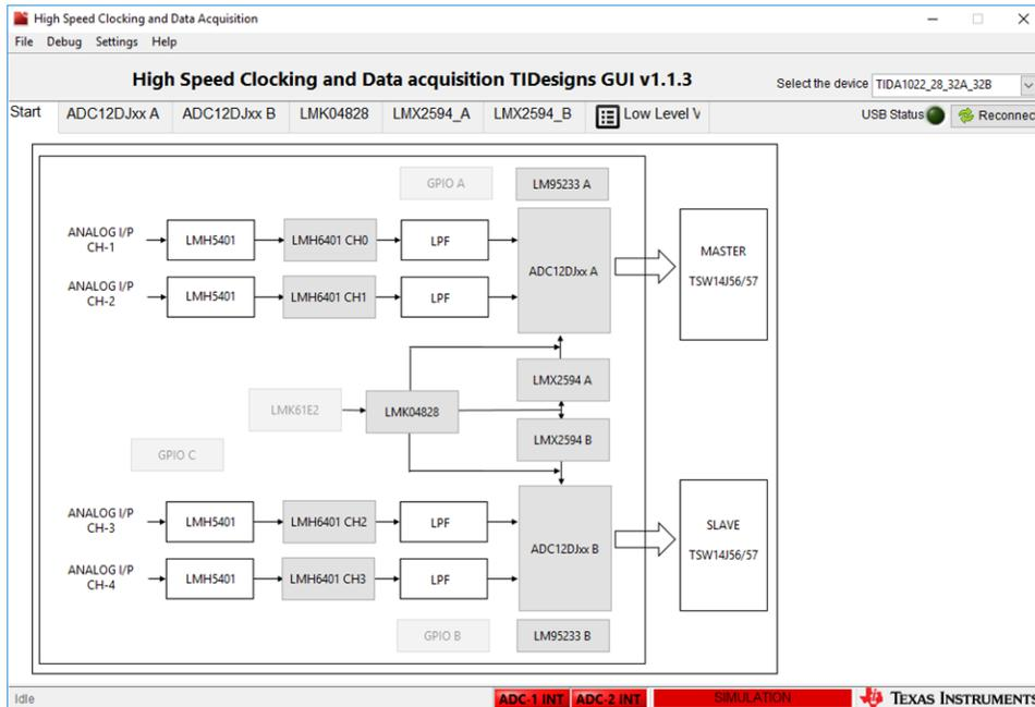
Figure 17. HSDC TID GUI – Low-Level Programming View
