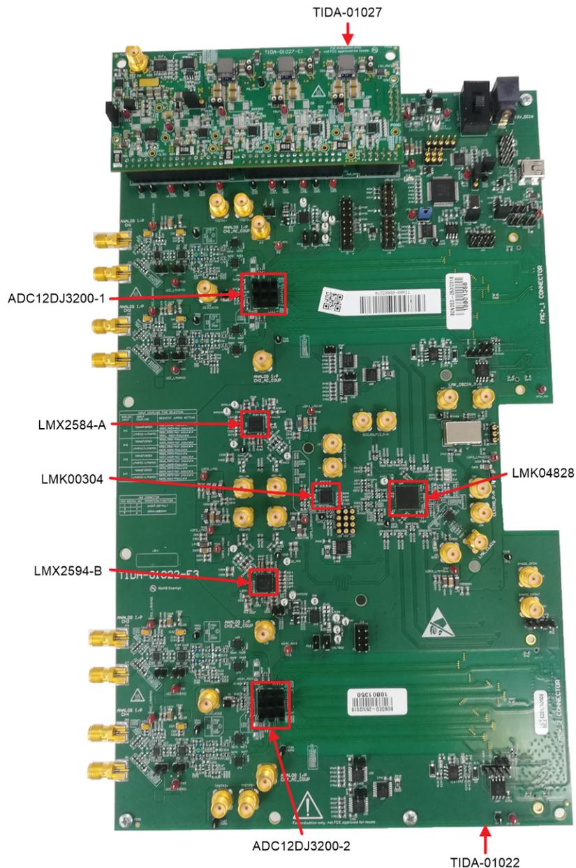
Figure 15 shows the TIDA-01027 board image, in this reference design the TIDA-01027 board is configured as DC/DC free running mode (default mode). The TIDA-01027 output connectors are made compatible with the TIDA-01022 power input headers J58, J59, J60, and J63.
