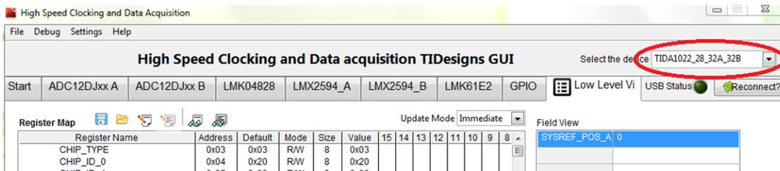
2. Navigate to the *Low Level* tab, select the configuration files to be programmed, and click the *OK* button. Follow these steps as numbered and encircled in the screen shot in Figure 22.
