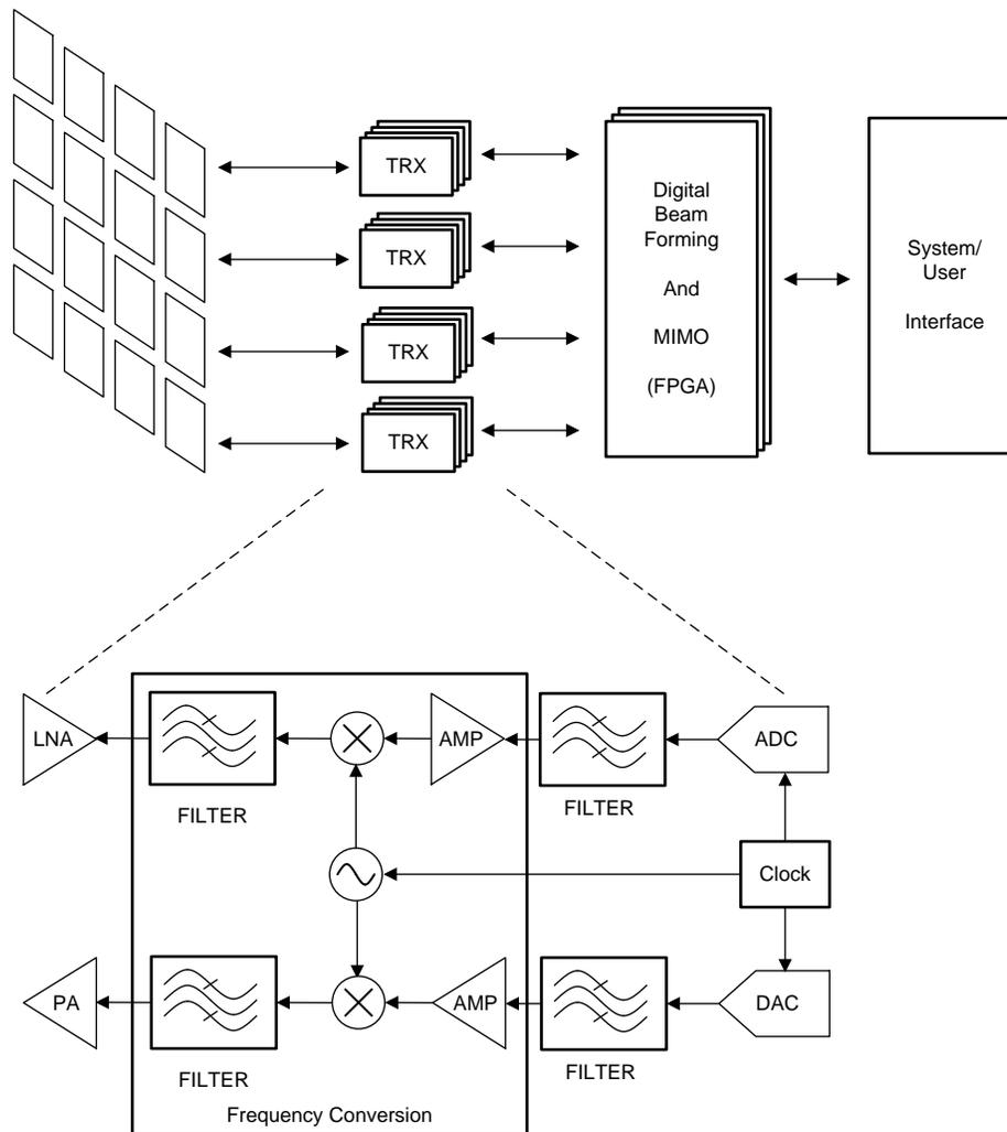
Similarly RADAR, electronic warfare, satellite communication payloads require large numbers of transceivers (transmit and receive signal chain) in their applications.
