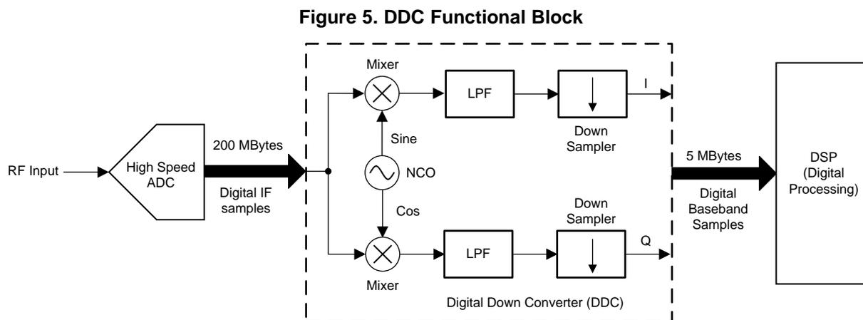
Due to applications needs, digital down conversions are done at the RF front end (analog domain) or after digitization in FPGA or DSP processors (digital domain), or a combination of both approaches. These digital features are built into new RF ADCs which further reduces system complexity, software flexibility to choose decimation, NCO frequency, and footprint.
