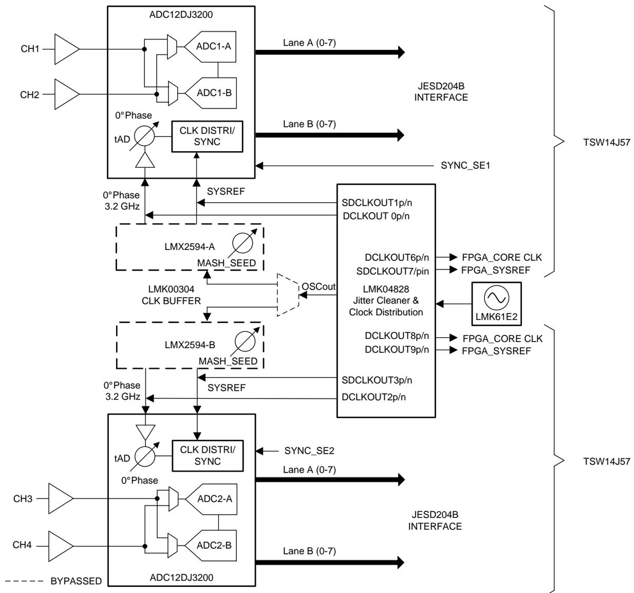
In this reference design ADC12DJ3200 operated in decimation mode (JMODE15 and JMODE16).
