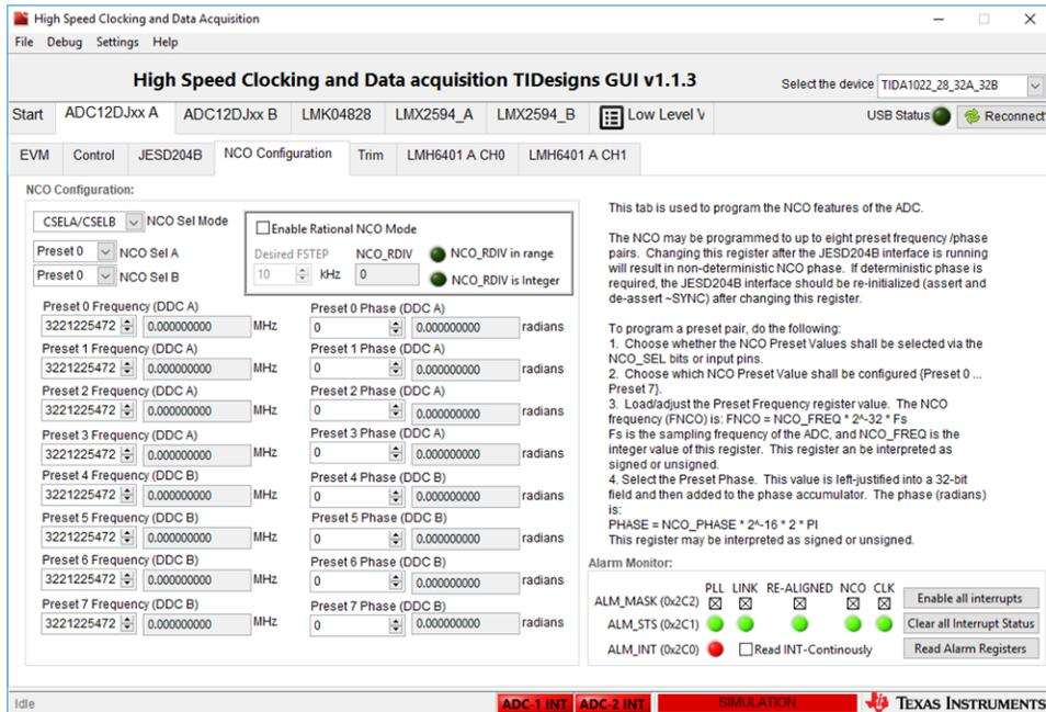
Figure 19 shows the ADC capture screen in HSDC Pro GUI
