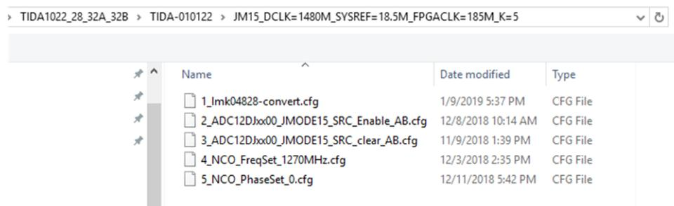
3. Configure both ADC12DJ3200 JMODE15 (x16 decimation) by loading the configuration file in the *Low Level*/page of the HSDC Pro GUI in the following order for both master and slave capture card:
