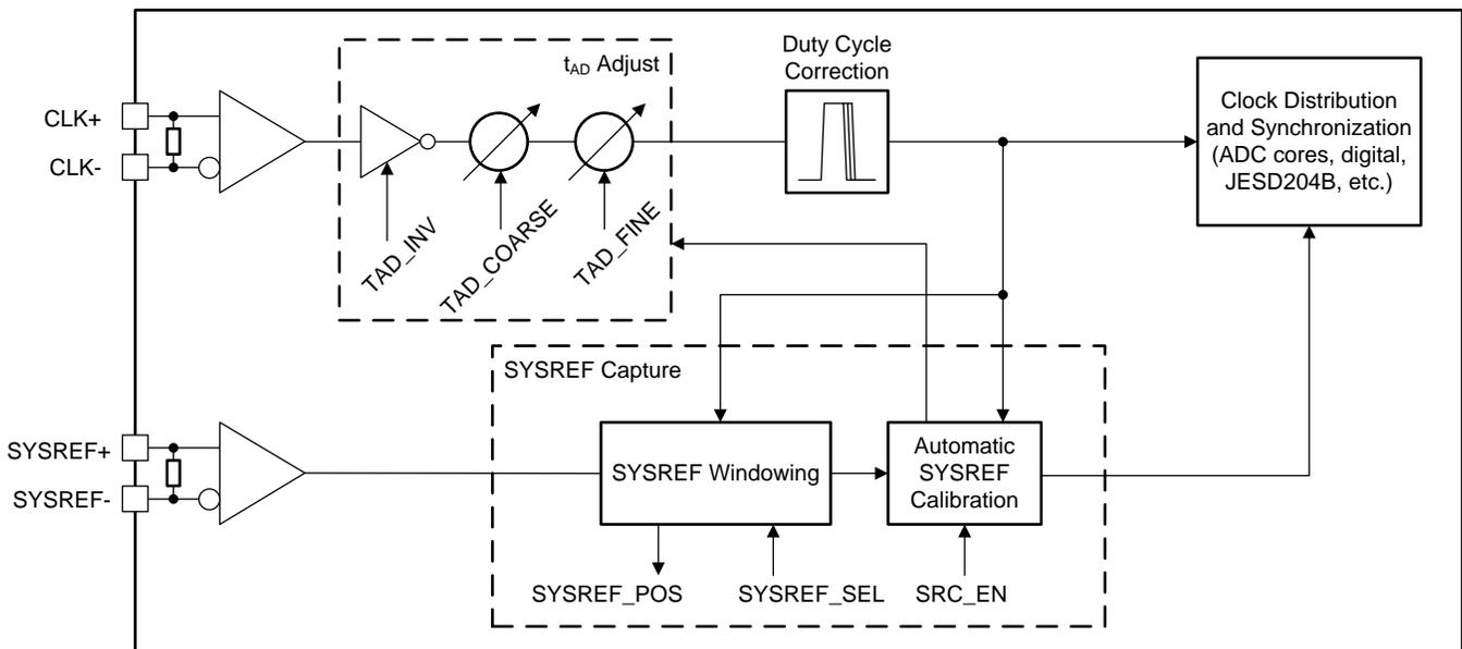
This  $t_{AD}$  feature gives the flexibility to adjust  $t_{AD}$  registers to align the sampling instants across multiple ADCs with 19-fs resolution.
