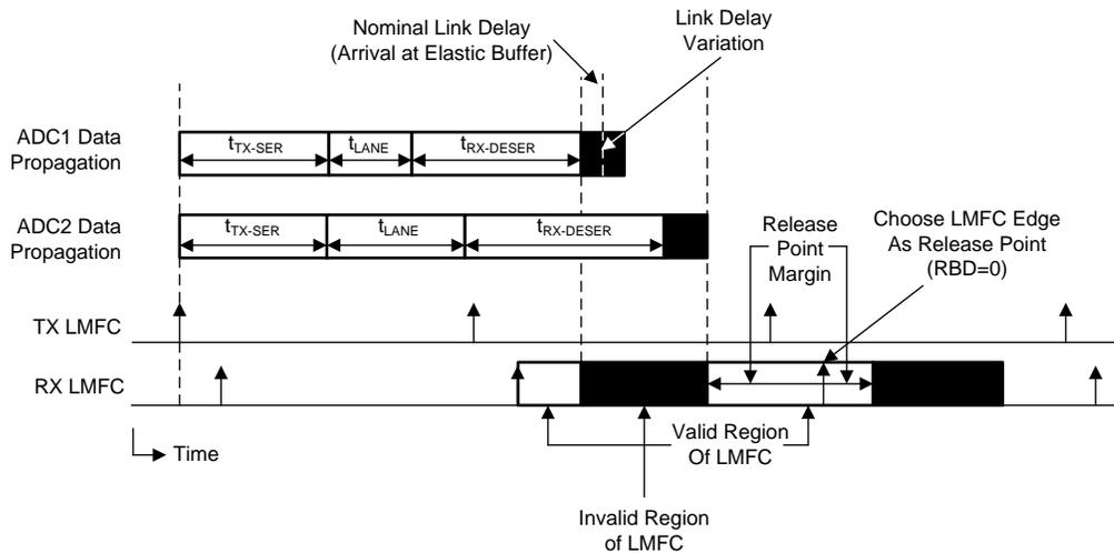
Determine the invalid region of LMFC period, then set the release buffer delay (RBD) parameter to shift the release point with number of frame clock from the LMFC edge so it occur within valid LMFC cycle.
