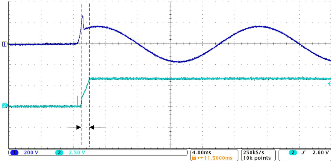
**Figure 16. Startup Time for Half-Bridge Off-Line Switcher**
