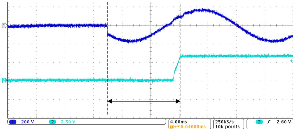
In the case of switch-cap regulator, startup time depends mainly on the passive elements around TPS7A78 since all the capacitors need to be charged to the specific value to start generating output voltage. Figure 17 and Figure 18 shows startup of the half-bridge and full-bridge configurations for the values mentioned in the Section 2.4.3. The half-bridge has more than two times the startup time as the full-bridge since it rectifies the input voltage in only half of its cycle.
