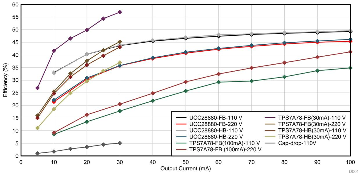
The efficiency of the discrete cap-drop regulator for 110 VAC input while sweeping the output current from 5 mA to 30 mA is in the range of 1–5%. Most of the power is dissipated in series resistor  $R_S$ , and a Zener diode which results in poor efficiency of the converter. There is a standby power loss of 1.8 W which is present independent of the load requirement.
