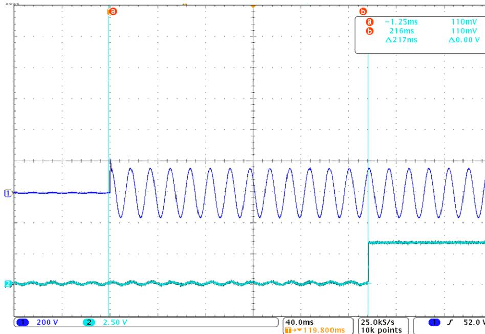
**Figure 18. Startup Time for Full-Bridge Switch-Cap Regulator**
