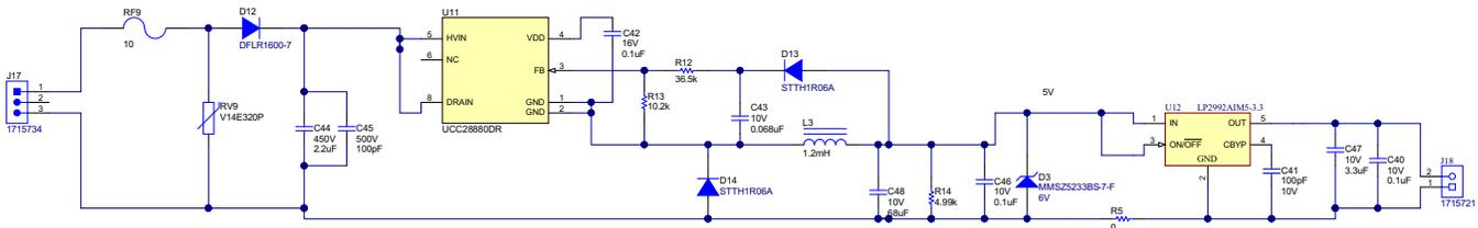
Figure 7. Off-Line Buck Converter for Full-Bridge Configuration Schematic
