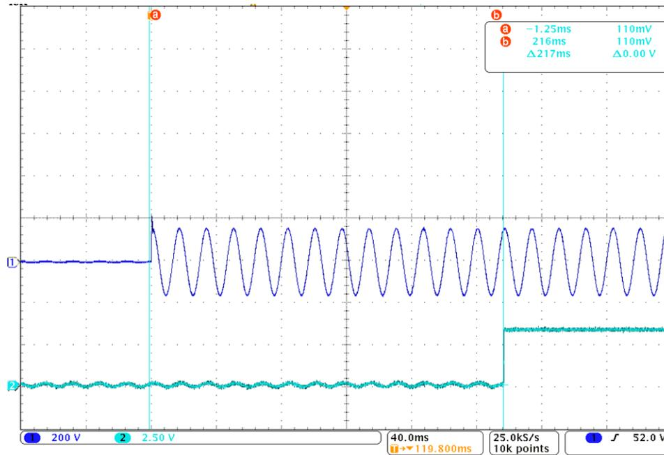
Figure 14 shows the startup time for the cap-drop regulator when 110 Vac is applied. It has the largest startup time of 350 ms to reach from 0 to 3.3 V.
