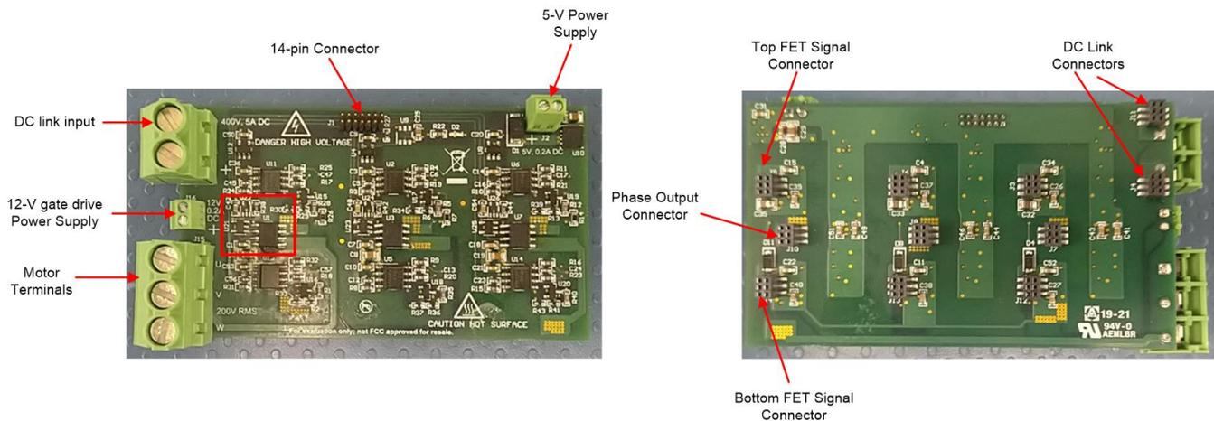
The current-sensing circuit for phase U is shown highlighted within the red box in Figure 13. Each phase has a dedicated current sensor, voltage reference, and buffer op amp for phase current-signal processing. A single-voltage reference can be used for all three phases - dedicated references are used in the TIDA-010059 design for ease of routing.
