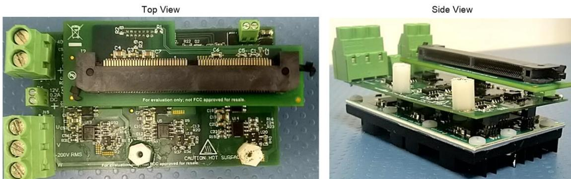
The C2000 control card can be slotted into the HSEC8 120-pin connector on the interface PCB as in Figure 17.
