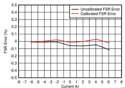
Figure 22 shows that the FSR Error in % across the measured current range at a switching frequency of 32 kHz. The uncalibrated error is within  $\pm 0.2\%$  and the calibrated error is within  $\pm 0.03\%$ .
