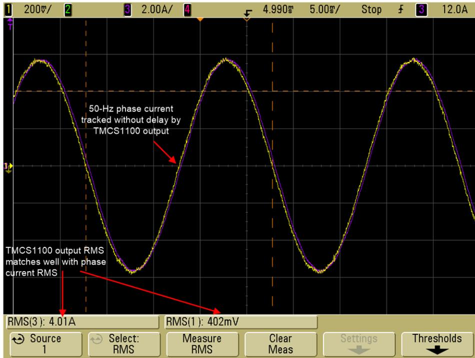
Figure 25 shows the phase current and TMCS1100 output (post R-C filter) within a switching time period in the presence of switching noise. Observe that the TMCS1100 device follows the phase current accurately with negligible delay enabling high-performance control.
