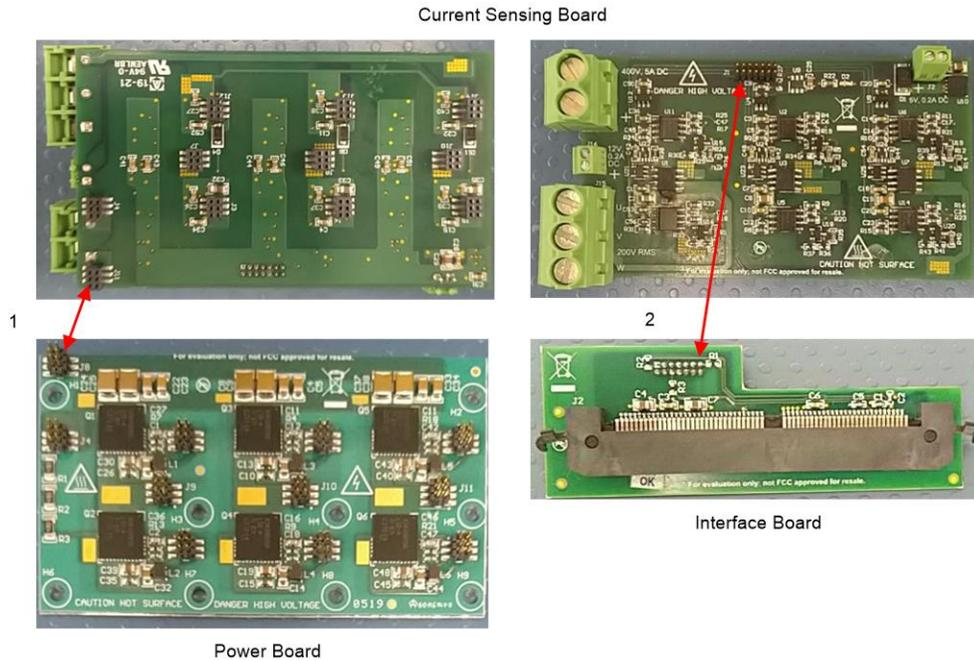
Figure 16 shows the top and side views of the assembled TIDA-010059 design boards.
