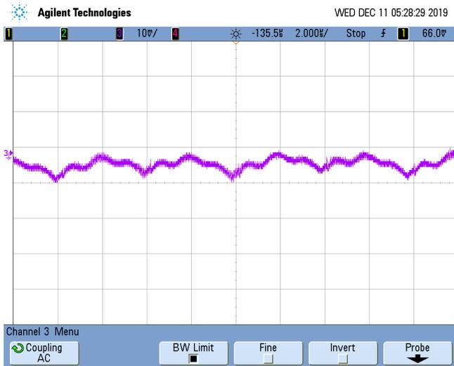
Figure 30. Output Ripple of Negative Rail After Power Filter
