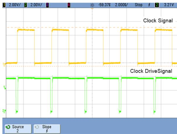
**Figure 19. Synchronization at Full Load With 50% Duty Cycle Clock**
