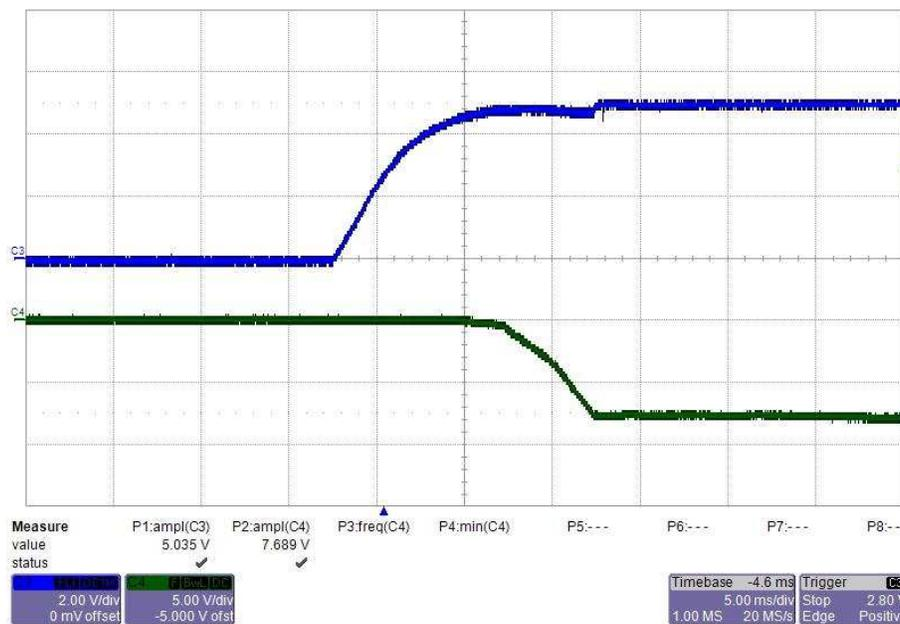
From top to bottom: CH3: input voltage 2 V/div, CH4: output voltage 5 V/div, 5 ms/div
