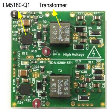
**Figure 12. LM5180-Q1 Based Flyback PCB Board Bottom Side**
