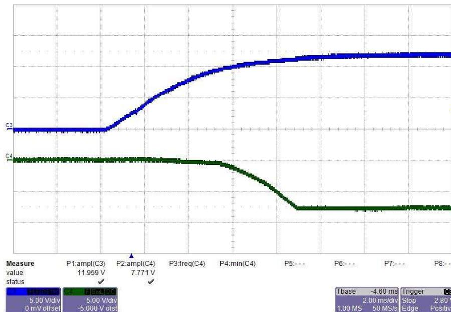
From top to bottom: CH3: input voltage 5 V/div, CH4: output voltage 5 V/div, 2 ms/div
