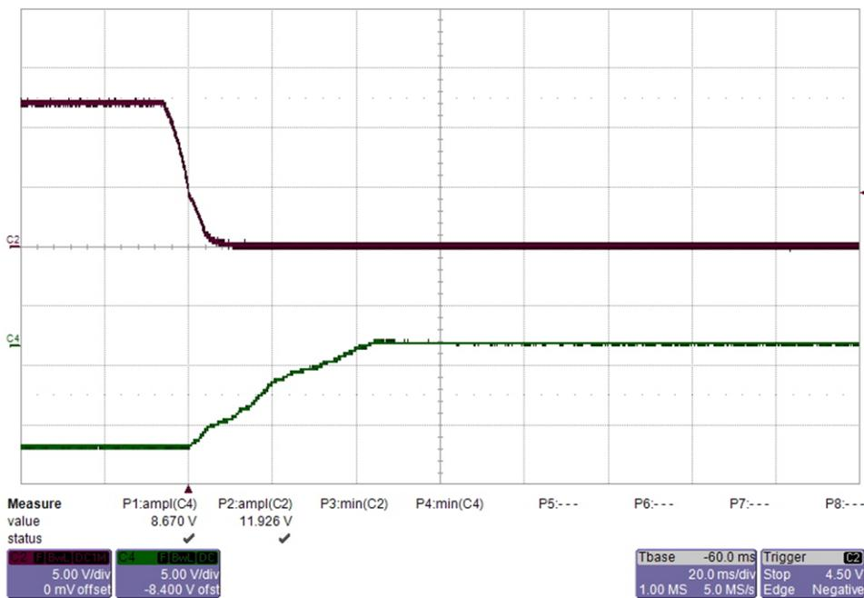
From top to bottom: CH3: input voltage 5 V/div, CH4: output voltage 5 V/div, 20 ms/div
