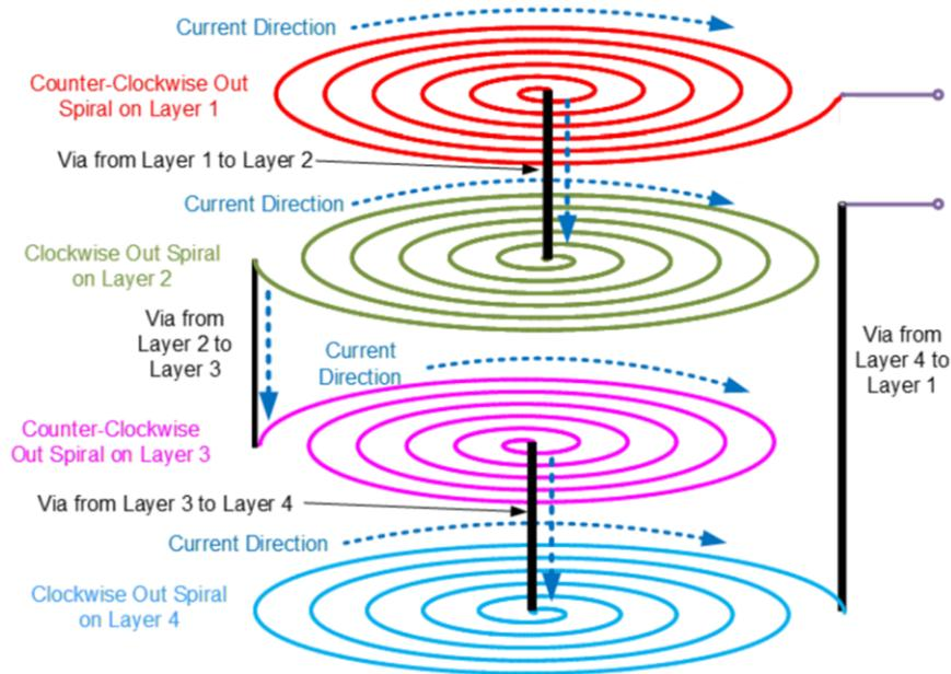
Figure 14. Connection Process of Coils on 4 Different Layers
