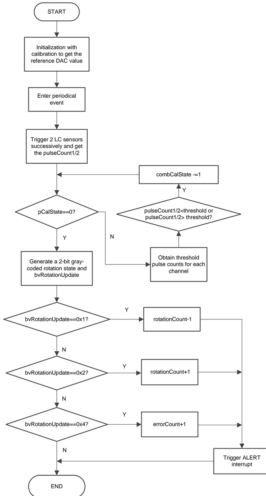
Figure 18 shows the flowchart for LC sensing task in SCE. In the Constants and Data Structures Panel in SCS, there are user-defined parameters which can be tuned for the performance evaluation and optimization, as listed in Table 2.
