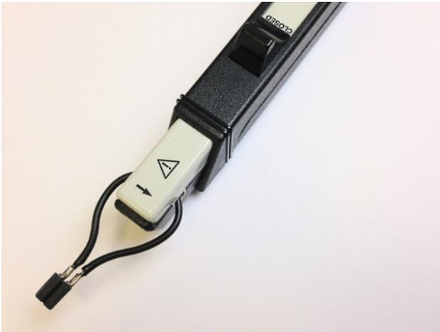
**Figure 19. Probe With Long Ground Lead and Alligator Clip vs Probe With Ground Spring**
