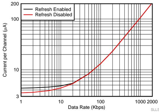
**Figure 50. ISO7041 Supply Current vs Data Rate at 3.3 V (With 15-pF Load)**
