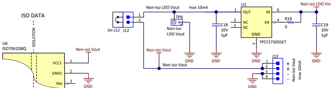
The main purpose of NON-ISO LDO circuit block is to remove the remaining output ripple voltage of the NON-ISO BUCK. The LDO is a 3.0-V version of the TPS727 LDO-family. The TPS727 devices consume extremely low quiescent current while simultaneously delivering excellent PSRR with very little headroom ( $V_{IN} - V_{OUT}$  differential voltage), and very good transient response. These features are combined with low noise without a noise-reduction pin.
