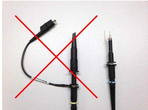
The reference design contains test points (TP) for all the different circuit blocks to simplify the evaluation of the board. To modify the probe, remove the probe tip cover. In addition, the ground lead and alligator clip must be replaced by a ground spring as [Figure 19](#) shows. The modified probes fit directly into the test points (TP). The small ground spring significantly reduces the noise, which can couple otherwise into the long ground lead of a standard probe configuration.
