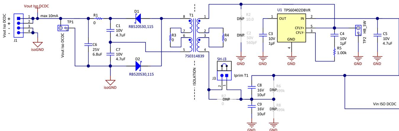
J1: *Vout Iso DCDC* – accurate measurement of the output voltage of the ISO DC/DC and connecting a load (SMU or resistor decade). Influence of measurement cable voltage drop is eliminated by a four-wire connection, supported by the four-pin header J1.
