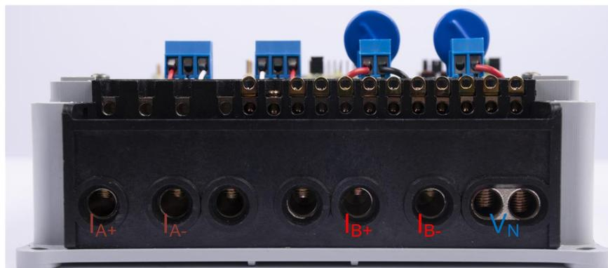
**Figure 3-4. Front View of Reference Design With Test Setup Connections, Two-Voltage Configuration**
