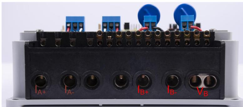
Figure 3-6. Front View of Reference Design With Test Setup Connections, One-Voltage Configuration
