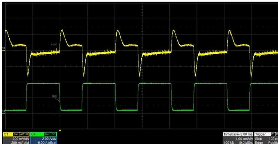
Figure 9 shows the 12-V output voltage (at J11) when the load current pulses between 1.85 A and 3.7 A. The input voltage is 48 V at J1.
