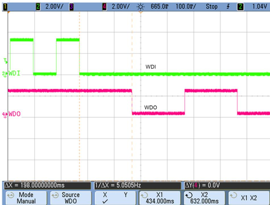
**Configuration 2:** While keeping the CWD pin unconnected, a timeout of 1.6 s is obtained with the watchdog reset delay for 200 ms as Figure 26 shows.
