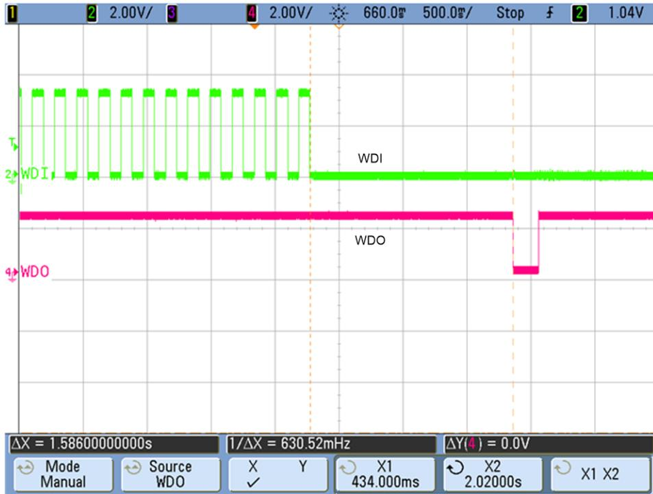
**Configuration 3:** Any other timeout value is achieved by connecting a specific capacitor at the CWD pin. As an example, a 10-nF capacitor is connected and timeout delay of 830 ms is obtained as [Figure 27](#) shows. [Table 2](#) summarizes timing values for all the three configuration of watchdog timer.
