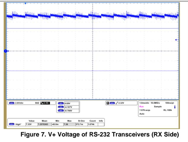
Figure 7. V+ Voltage of RS-232 Transceivers (RX Side)
