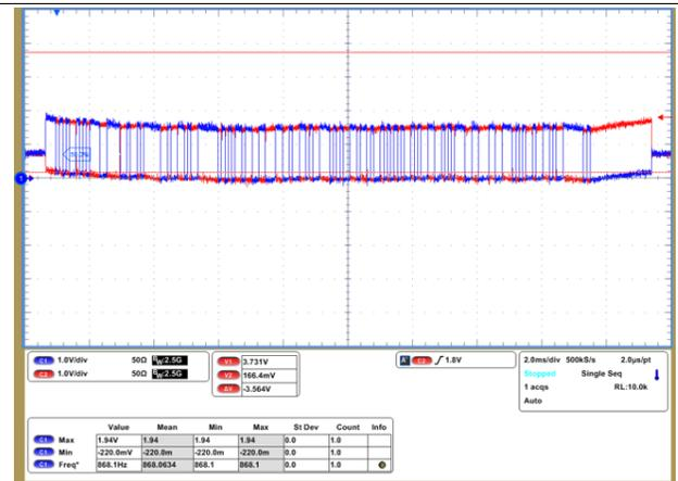
Figure 14. 9600 Baud Rate RS-485 Signal After 800 feet Cable Transmission
