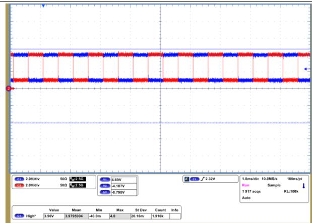
Figure 10. The Converted RS-485 Signal (RX Side)
