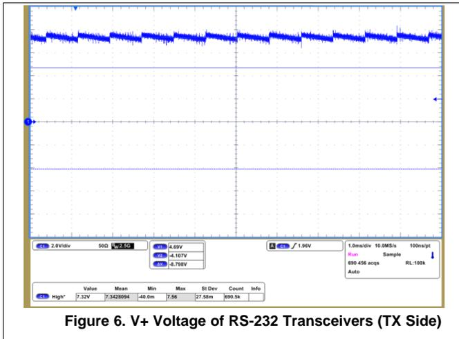
Figure 6. V+ Voltage of RS-232 Transceivers (TX Side)
