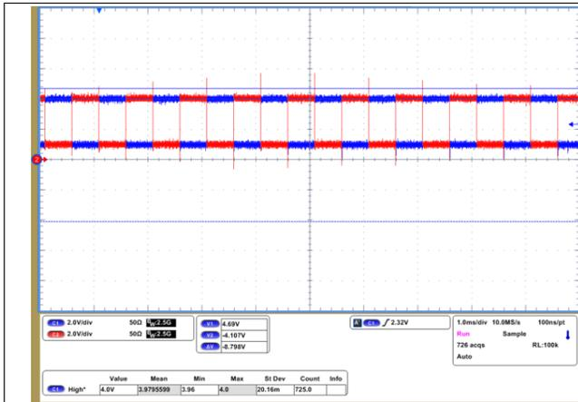
Figure 9. The Converted RS-485 Signal (TX Side)
