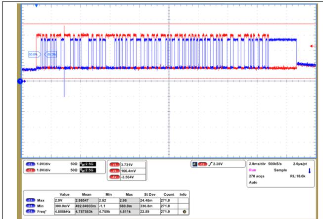
Figure 13. 9600 Baud Rate RS-485 Signal Before 800 feet Cable Transmission
