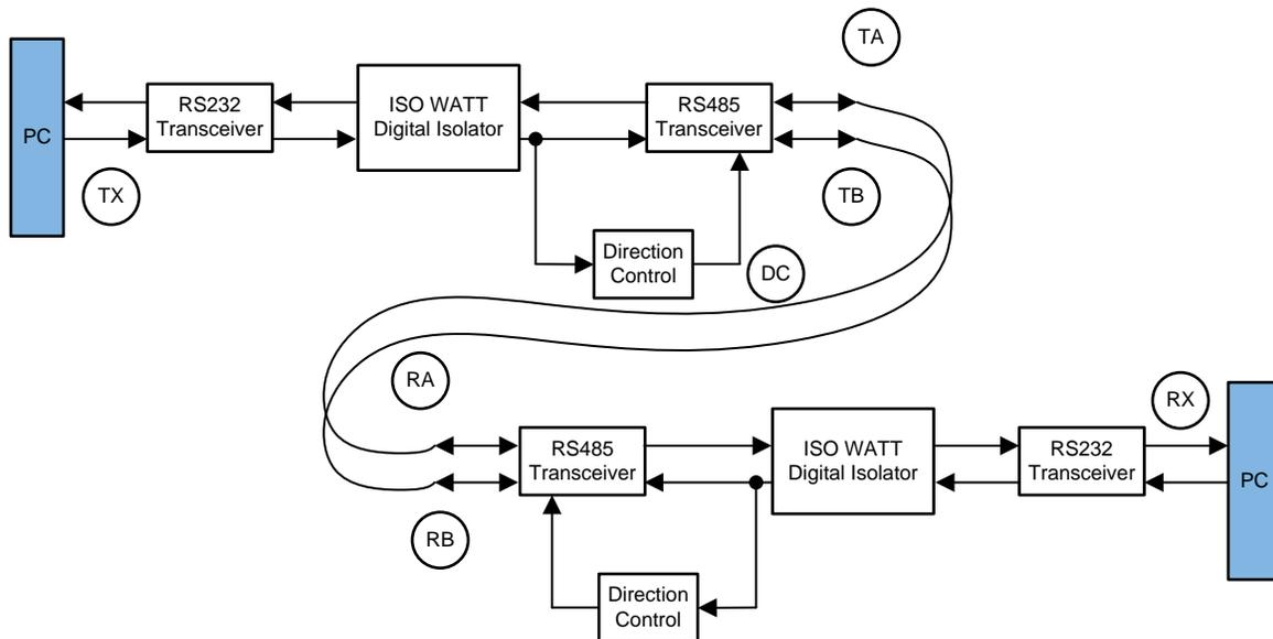
**Figure 4. The Two-way Half-duplex System Setup In Lab**
