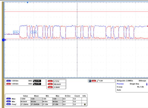
Figure 15. Received 115200 Baud Rate RS-485 Signal after 800 feet Cable Transmission
