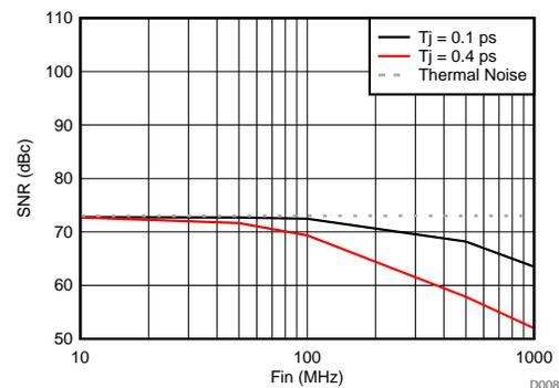
Figure 7 shows the resultant SNR plot due to clock jitter and thermal noise source calculated in Equation 2, SNR degrades due to noise source with increasing input signal frequency.
