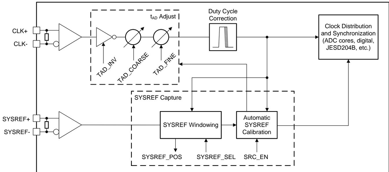
This  $t_{AD}$  feature gives the flexibility to adjust any one or both registers of the ADC to make 90° phase shift between ADCs with 19-fs resolution.
