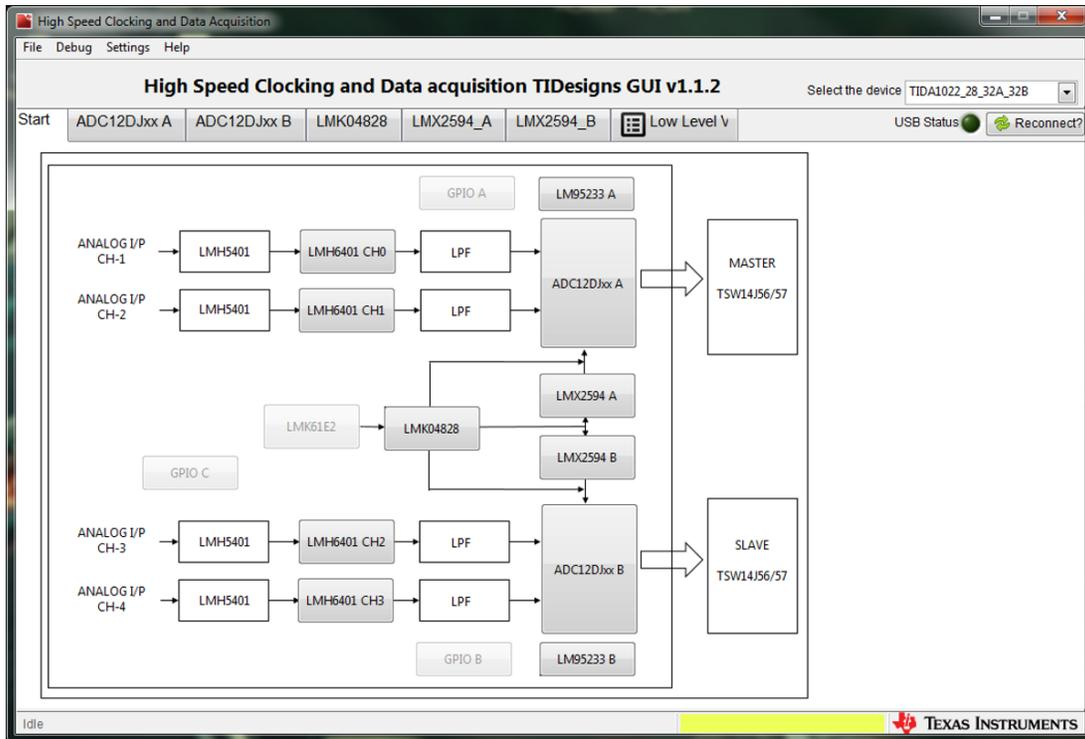
Figure 23. HSDC TID GUI - Low Level Programming View
