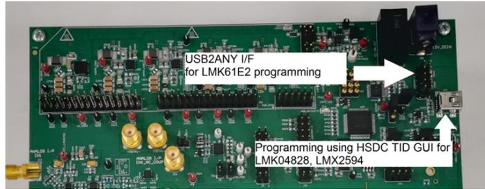
The programming procedure for the built-in programming interface follows:
