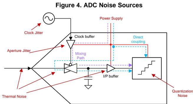
Figure 4. ADC Noise Sources
