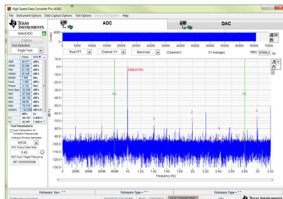
Figure 29 and Figure 30 show the resultant spectrum of 12.8 GSPS with and without IL spur. Figure 29 shows interleave spur at locations  $FS/2$ ,  $FS/4$ ,  $FS/2-FIN$ ,  $FS/4-FIN$ , and  $FS/4+FIN$  associated with sampling clock  $FS = 12.8$  GHz.
