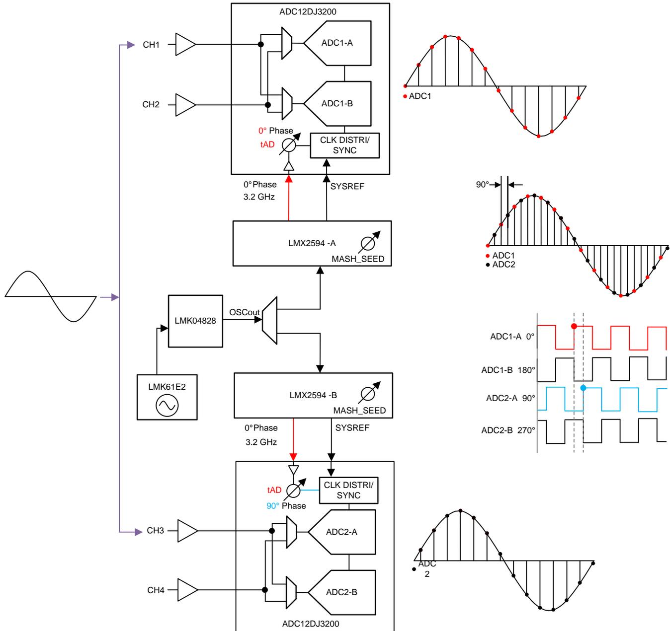
The ADC\_SYSREF, FPGA\_CORECLK, FPGA\_REFCLK, and FPGA\_SYSREF to be calculated based the ADC device clock (ADC\_DEVCLK) requirement and SERDES lanes used for capture.
