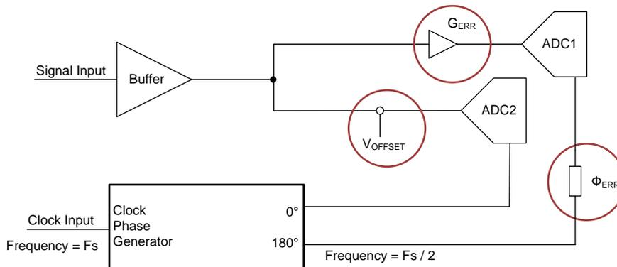
Figure 8 shows a two-ADC interleaved system with typical error sources like offset error, gain error, and time mismatch error between two ADCs which generate predictable spurs in the spectrum of the system.
