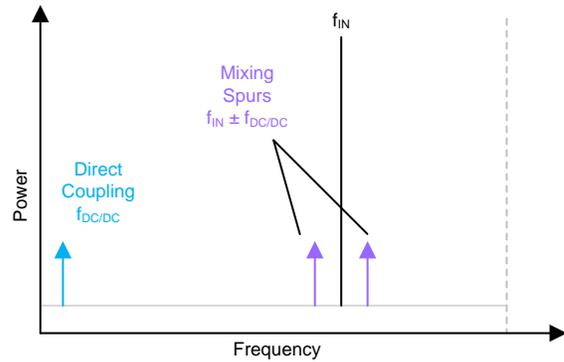
Figure 4, illustrates the typical noise sources degrading converter performance are thermal noise, converter aperture jitter, clocking jitter, and the quantization noise of the converter itself. Furthermore, power supply noise can be directly coupled or mixed with the input signal as Figure 5 shows.
