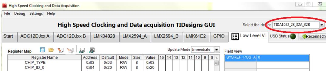
2. Navigate to the *Low Level* tab, select the configuration files to be programmed, and click the *OK* button. Follow these steps as numbered and encircled in the following screen shot:
