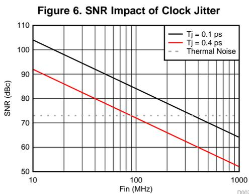
Figure 6. SNR Impact of Clock Jitter
