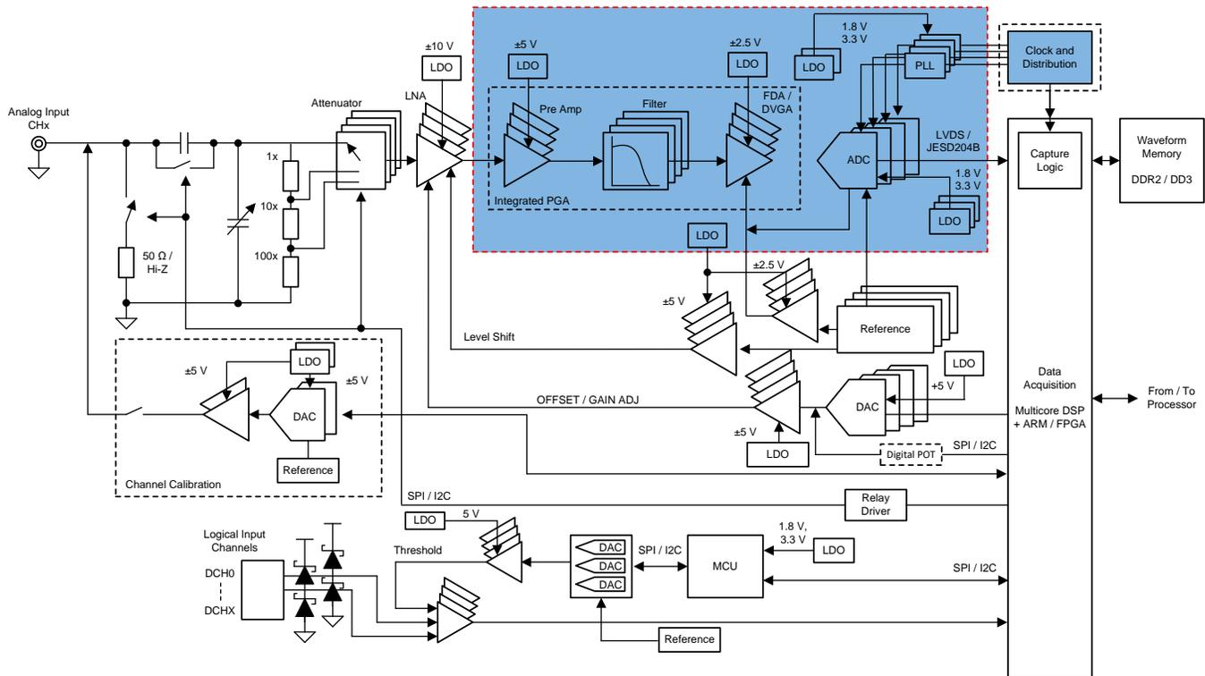
High-performance multichannel digital storage oscilloscopes require a signal chain with a wideband AFE, high dynamic range (SFDR), high SNR, and low channel-to-channel skew. Most high-speed oscilloscopes use 8-bit vertical resolution for waveform visualization but technological development demands new generation scopes at 12- to 16-bit resolutions. The analog bandwidth in the order of the 200-MHz to 5-GHz range requires a sampling rate from 5 to hundreds of GSPS.
