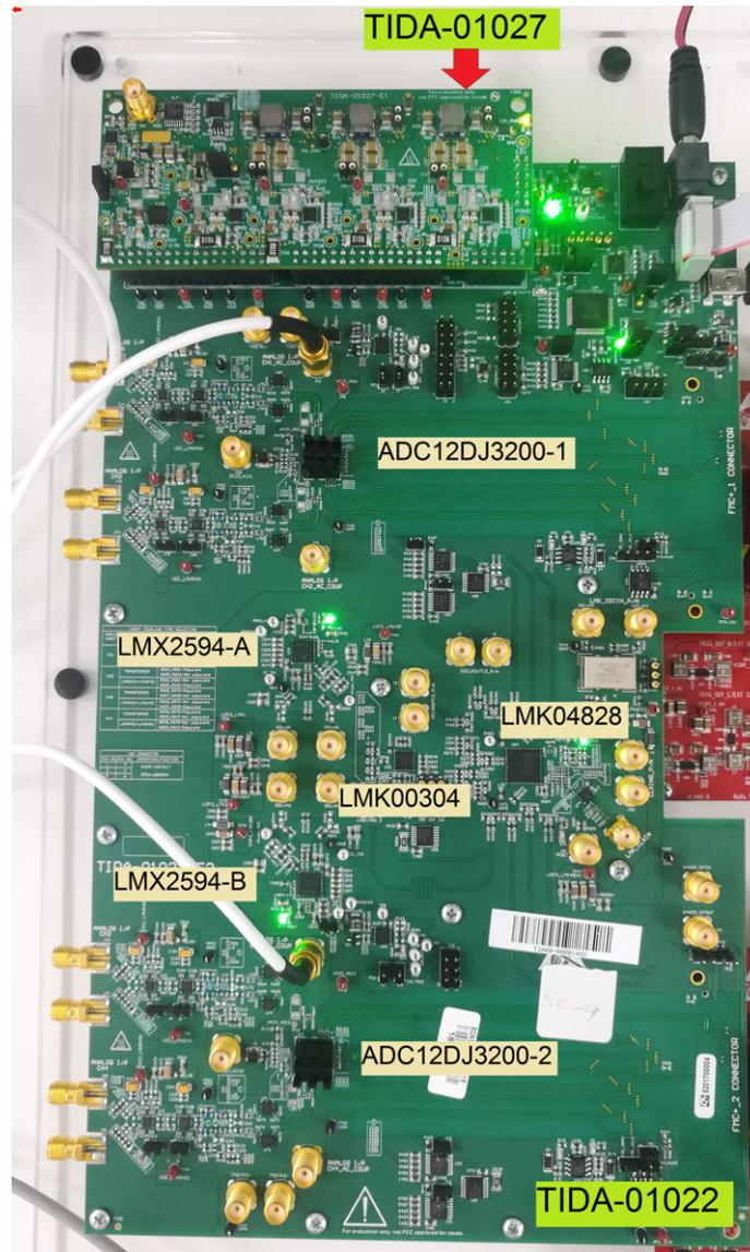
Figure 21 shows the TIDA-01027 board image, in this reference design the TIDA-01027 board is configured as DC/DC free running mode (default mode). The TIDA-01027 output connectors are made compatible with the TIDA-01022 power input headers J58, J59, J60, and J63.
