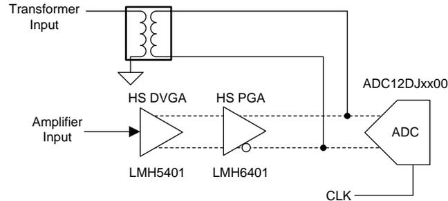
The transformer inputs are designed with Marki™ Microwave Balun BAL-0006SMG parts, which support an input signal of 500 kHz to 6 GHz. The amplifier input path supports frequencies from DC to approximately 1.5 GHz. Detailed circuit information is found in [Flexible 3.2-GSPS Multichannel AFE Reference Design DSOs, RADAR, and 5G Wireless Test Systems](#), the TIDA-01022 design guide.
