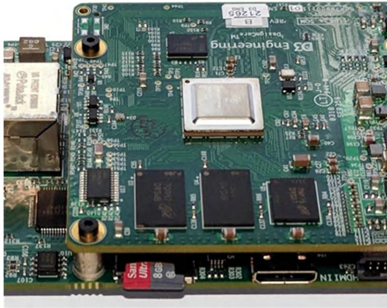
**Figure 3-2. Micro SD Card Inserted Into TDA3x System**
