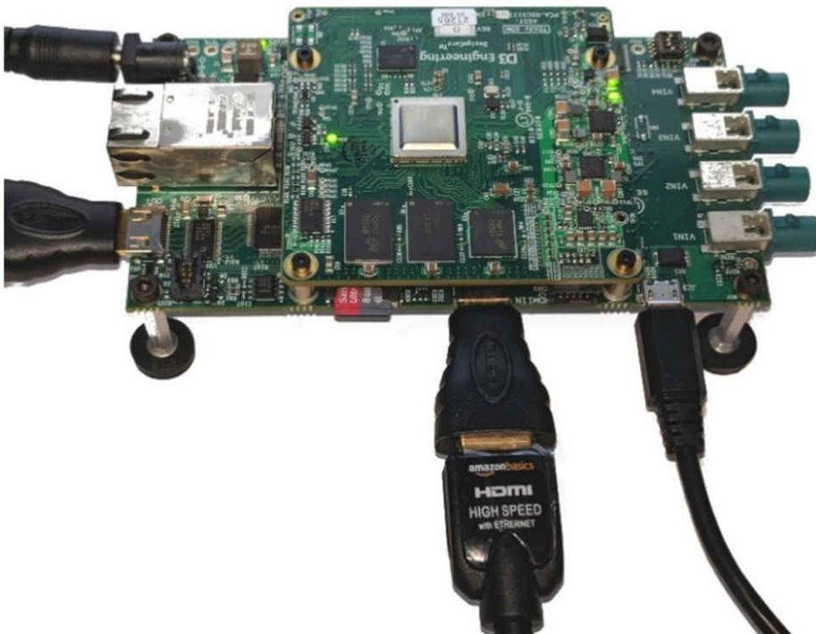
**Figure 3-5. TDA3x System Connected to a Power Supply**
