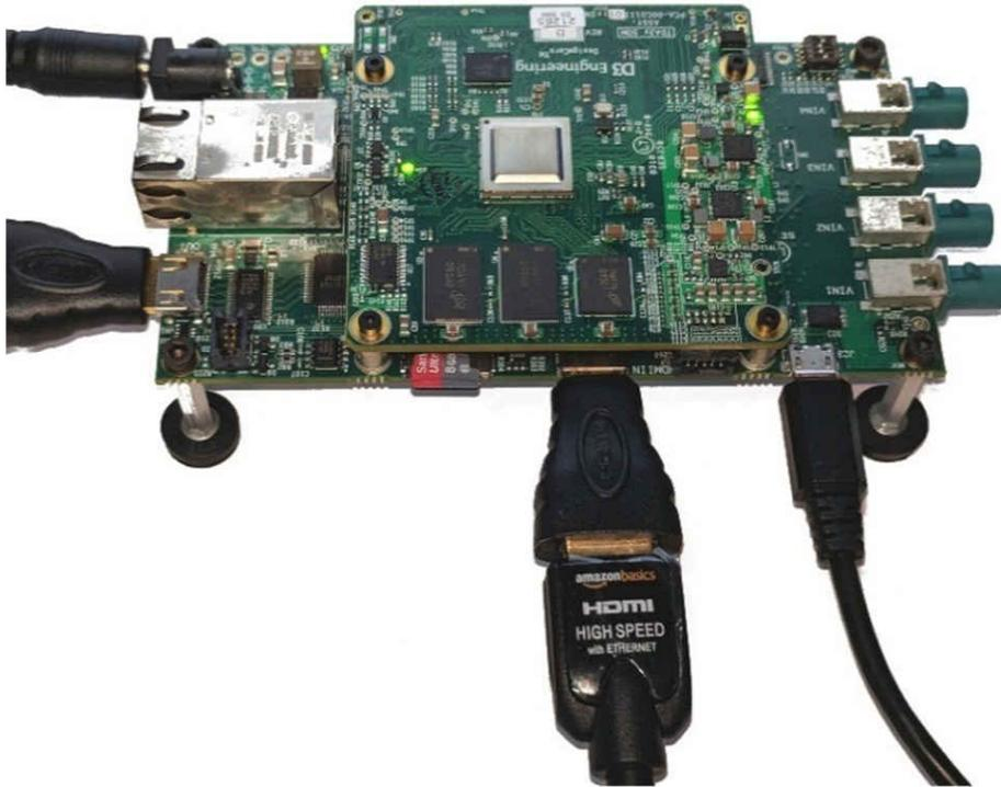
**Figure 3-4. HDMI Mini Connected to the TDA3x System HDMI IN Port**
