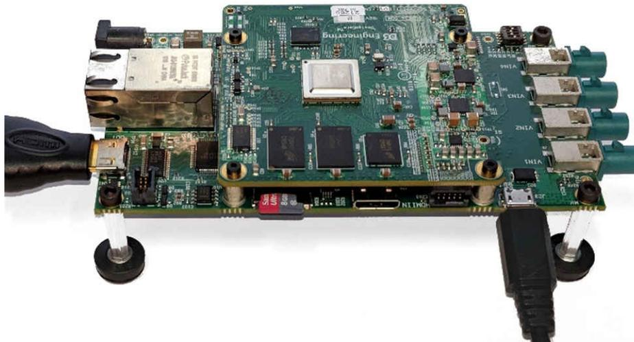
**Figure 3-3. HDMI Mini Connected to the TDA3x System HDMI OUT Port**
