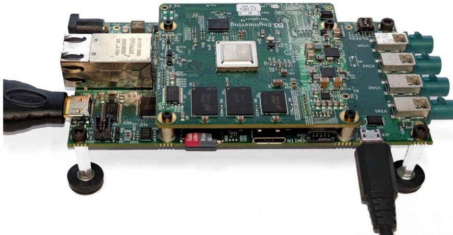
**Figure 3-1. USB Micro B Cable Connected to the Serial Console Debug Port**
