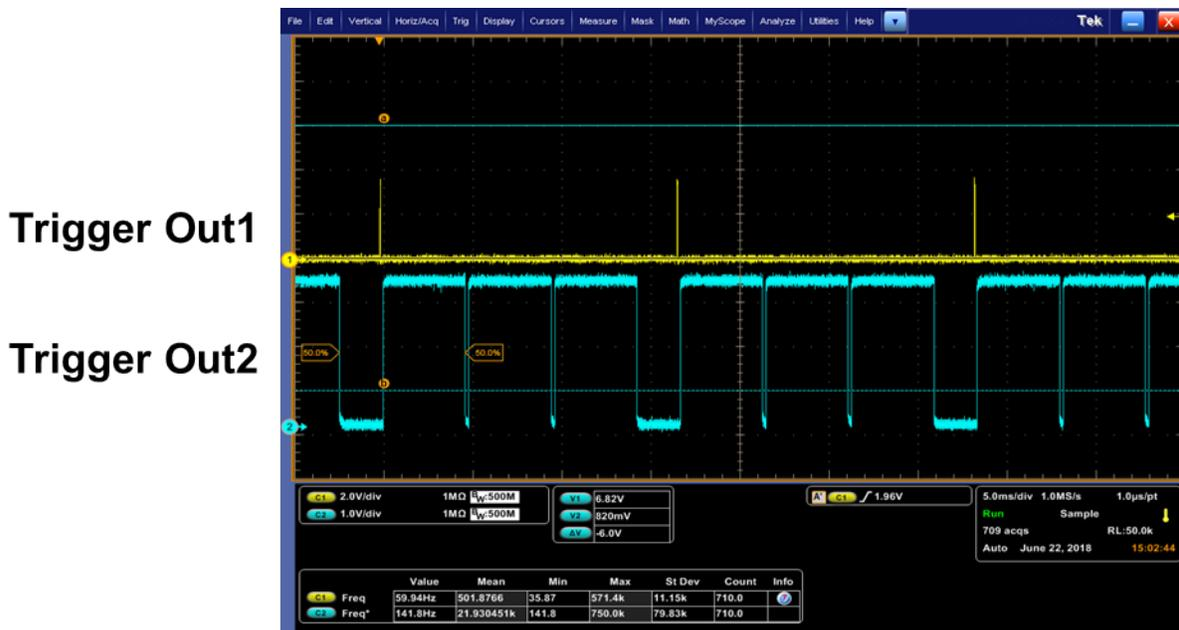
Figure 9. Scope plots of Trigger Out1 and Trigger Out2 (24-bit Monochrome)
