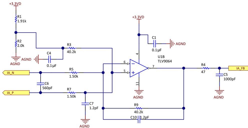
The current sensing circuit is designed as a non-inverting amplifier operating from unipolar single supply. The bidirectional current-sensing capability is achieved by adding a 1.65-V reference voltage level shift to the current sense amplifier output. The level shift of 1.65-V bias enables the positive current sensed at op-amp output is above 1.65-V and negative current sensed at op-amp output is below 1.65 V.
