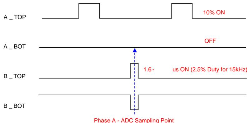
During the testing the ADC of the MCU samples the current sense amplifier output at the middle of phase A high side off period, which is falling near the IGBT switching of phase B, meaning the noise generated during the IGBT switching will couple to the current sense amplifier circuit. The radiated noise emission signal is captured by a floating probe close to the input path of the current sense amplifier, which [Figure 38](#) shows.
