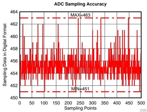
**Figure 41. ADC Sampling Points Distribution**
