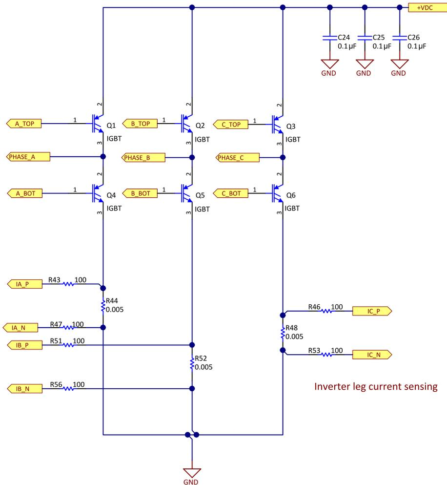
**Figure 8. DC Bus Capacitor Placed in Reference Design Board**
