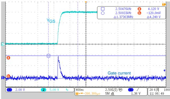
Figure 22. Sink Current From Gate Driver
