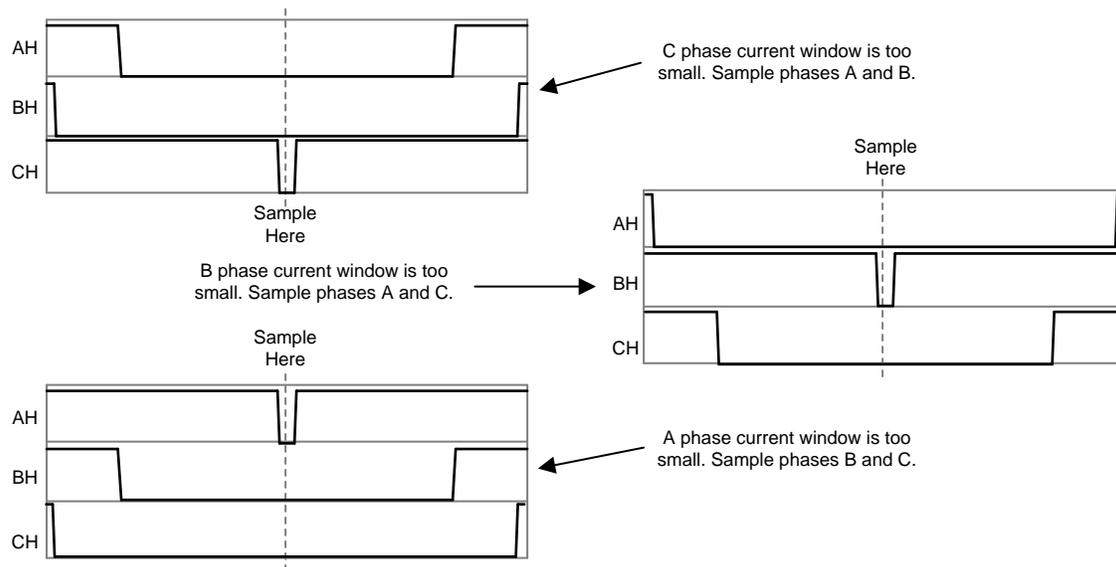
The two-shunt current measurement technique uses the principle of Kirchhoff's current law (KCL), which is that the sum of the currents into a single node equals zero. By measuring only two-phase currents, the third is calculated with KCL. [Figure 3](#) shows a circuit for the two-shunt current measurement technique.
