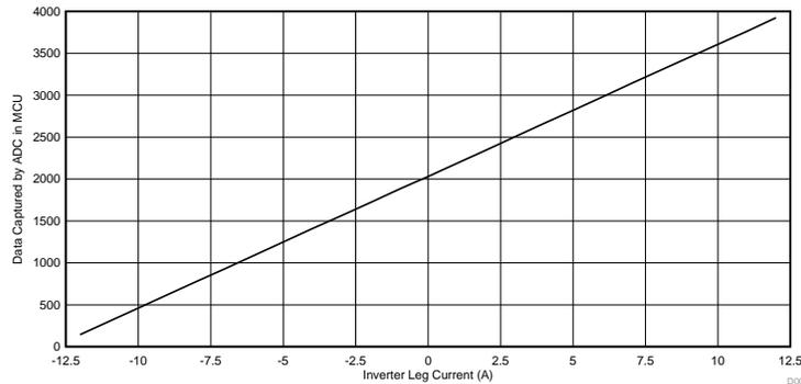
DC accuracy of the current sense amplifier TLV9064 is done with 5-mΩ sense resistor at a gain of 25.125 V/V and at 25°C ambient temperature. The full-scale DC bus current range is -13.2 A to +13.2 A. The inverter leg current is measured with a precision 6½ digit multimeter connected in series to the inverter leg shunt and the output voltage of the current sense amplifier TLV9064 is measured with another precision 6½ digit multimeter.
