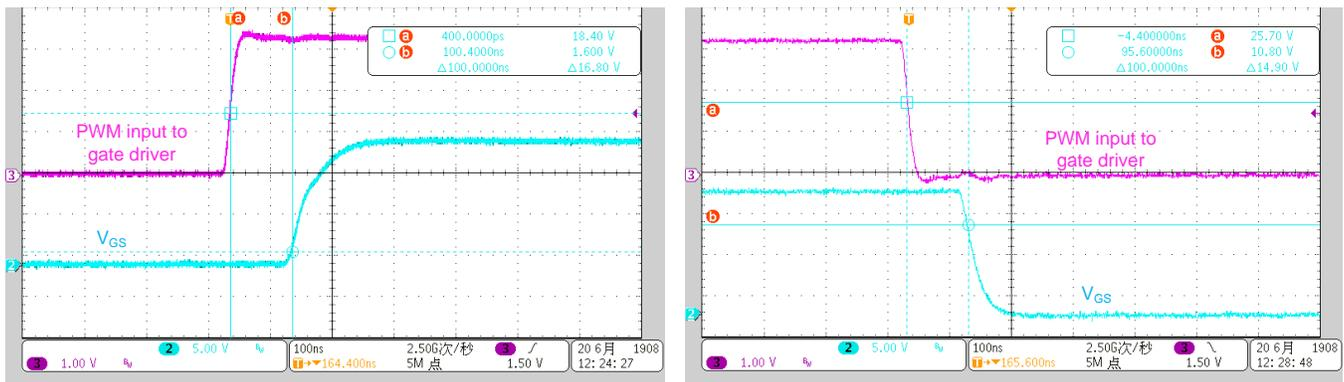
Figure 25 shows the UVLO protection of UCC27712, and the threshold voltage observed is approximately 8.4 V, which ensure that the IGBT is turned on properly with sufficient gate voltage.
