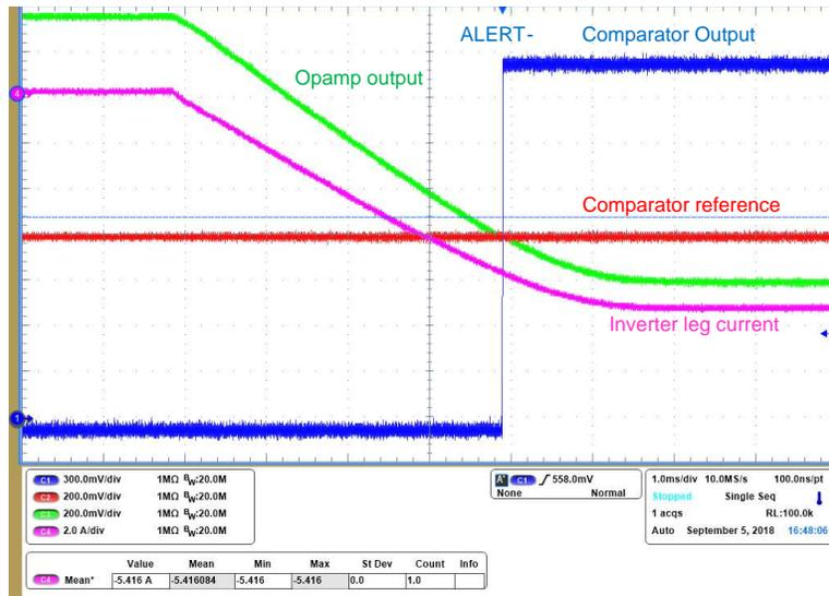
Figure 46. Overcurrent Detection for Negative Current at 2.0 ms/div
