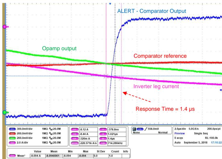
Figure 47 shows the overcurrent protection in hardware, which is achieved by pulling up the active-low enable pin of line driver SN74AHC367. Figure 48 shows the response time from overcurrent detection comparator output to the IGBT gate turn off.
