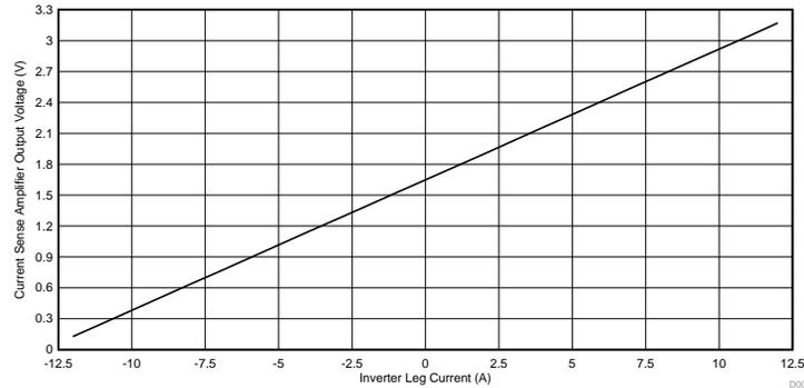
With the purpose of evaluating the transfer function for actual data used in the sensorless FOC algorithm, Figure 33 shows the transfer function of the inverter leg current through the shunt resistor versus the values read from ADC data buffer of TMS320F28027F. The transfer function is linear across -12 A to +12 A current. The transfer function is also linear, which means no extra calibration algorithm needed.
