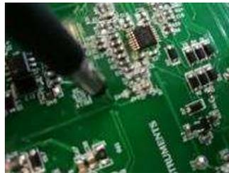
[Figure 39](#) shows the test results of noise effect on current sense amplifier, the floating probe near amplifier input shows DC shift and noise oscillation due to IGBTs switching. Noise is also observed on the amplifier output.
