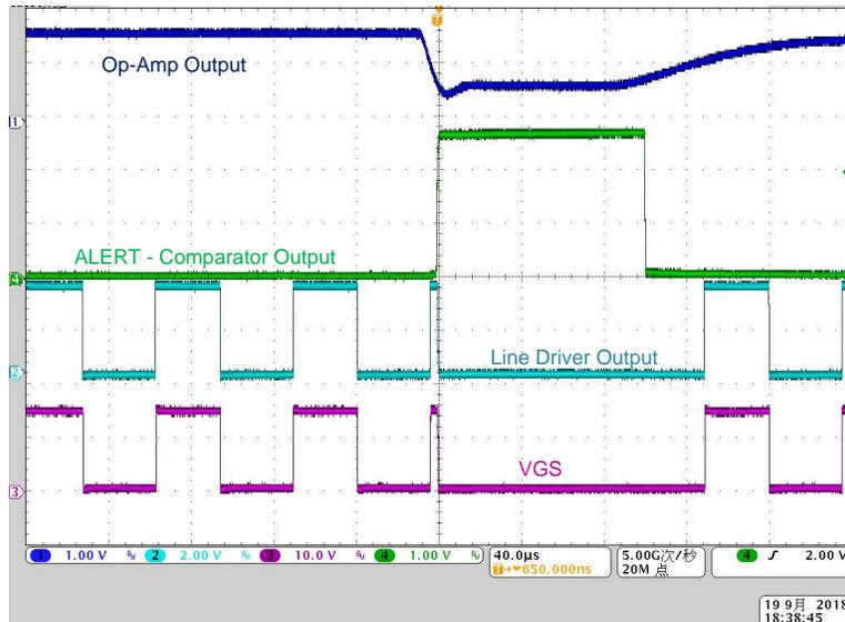
Figure 48. Response Time of Overcurrent Protection in Hardware
