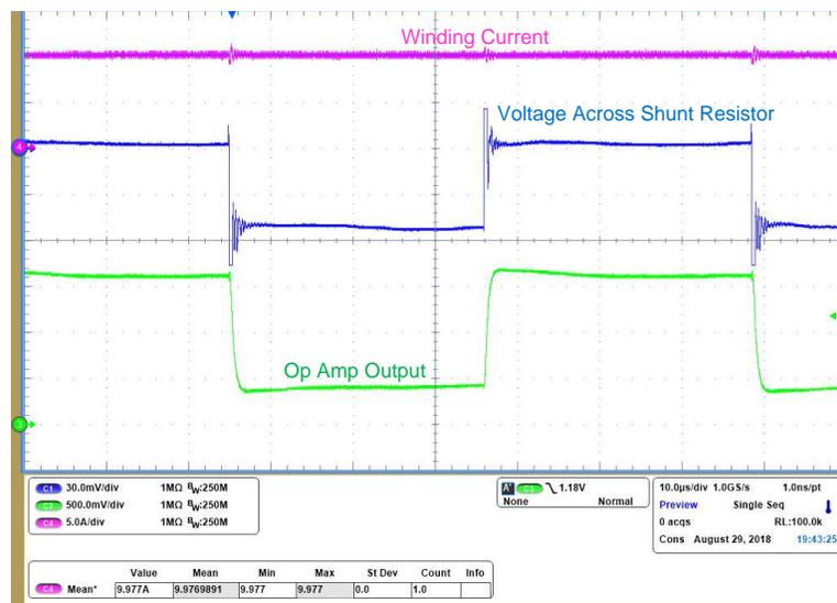
Figure 28. Step Response of Current-Sensing Circuit With 10-A Positive Current
