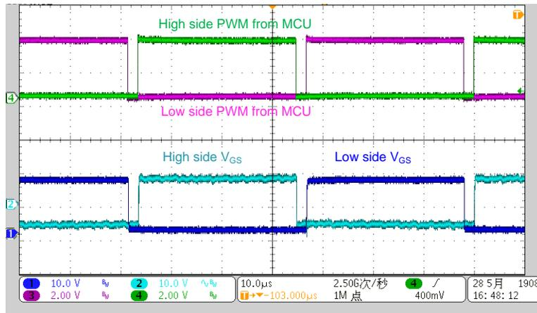
Figure 20 shows the PWM signals of high-side and low-side gate to source voltage from UCC27712, which shows that the dead time configured by the MCU at both of the edges of the PWM. The dead time is programmed to 2  $\mu$ s.
