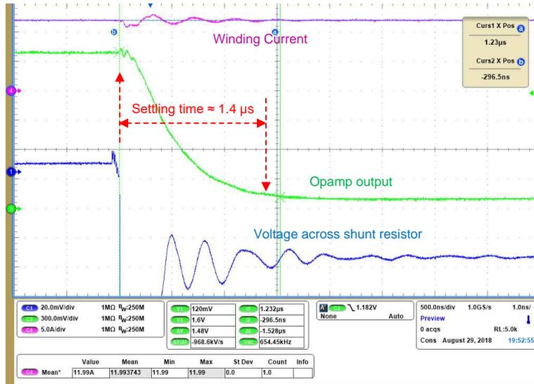
Figure 31. Step Response of Current-Sensing Circuit With 12-A Negative Current
