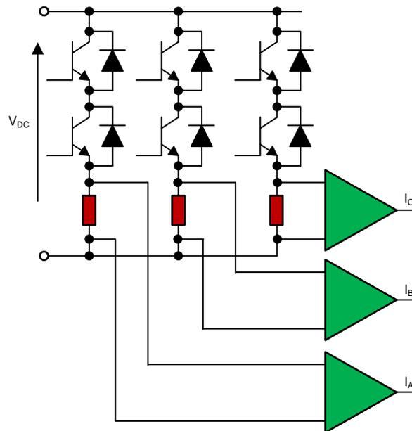
**Figure 2. Using Three-Shunt Current Sampling Technique**
