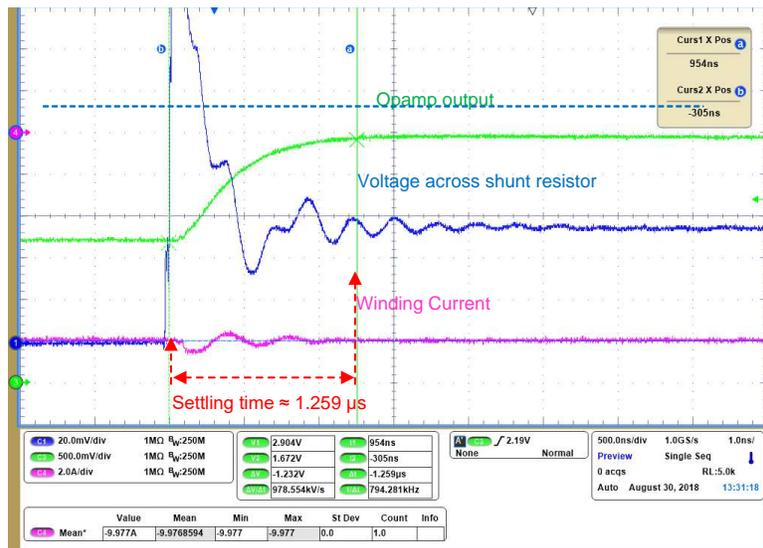
Figure 30 and Figure 31 show the step response with winding current at 12 A winding current. The settling time of current sense amplifier output is 1.34  $\mu$ s. Faster settling time and rail to rail output capability helps to minimize the current sense distortion especially with 2-shunt at lower phase duty cycles.
