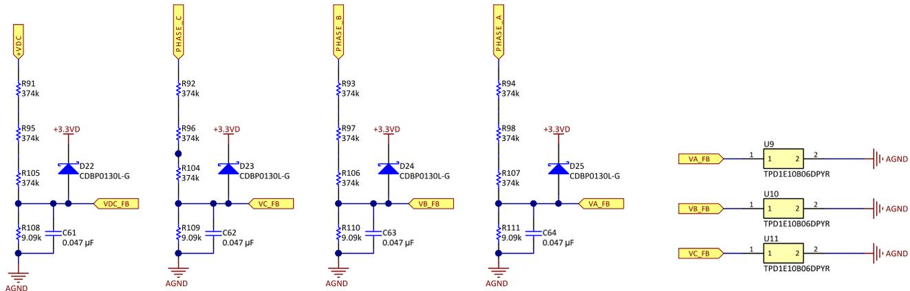
In Figure 13, PHASE\_A, PHASE\_B, and PHASE\_C are the phase voltages. These voltages are properly scaled and fed to the MCU through VA\_FB, VB\_FB, and VC\_FB. The maximum phase voltage feedback measurable by the MCU can be calculated as Equation 16 shows, considering the maximum voltage for the ADC input is 3.3 V.
