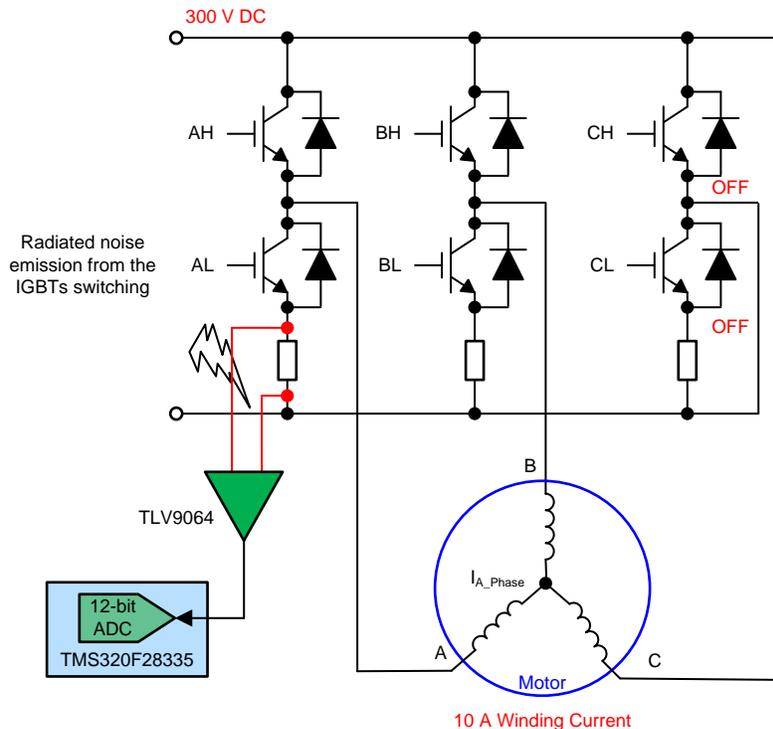
The DC bus voltage is set at 300 V, and the winding current is at 10 A. PWM is applied to Phase A and Phase B. Phase C is left open. Figure 37 shows the PWM signals, the PWM signal driving the high-side IGBT for Phase A has 10% duty, and the low-side IGBT is kept off. The PWM signal driving high-side IGBT for Phase B has 2.5% duty, and the frequency is set at 15 kHz.
