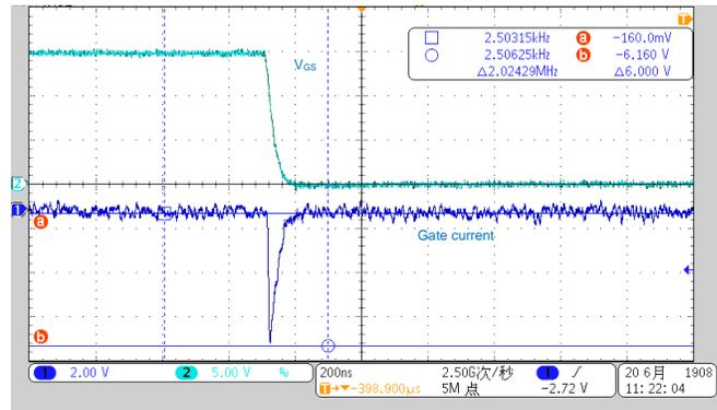
Figure 23. Source and Sink Current From Gate Driver
