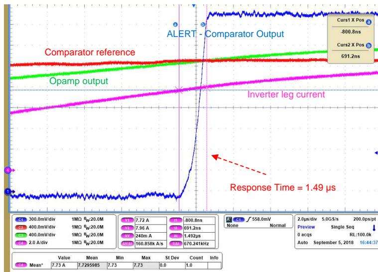
Figure 45 shows the overcurrent detection for negative inverter leg current (positive inverter leg current refers to negative winding current). Figure 46 shows the response time for overcurrent detection and the response time is approximately 1.4  $\mu$ s.
