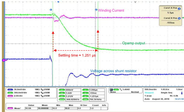
Figure 29. Step Response of Current-Sensing Circuit With 10-A Negative Current
