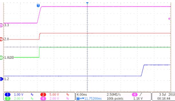
Figure 93. Passive Sequencing 2.8 V, 1.8 V, and 1.2 V
