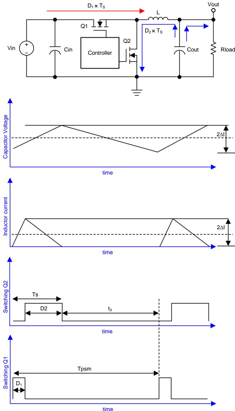
**Figure 3. DCM Mode Operation**
