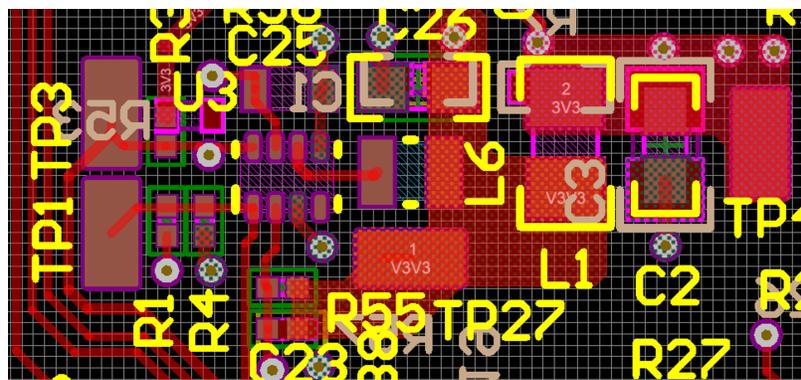
Figure 15. DC/DC Layout Example
