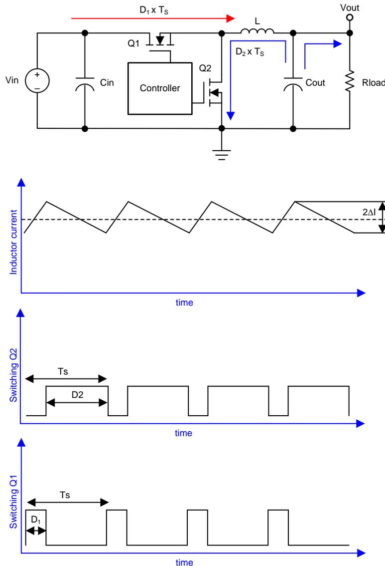
**Figure 2. CCM Mode Operation**
