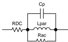
Figure 6. Bead Equivalent Model
