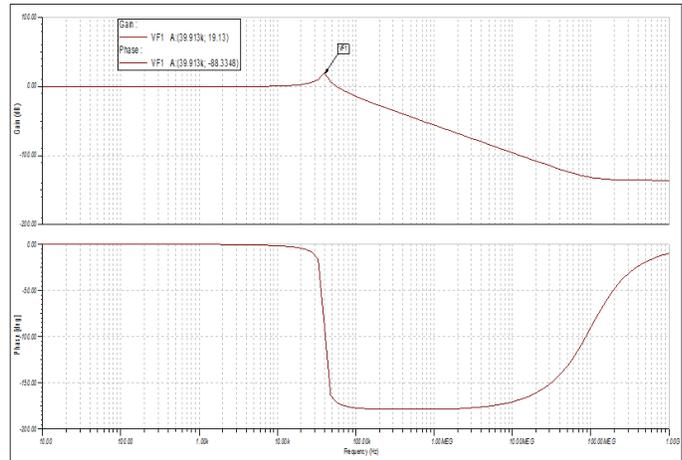
Figure 9. Undamped Filter Response
