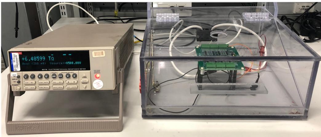
Figure 14.  $R_{IO}$  Test Platform of TIDA-060014
