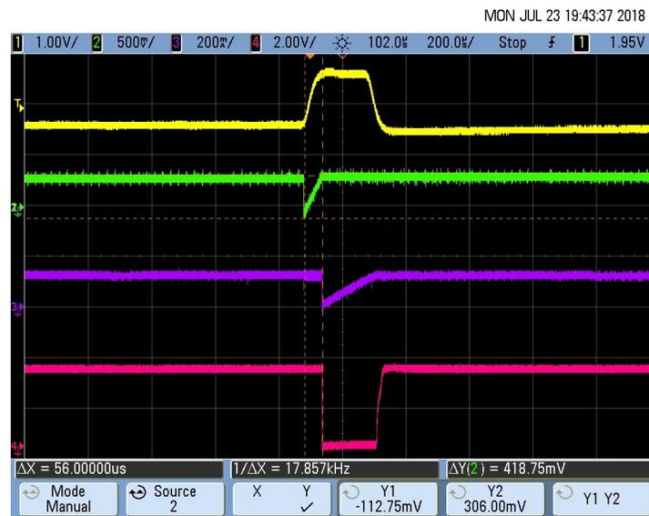
Figure 58. Pacemaker Detection Output (Rise Time  $T_R$ ) for 8-mV, 200- $\mu$ s Pace Pulse
