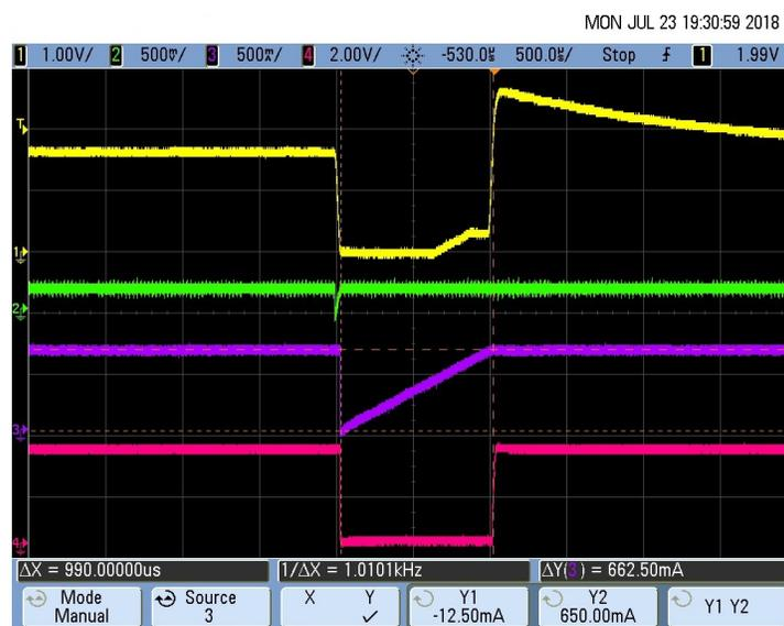
Figure 82. Negative Pace Signal Detection - Negative Pace Pulse Detected by setting the Polarity Check (CH-6) Output of the DAC Low
