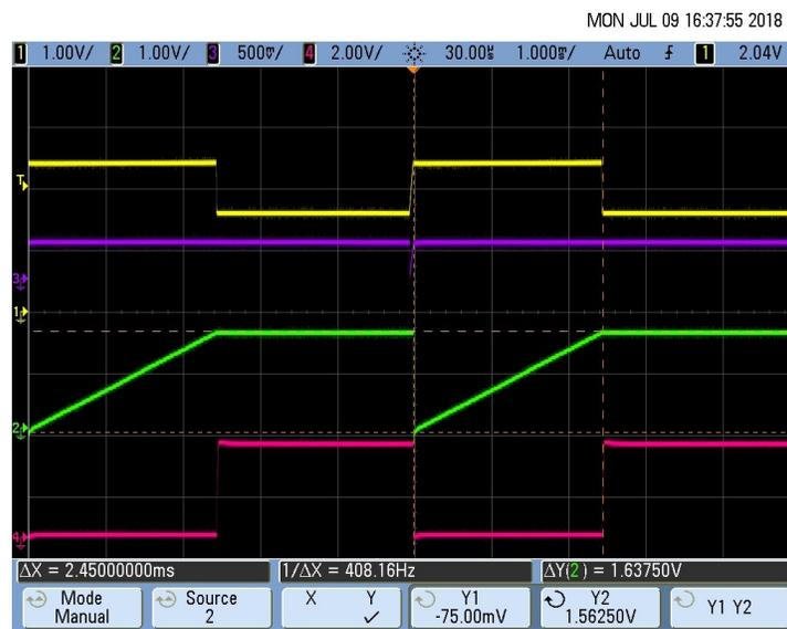
Figure 51. Pulse Duration Measurement of the Pace Pulse ( $T_D = 2.5$  ms)
