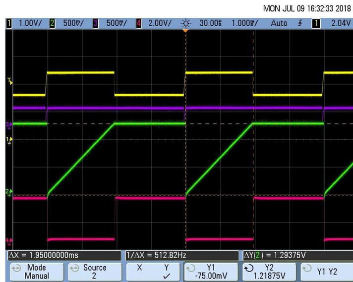
Figure 50. Pulse Duration Measurement of the Pace Pulse ( $T_D = 2$  ms)
