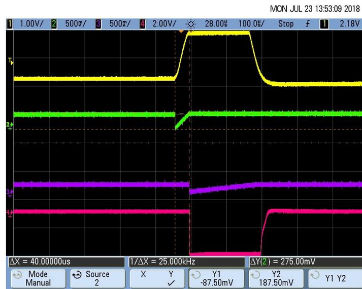
Figure 66. Pacemaker Detection Output (Rise Time  $T_R$ ) for 16-mV, 200- $\mu$ s Pace Pulse
