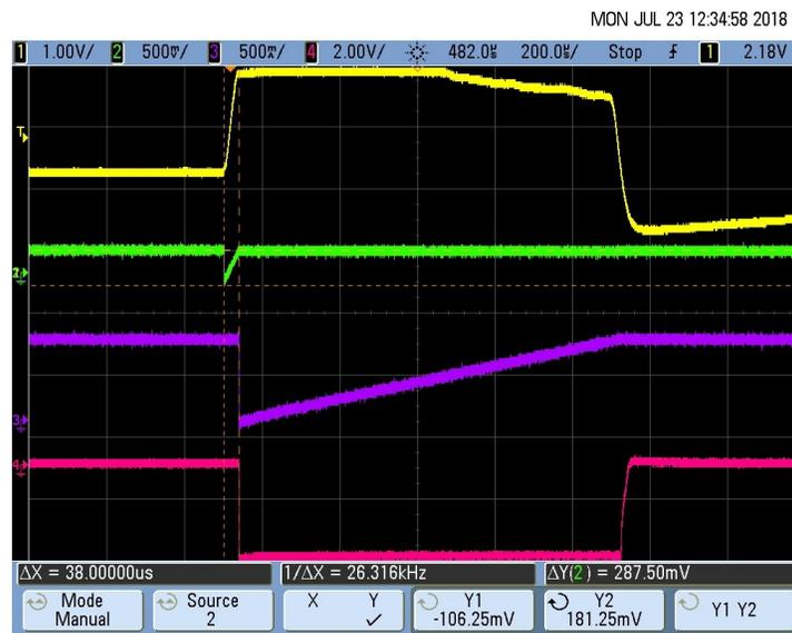
**Figure 70. Pacemaker Detection Output (Rise Time  $T_R$ ) for 16-mV, 1-ms Pace Pulse**
