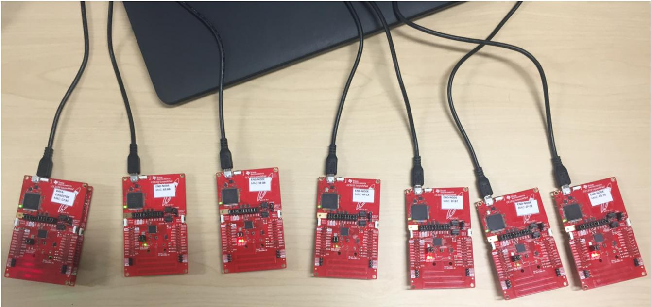
**Figure 16. 6-Hop Linear Topology Setup**
