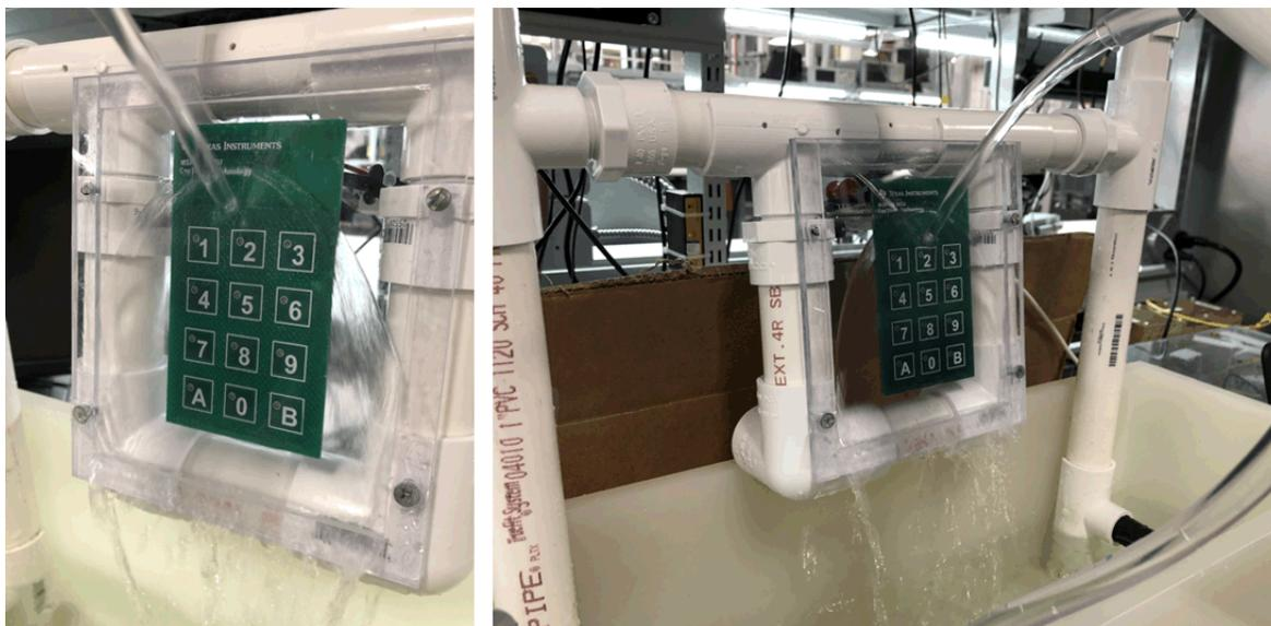
**Figure 17. Continuous Water Flow Test Setup**
