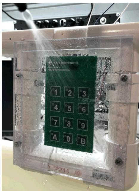
Figure 20. Continuous Water Spray Test Setup
