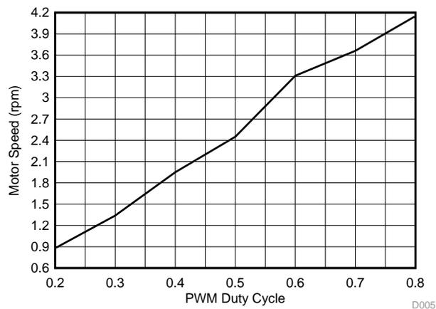
Figure 29. Motor Speed With PWM Duty Cycle
