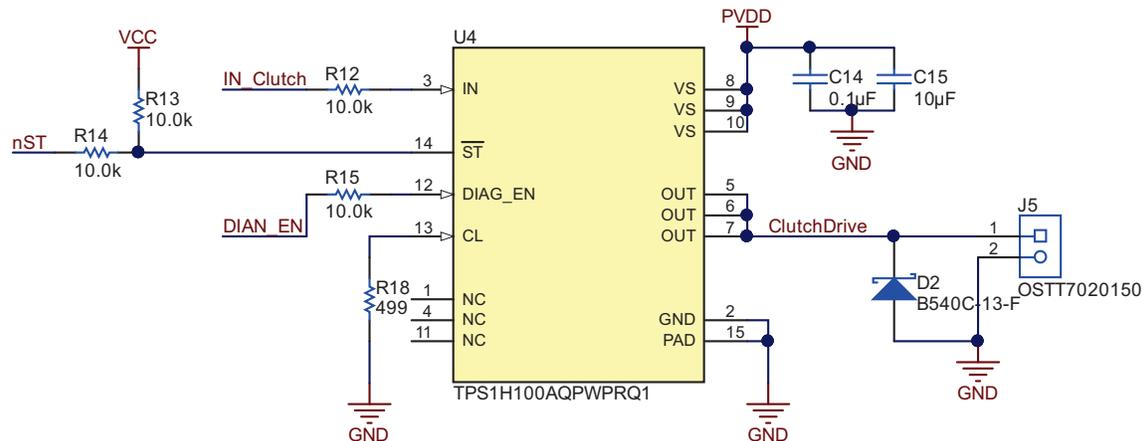
Figure 4. Clutch Drive Circuit
