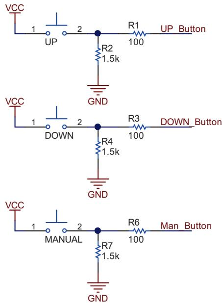
**Figure 9. Push-Button Circuit**
