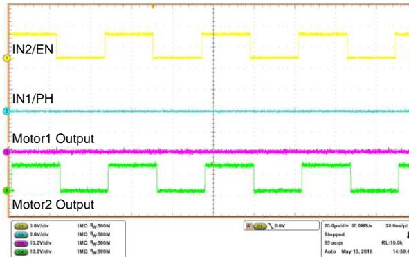
**Figure 19. Reverse Gate drive Signals**
