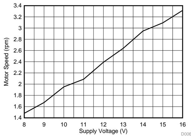
**Figure 30. Motor Speed With Supply Voltage**
