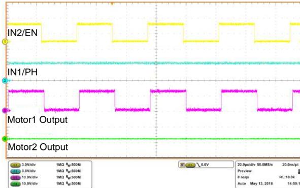
**Figure 18. Forward Gate Drive Signals**
