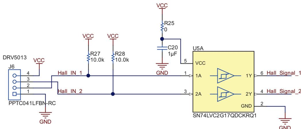
Figure 7. Hall Effect Sensor Circuit
