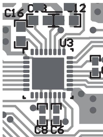
**Figure 39. Bypass Capacitors of AVDD and DVDD**
