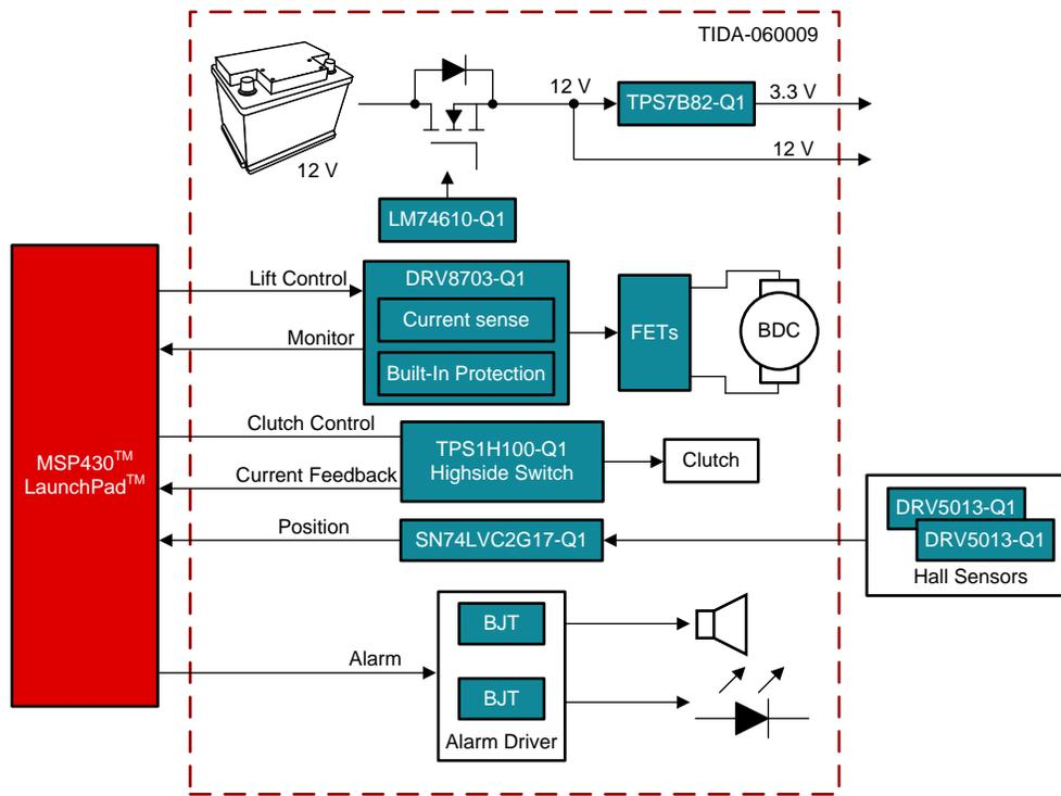
Figure 2. TIDA-060009 Block Diagram
