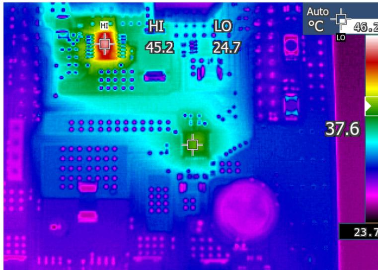
Figure 32. Motor and Clutch Thermal Test
