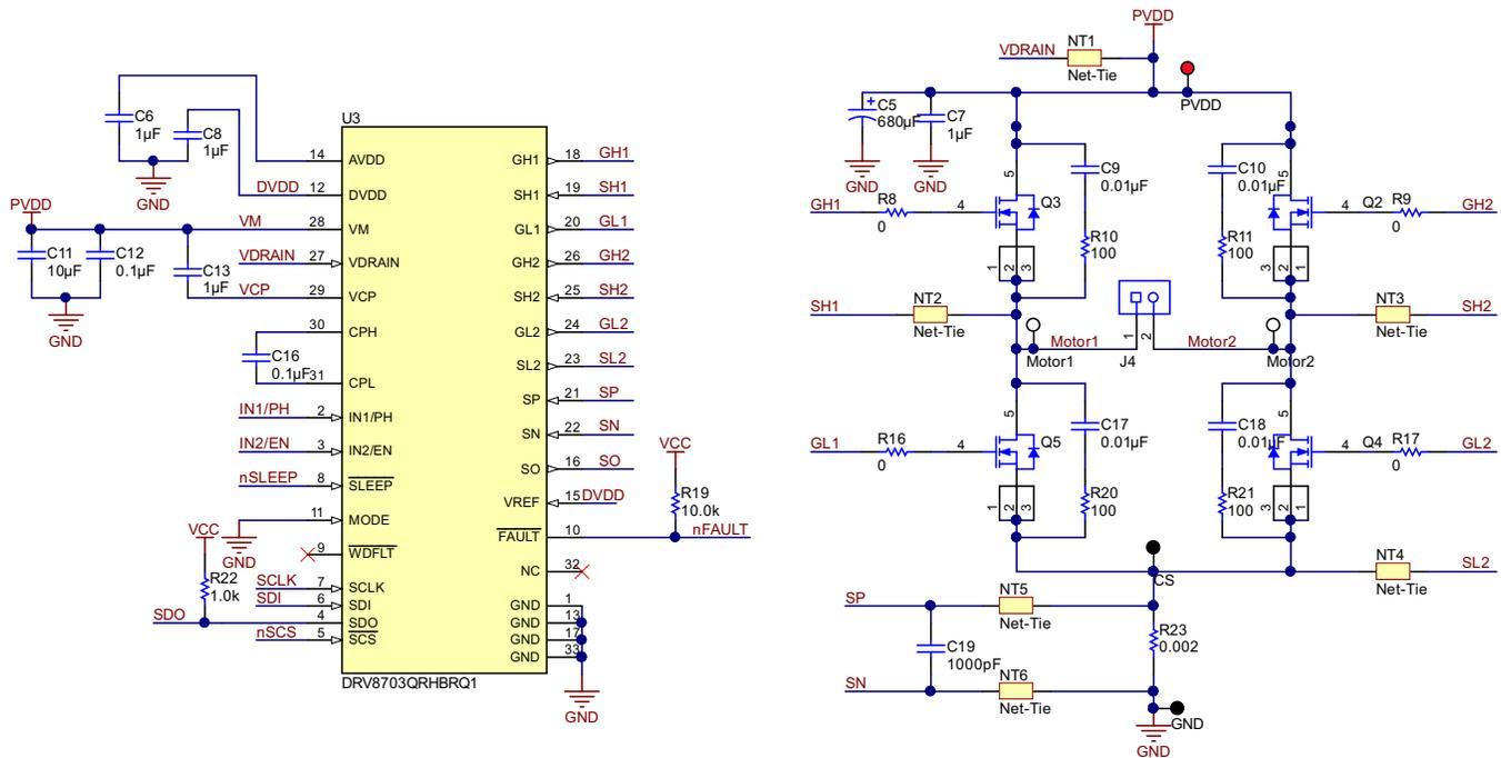
(1) The VM pin on the DRV88703-Q1 device supplies the PVDD voltage.
