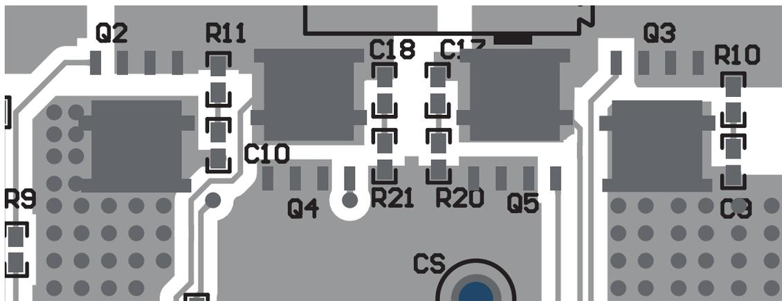
**Figure 38. MOSFET Drain Layout**
