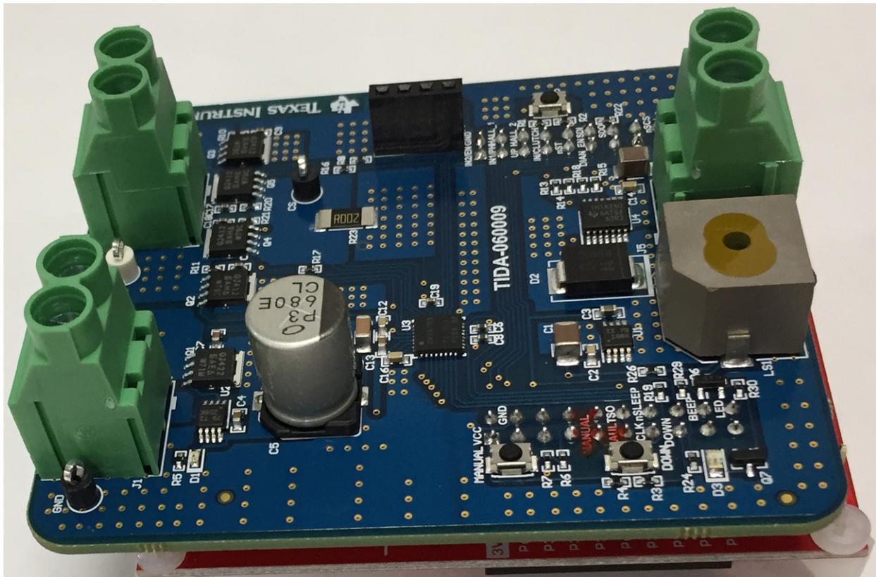
**Figure 11. TIDA-060009 Connection With LaunchPad™ Development Kit**
