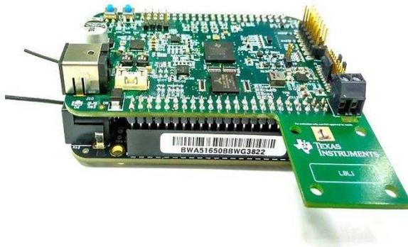
**Figure 26. DSP Board Sitting on top of BeagleBone™ Black Wireless With DC Jacks Aligned**
